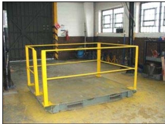
A storage pallet was constructed for Recycling Division to hoist paper into their compactor
