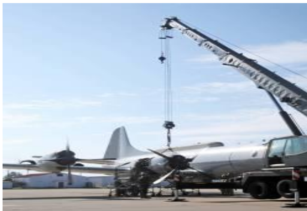
NMCB 74 Crane Crew Lifting EP-3 Turbine
