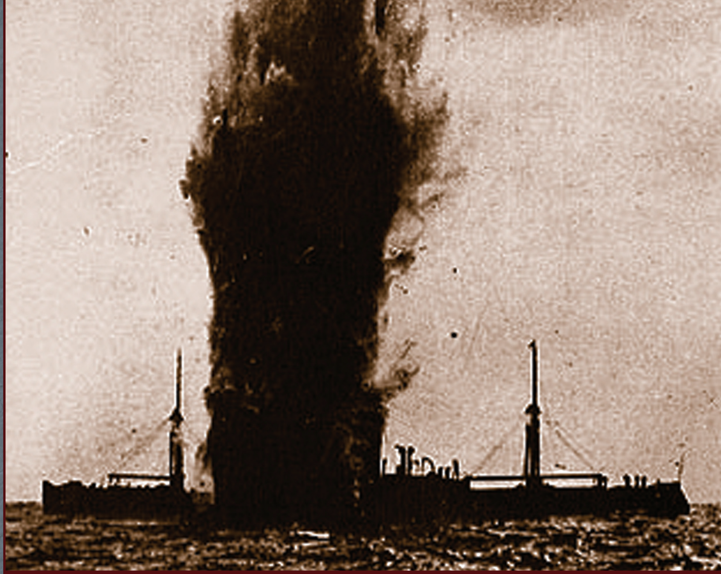
■ A German torpedo explodes against the side of an Allied transport. The Schwarzkopf torpedo had a warhead containing 200 pounds of guncotton explosive, enough to hole any ship.
