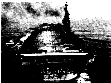
STERN VIEW of the FDR shows increased flight deck space and small island arrangement.
