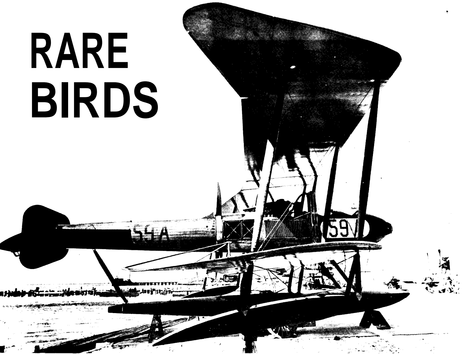
UNIQUE among aircraft which did not go into wartime production was the Gallaudet seaplane. It featured a four-bladed propeller amidships driven by a Duesenberg engine. Above is 59-A at Pensacola in February 1917. Note the anchor design on the rudder, a
