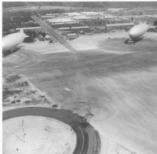
ZP-41 K-ships at Sao Luiz, Brazil. Note the portable stick mast in the foreground.
