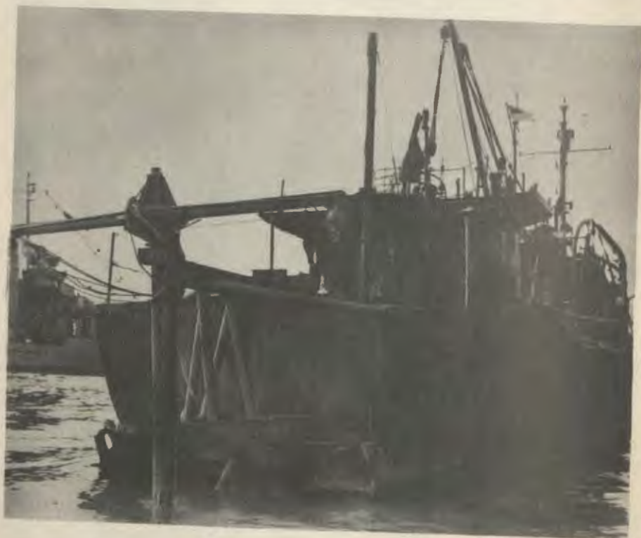
The McFarland's jury rudder made of telephone poles and I beams.
