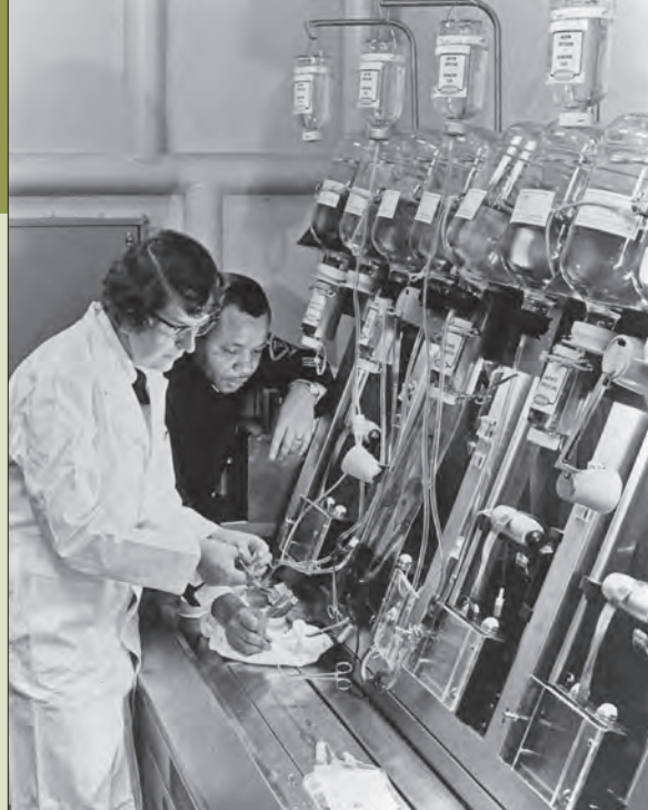
Lieutenant Commander Edna McCormick and Hospital Corpsman Chief H. E. Williams use a cytoglomerator to reconstitute frozen blood aboard Repose (AH 16).
