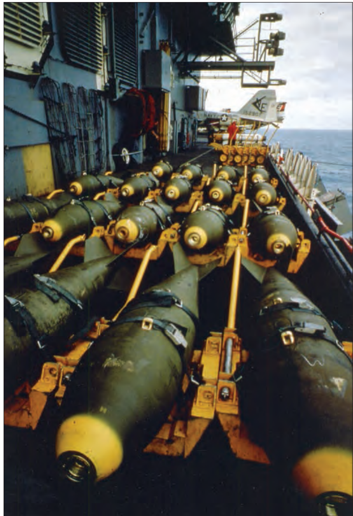
General purpose, or iron, bombs crowd the deck before ordnancemen load them onto Task Force 77 attack planes.
