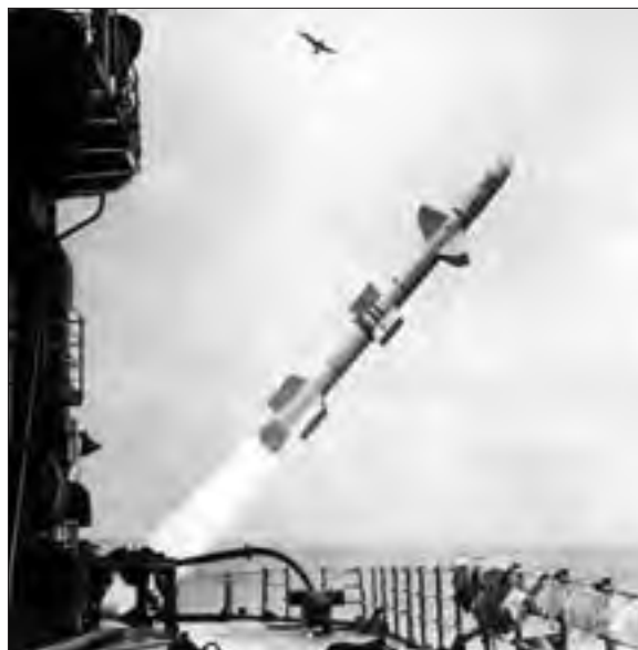
A Talos missile blasts skyward from a Navy cruiser during a test of the weapon’s guidance system in early 1968.
