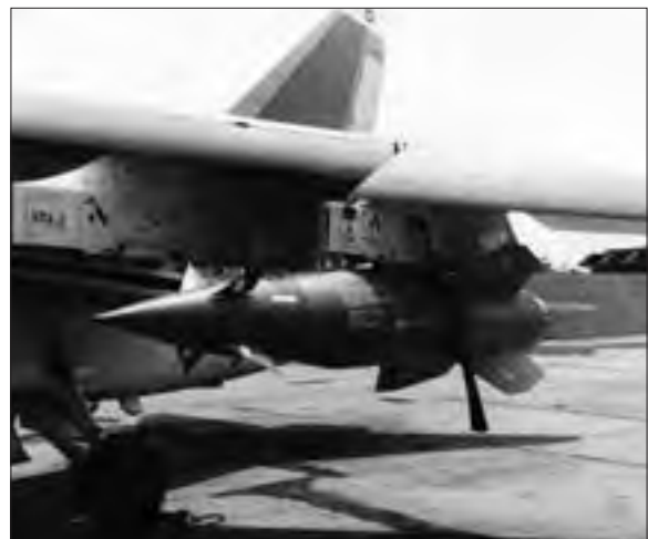
An AGM-12 Bullpup air-to-ground missile affixed to the wing of an A-7 Corsair.
