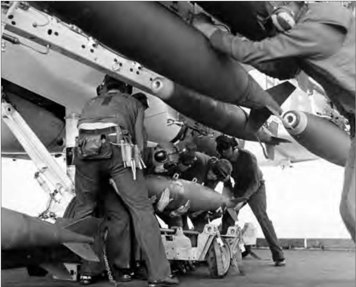
Attack Squadron 85 ordnancemen prepare to lift and attach a 500-pound bomb to a wing station of an A-6A Intruder during the spring of 1968.
