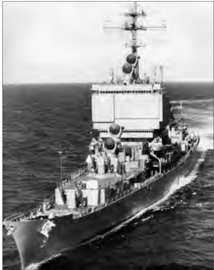
Nuclear-powered guided missile cruiser Long Beach (CGN-9) armed with Talos and Terrier surface-to-air missiles steams through the Western Pacific during the war.
