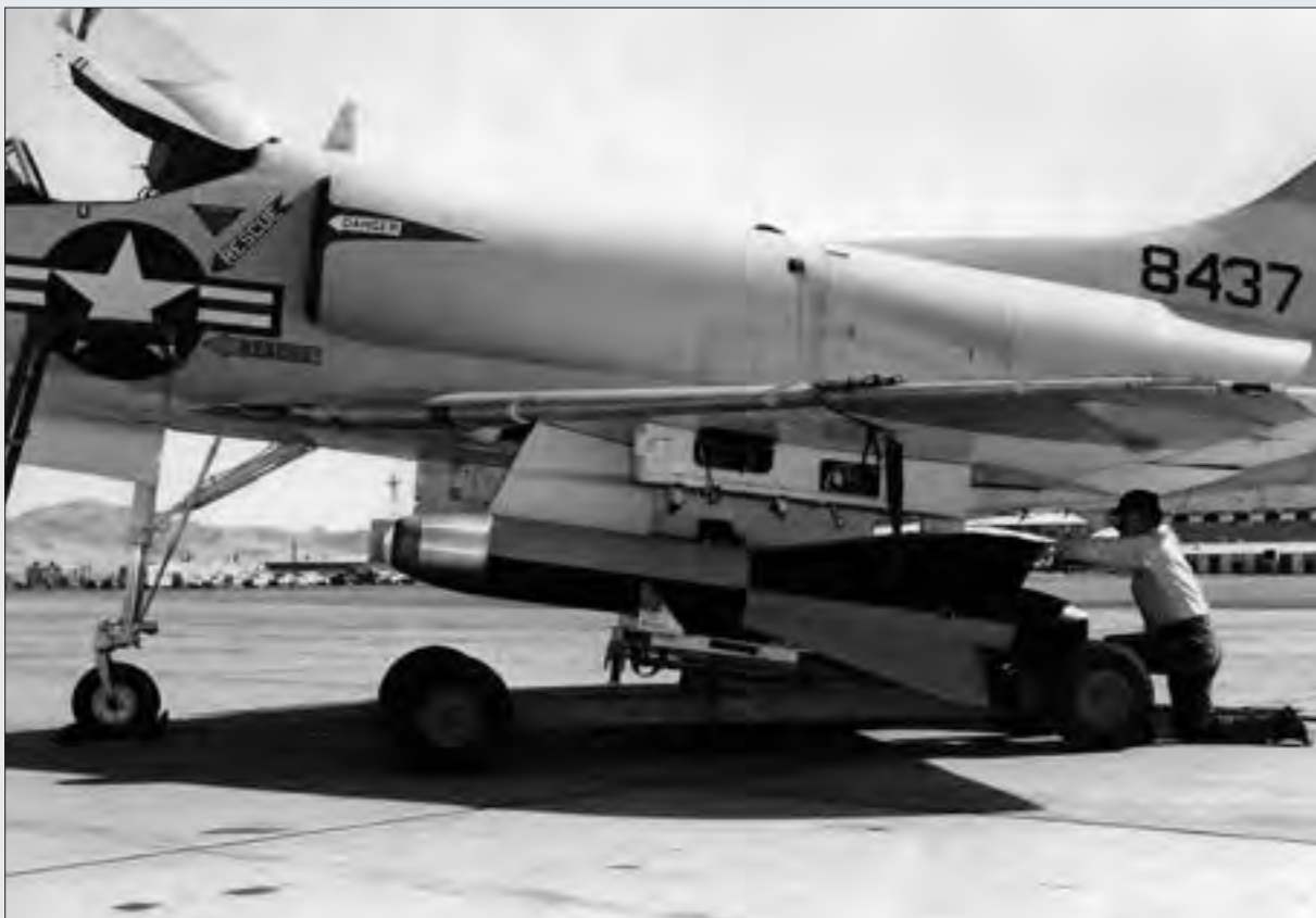
A Navy technician at the China Lake Naval Ordnance Test Station affixes a Walleye TV-guided glide bomb to an A-4 Skyhawk during the weapon's prewar development.
