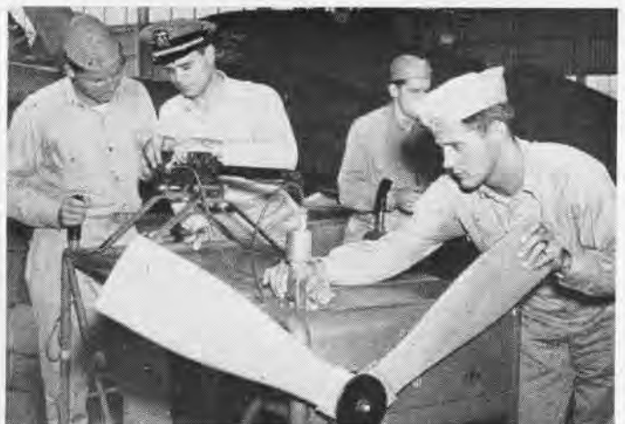
SYNCHRONIZING .30 caliber machine guns to fire through rotating blades of propeller requires utmost precision
