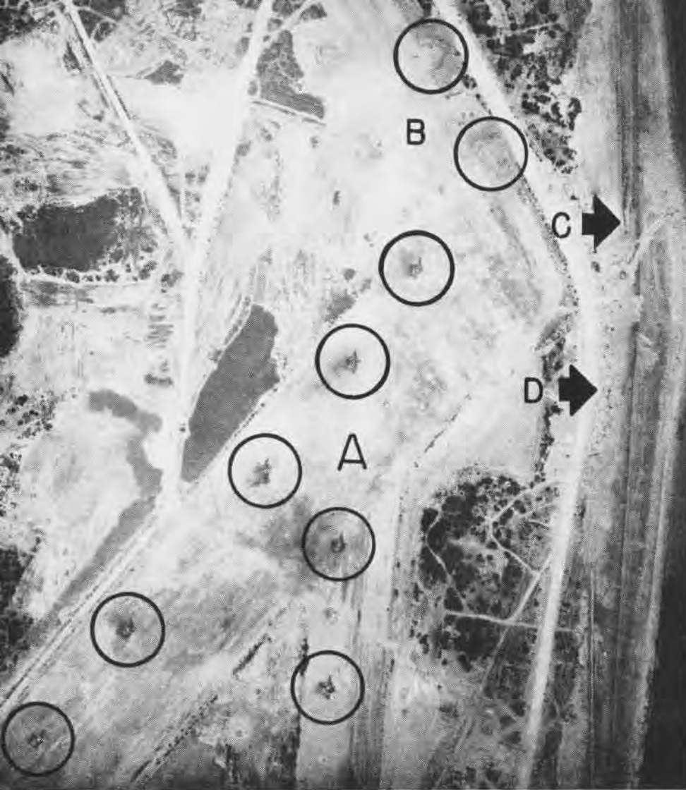
▲ A. JAP BOMBERS DESTROYED BY STRAFING B. REVETMENTS BUILT TO PROTECT PLANES C. TRENCHES AND BARBED WIRE POSITIONS D. TRENCHES AND MACHINE GUN POSITIONS
