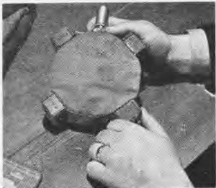
JAP BOMB HELD TO PLANE BELLY BY MAGNETS
