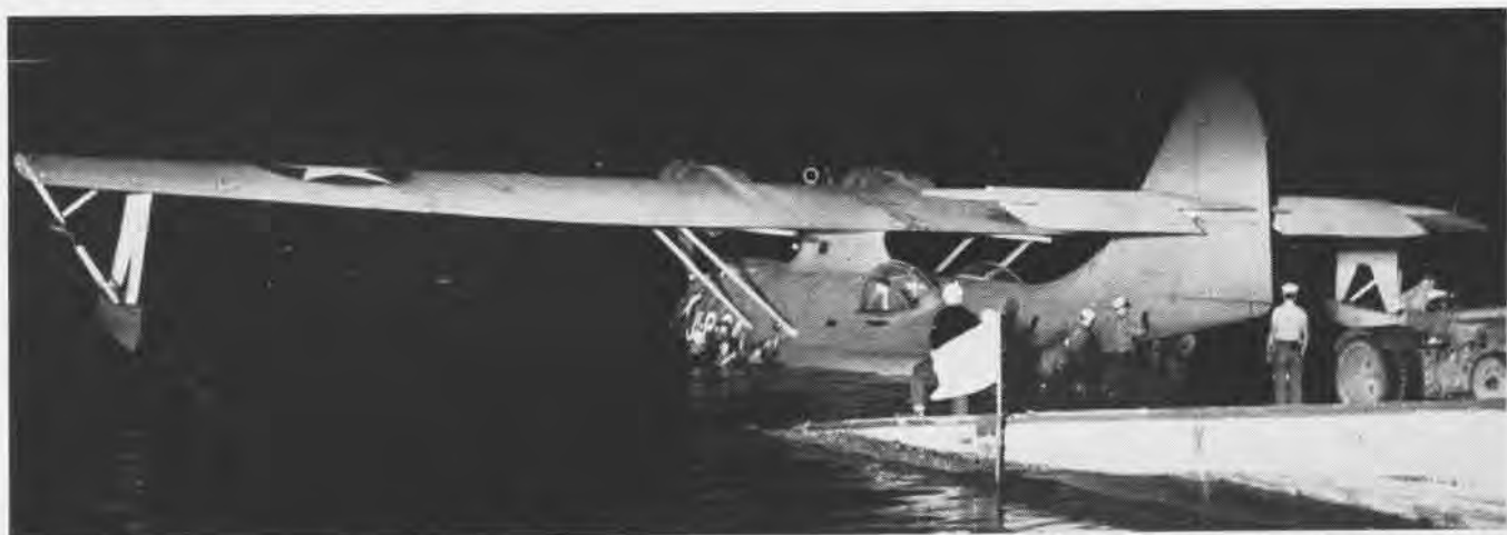
NOT ALL BEACHING OPERATIONS ARE DURING DAYTIME; HERE CREWMEN ATTACH THE CATALINA'S WHEELS SO TRACTORMAN CAN PULL IT FROM WATER
