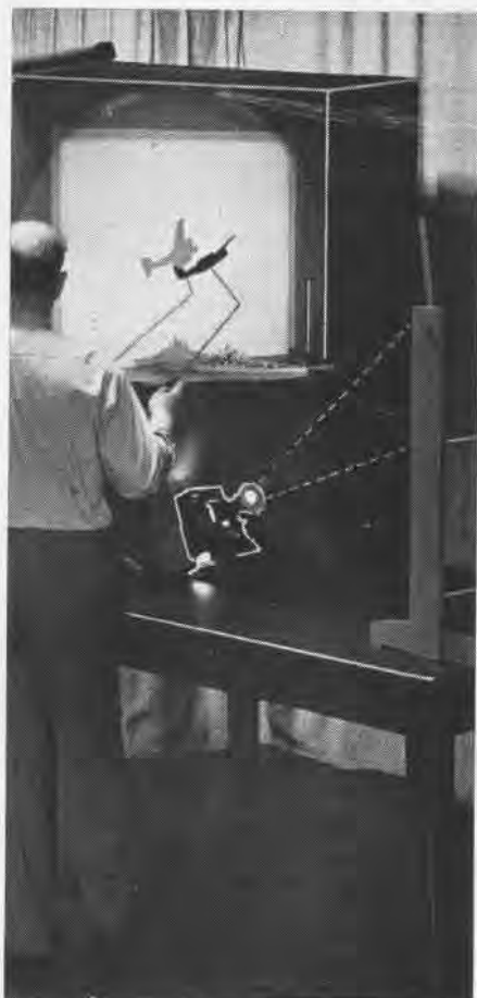
Projectors are used as light sources, but an ordinary light bulb fitted with cardboard shade will produce necessary illumination
