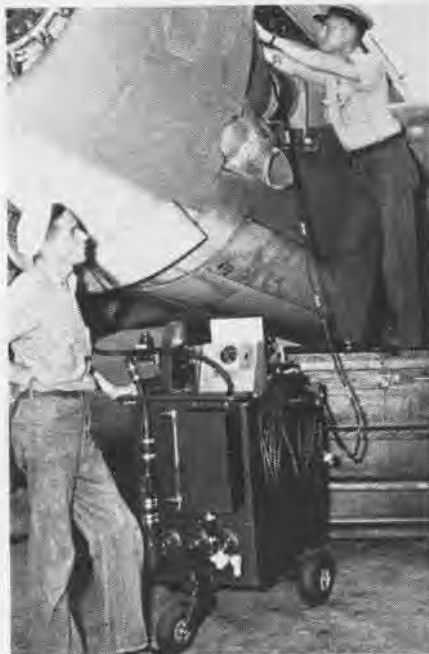
ENGINE PRE-OILING DEVICE BUILT FROM SCRAP
