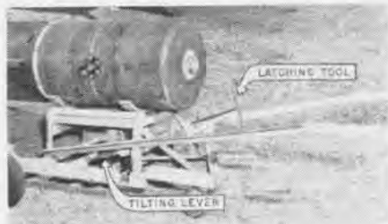
RACK HOISTS BOMBS INTO LOADING POSITION
