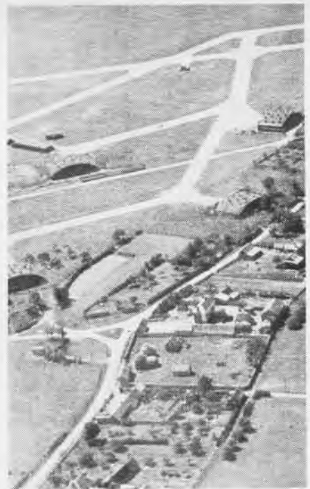
Dummy bushes constructed of netting on framework placed on roofs of hangars make these structures blend into the landscape
