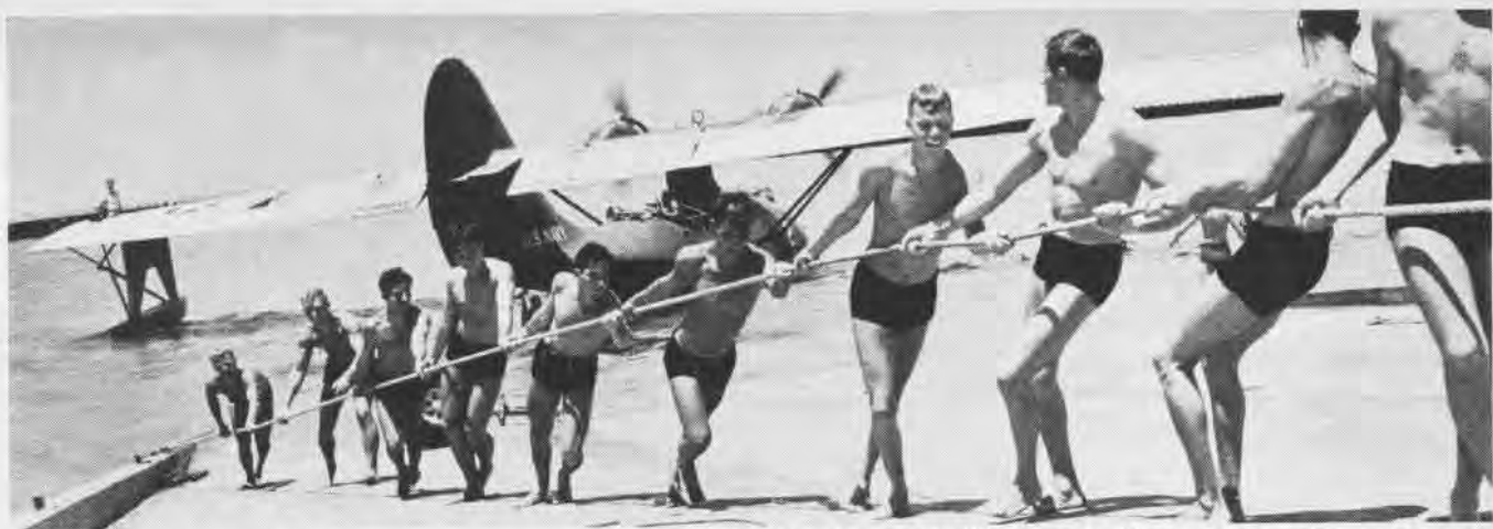
TANNED CREWMEN IN SWIMMING TRUNKS PULL ON LINE TO BRING PBY NEAR RAMP SO THAT BEACHING WHEELS CAN BE ATTACHED AND PLANE HAUL UP
