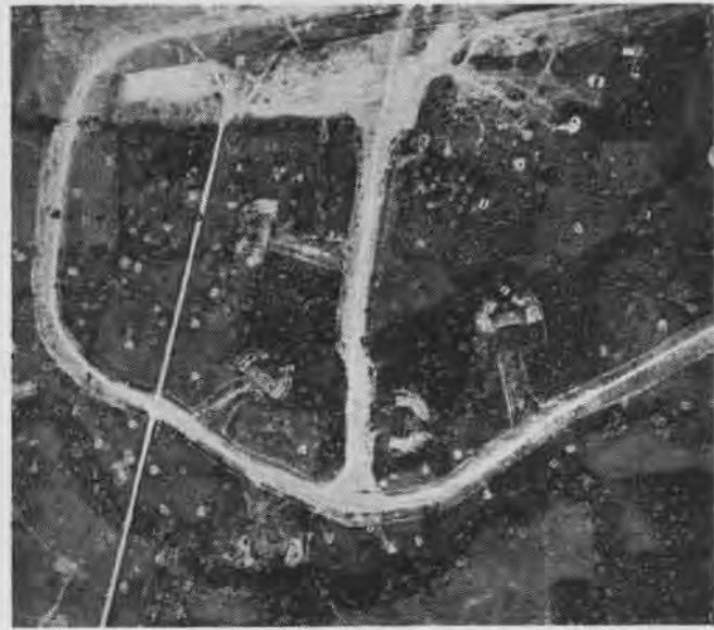
Covers of interlaced poles were built over revetments by enemy. Nets and foliage also were utilized to camouflage Jap planes.
