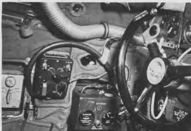
Echo of ship's radar pulse returns if IFF, showing at left of the picture, is turned on. In PB4Y-1 box is at left of pilot's position
