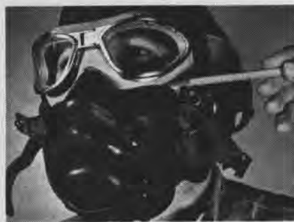
MARKING CUSHION RESULTS IN TIGHT FIT
