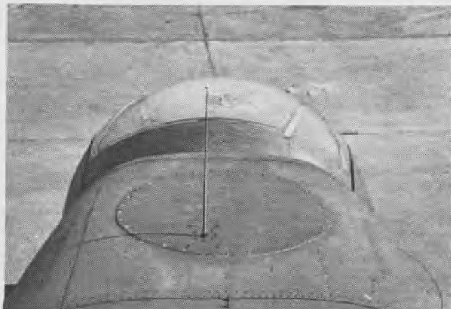
Land-based as well as carrier planes need IFF. This PB4Y-1 has two IFF antennas, one aft of nose turret, the other aft of plane's wings
