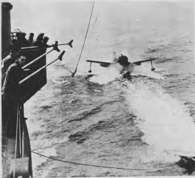
CORRECT TIMING of plane to ship's movement is the secret of Charlie recoveries. Here, a plane lands in slick, heads for the sled
