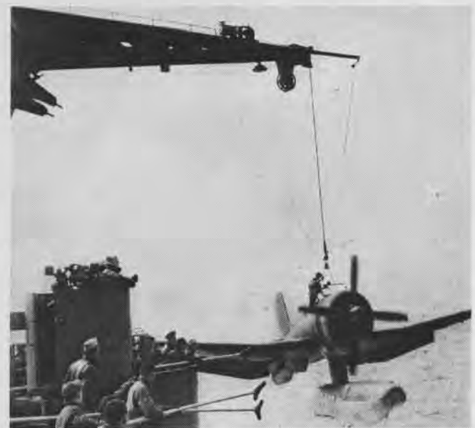
WINCH RIGGED over a boom hauls plane aboard, finishing successful Charlie recovery. In Dog recoveries, ship maintains course
