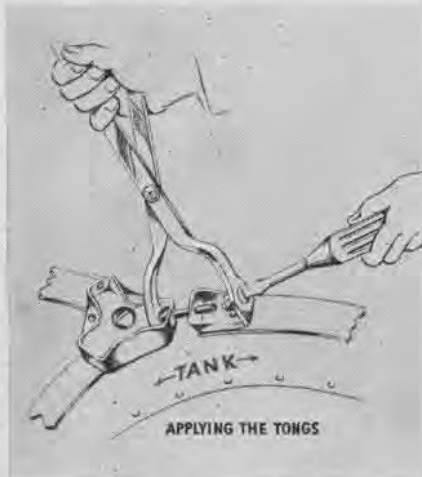
SPECIAL TONGS MAKE INSTALLATION EASY
