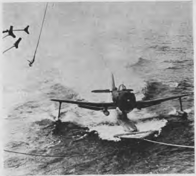
PILOTS SHOULD taxi up wake of the sled until main float of plane is well up on net. Cutting engine causes sled to snag on the hook
