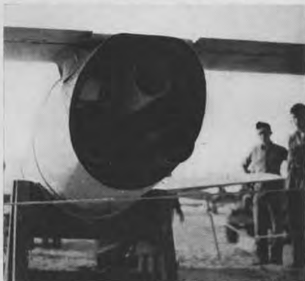
REAR VIEW OF BAKA BOMB SHOWS ROCKET EXHAUST CHUTES
