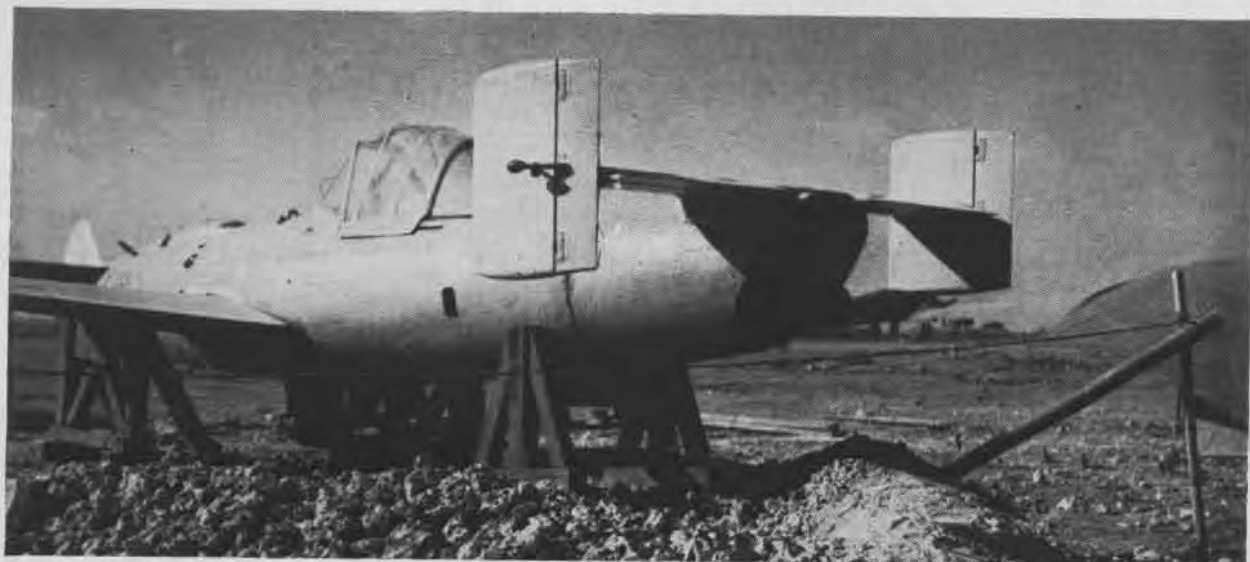
STUBBY BOMB SLIGHTLY MANEUVERABLE, WITH RANGE AROUND 50 MILES AND SPEEDS UPWARDS OF 500 MILES AN HOUR
