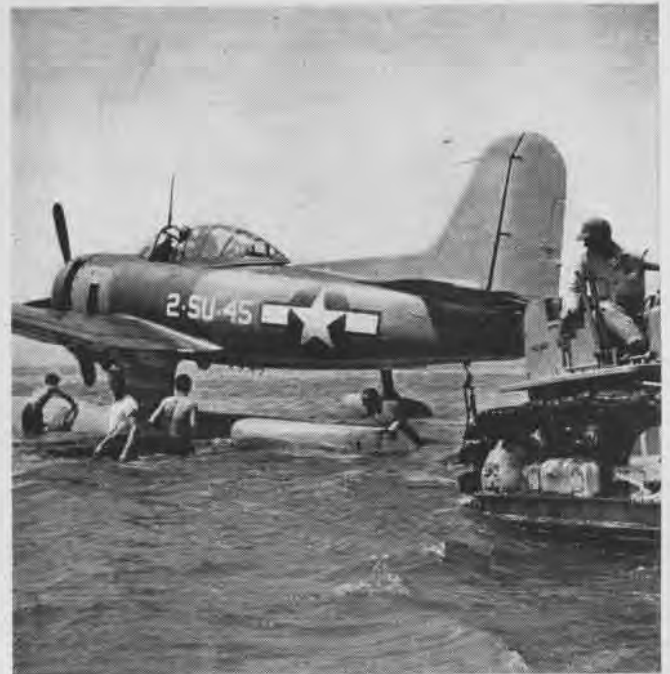
PILOTS GAIN experience in beaching during their training period. Crew clamps wheels to main pontoon, tractor hauls plane up ramp
