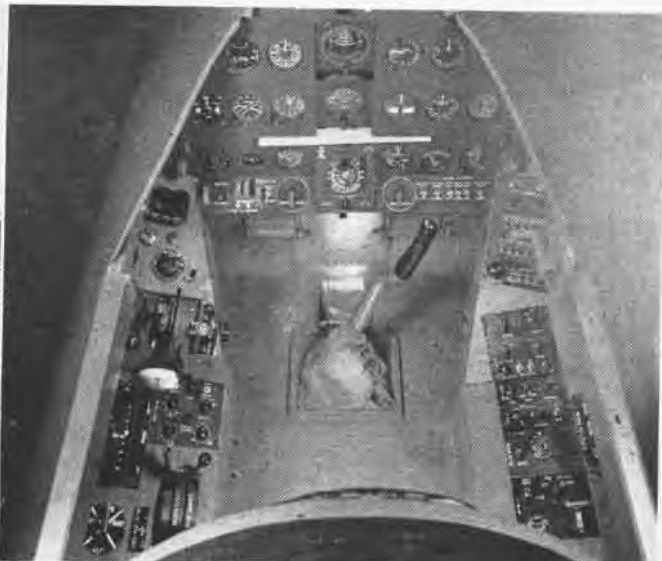
Arrangement in instrument panel mockup is more restful to pilot's eyes, is easier to work and contains fewer hazards than real plane
