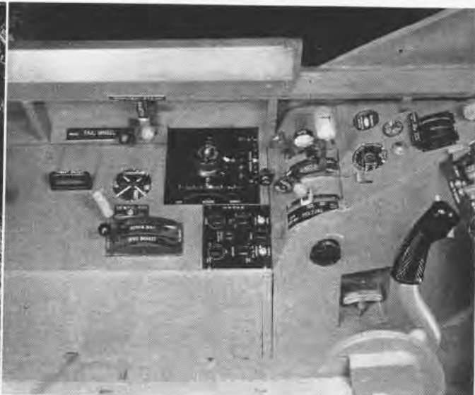
Shape of bomb bay, flap, supercharger and wheel controls makes possible easy identification in cockpit made by Special Devices
