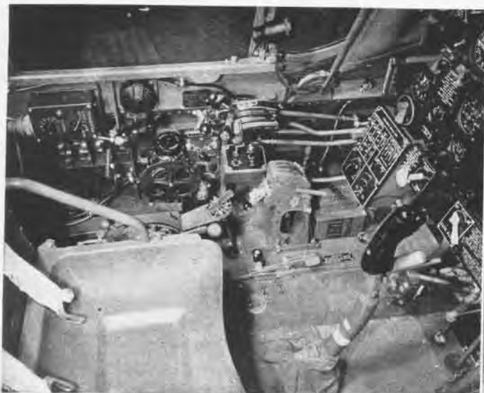
Irregularity of console in operational craft (above) differs sharply from that of mockup (right), showing rearrangement of controls
