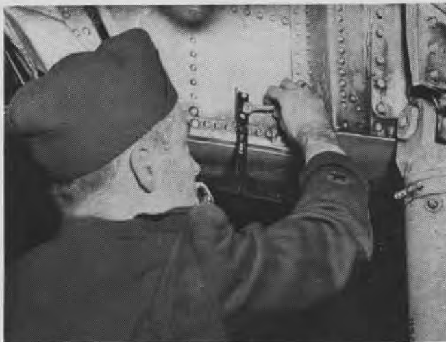
Boresight fittings provided by manufacturer determine plane's boresight datum line. On TBF or TBM planes ordnancemen must check erection manual to be sure correct boresight bracket is used. One set of fittings is provided for each six airplanes
