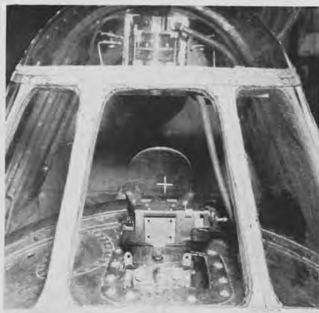
SMALL CROSS ON WINDSHIELD ACCURATELY MARKS LINE OF SIGHT
