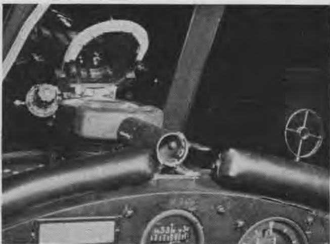
Countersunk mount developed in the Fleet for Mk. 8 sight in Avenger eliminates necessity for frequent removal. Older Mk. 8 mounts in TBF (M) type airplanes placed sight over a portion of instrument panel. Countersunk mount is permanently fixed
