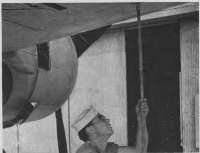
Ordnanceman uses hydraulic jack to level wing of Wildcat during boresight operations at NAS Norfolk. In boresighting plane the AOM should check pressure of airplane's tires to be sure they are inflated to pressure required in the erection manual
