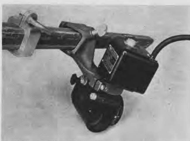
Reference ring holds Mk. 9 sight in use position on PV-1 type airplane. When sight is not in use, pilot may slide it to one side on mount bar. Reference ring on bar always remains in position, insuring fast, accurate adjustment of Mk. 9 when needed
