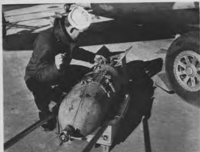
After installing Mk 2 wire in nose fuze, pass second strand of arming wire on back through aft bomb lug toward the tail fuze
