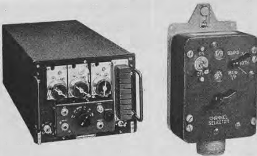
TRANSMITTER-RECEIVER UNIT OF NEW VHF (LEFT) AND CONTROL BOX OF UNIT (RIGHT)
