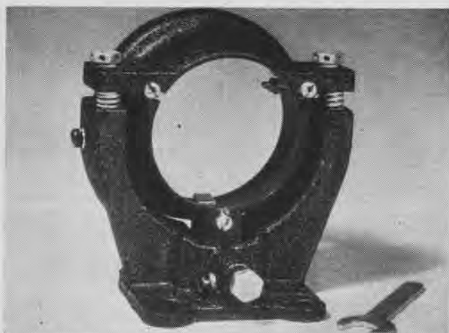
Base of Mk. 8 illuminated sight shows azimuth and elevation screw adjustments with wrench used for work. In boresighting, tension must never be entirely removed from springs around screws. AOM adjusts first in azimuth and then for elevation
