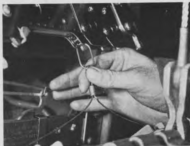
Swiveled loop of the Mk 2 arming wire is hooked into arming holder of bomb shackle. Removal of safety cotter key comes last
