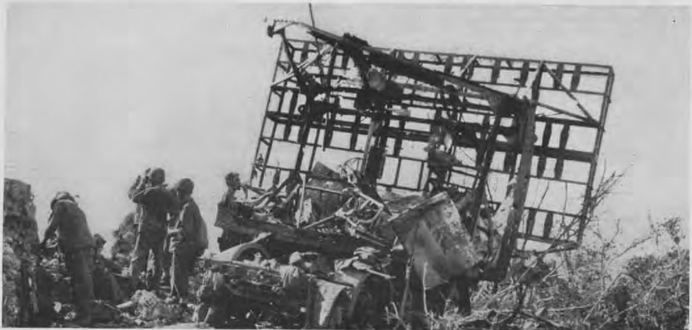
Mobile Mattress -type of enemy radar is mounted on Japanese army trailer. It has box screen, is used widely for land-based search
