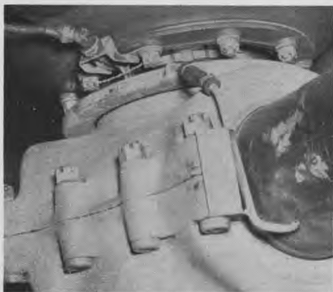
LINES ON CRANKCASE FLANGE MARK CORRECT PROPELLER SETTING
