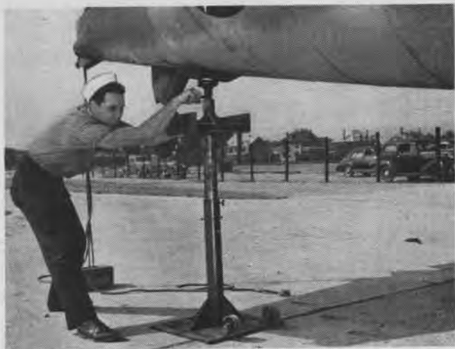
AOM uses jack to elevate fighter's tail preparatory to boresighting. Tail of plane must be elevated when necessary to bring boresight brackets in alignment with proper markings on screen erected for use with particular plane being boresighted
