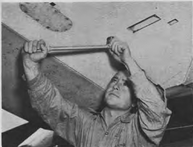
Vibration and operational shocks will throw guns and sights out of alignment. An alert aviation ordnanceman will check lugs securing fixed guns at every opportunity. An ASDevLant AOM tightens lugs on an Avenger . Some planes have lock washers
