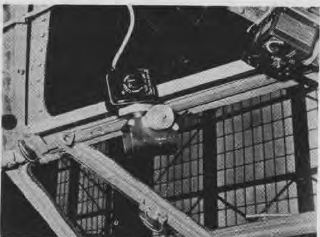
This Mk. 9 sight with tilting reflector head requires accurate adjustment for use in low level bombing. Bar mount with adjustable reference ring (PV-1 change No. 157) holds sight in place. NAS Patuxen River perfected this reference ring design
