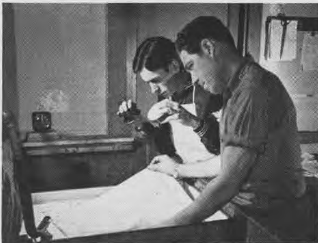
Special enlargers for making prints of microfilmed plans have a reel device which facilitates handling the many feet of film. A transparent type of paper can be secured and, with it, activities can produce any number of extra copies by the blueprint method
