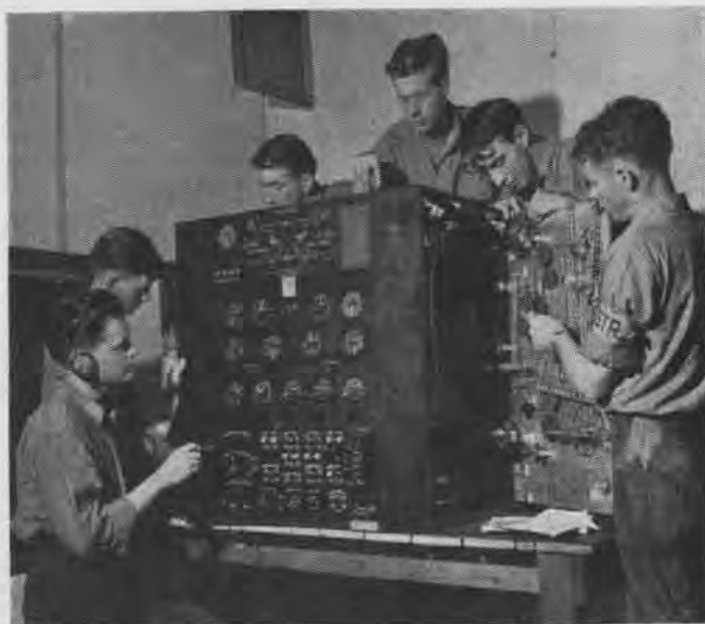
Students learn to operate and maintain the Flight Engineer's Panel during the twelfth week of their course. This device, used to train pilots and flight engineers in twin-engine plane operation, must be mastered. Instructor is a former trainee
