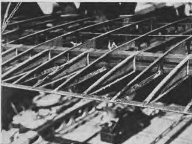
Lower right wing of an F-5-L flying boat shows mold and rot caused by water and long service during maneuvers at Guantanamo
