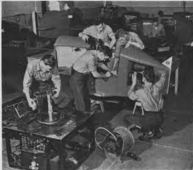
Putting the "do the job yourself" principle in operation, these artificer trainees dismantle a Link Trainer. In an adjustment shop trainees find and correct maladjustments created by the instructors. On air stations these men will maintain devices
