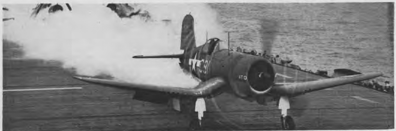
JET-ASSISTED TAKE-OFF DEVICES ENABLE AIRCRAFT TO TAKE THE AIR UNDER OVERLOAD CONDITIONS NOT THOUGHT POSSIBLE SEVERAL YEARS AGO
