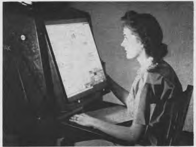
With readers such as this, checking the microfilmed plans is not at all difficult. From its reel the long roll of film can be fed through the viewing machine which projects image of the film on the glass. Operators check reels against list of airplane parts
