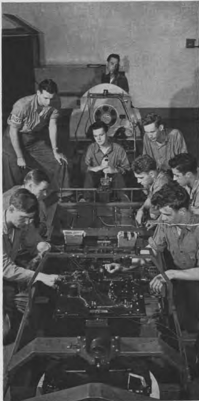
Trouble shooting becomes second nature to trainees at Special Devices School. Trainees at work on the Gunairstructor during the fourteenth week of their course make delicate adjustments on the movie unit. Students operate Gunairstructor
