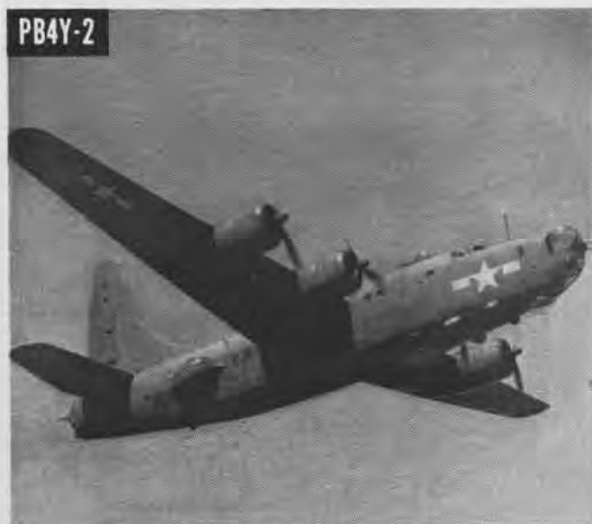
SINGLE FIN AND RUDDER GIVE SINGULAR APPEARANCE TO NEW PB4Y-2
