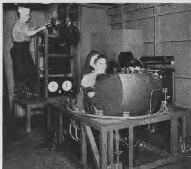
CARRIER EMPLOYS 3-A-2 DUAL PROJECTION TRAINER WITH TBF TURRET
