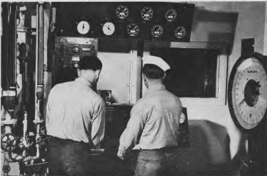
CONTROL PANEL FOR ENGINE TEST STAND; ARV (E) IS ONLY NAVY SHIP WITH A STAND
