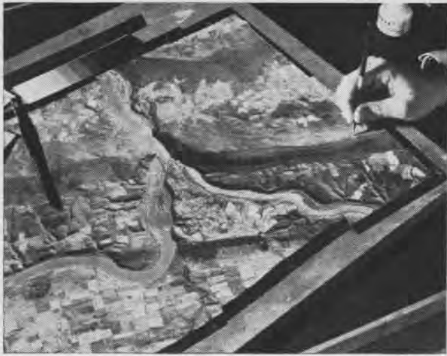
1 Photo surface model process begins with preparation of photo mosaic of area to be covered. From this mosaic, a copy negative and positive transparency are made on ordinary film
