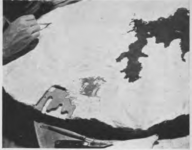
2 Clay-covered model is placed on enlarger table. Positive transparency is projected on clay and this image guides modeler as he creates the general detail of the terrain's contours
