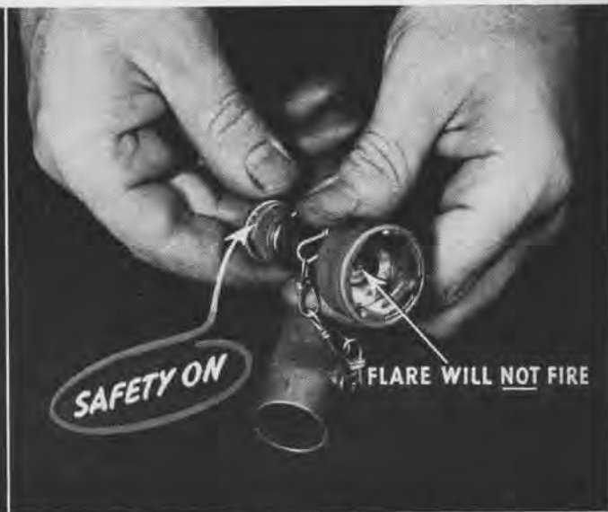
THICKNESS OF SAFETY PREVENTS PIN FROM GOING BEYOND THIS
