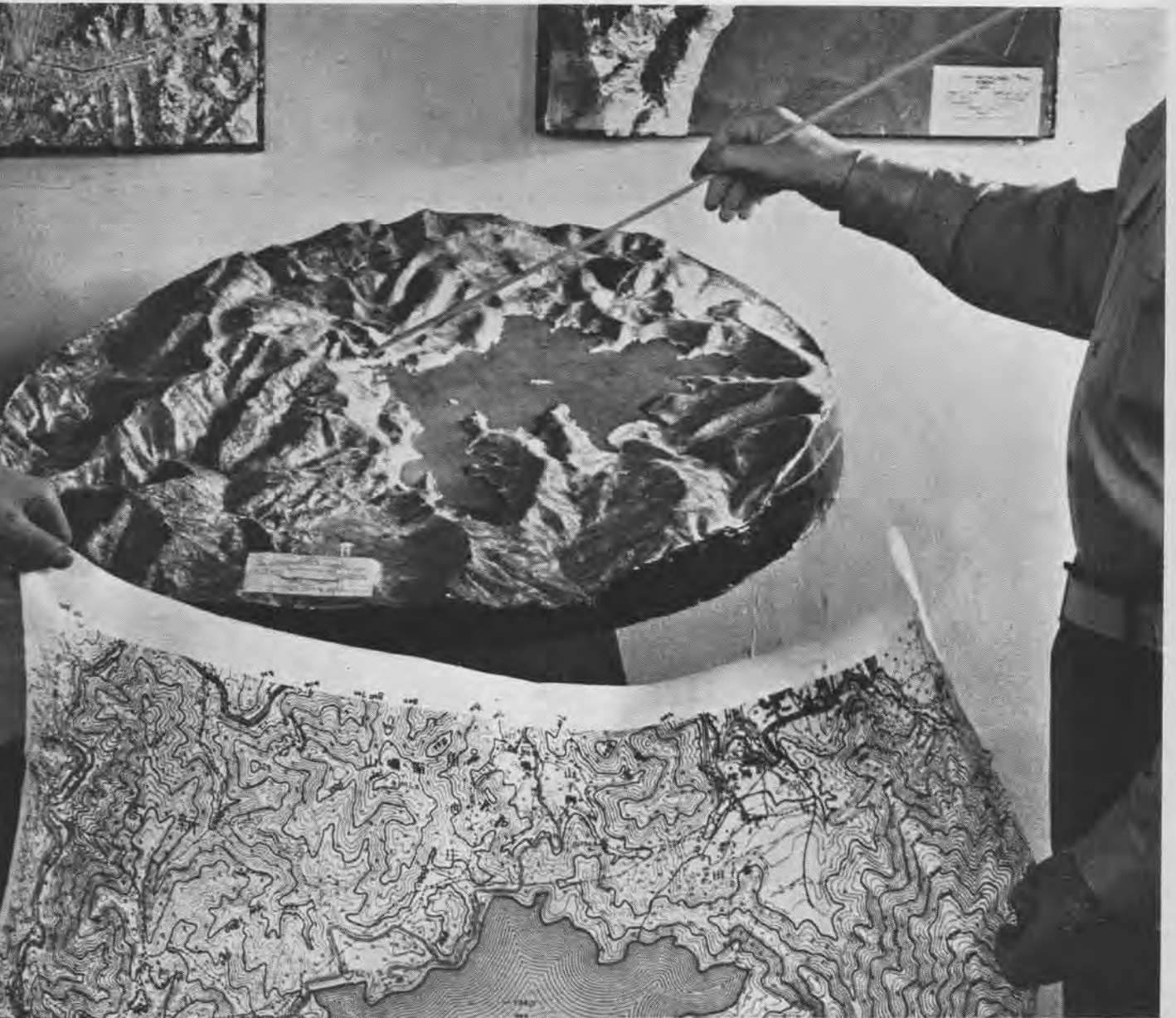
PHOTO SURFACE MODELS ARE AERIAL PHOTOS SUPERIMPOSED ON THREE-DIMENSIONAL CLAY MODEL. FLAT MAP BECOMES MODEL (ABOVE)
