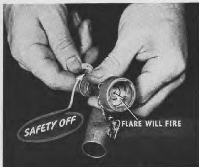
INSIDE OF PISTOL SHOWS PIN IN POSITION TO STRIKE PRIMER
