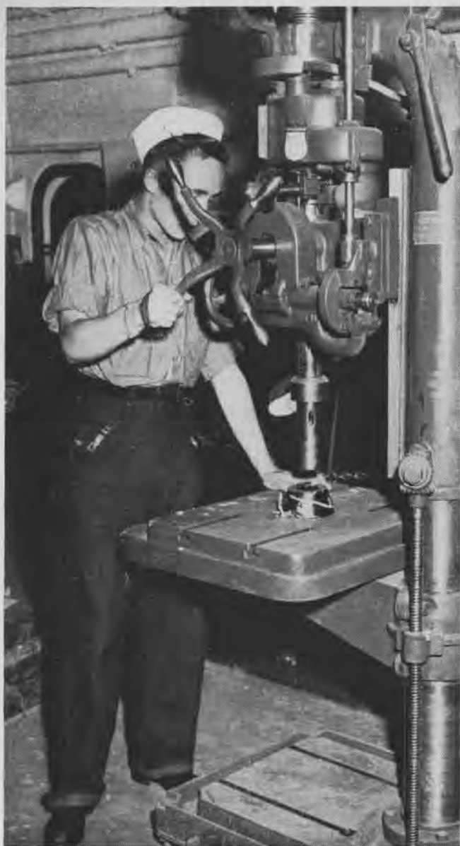
Crewman operates drill press aboard one of the A type aircraft repair vessels. The A and E types team up in pairs, between them providing almost every type of machine to fix damaged planes
