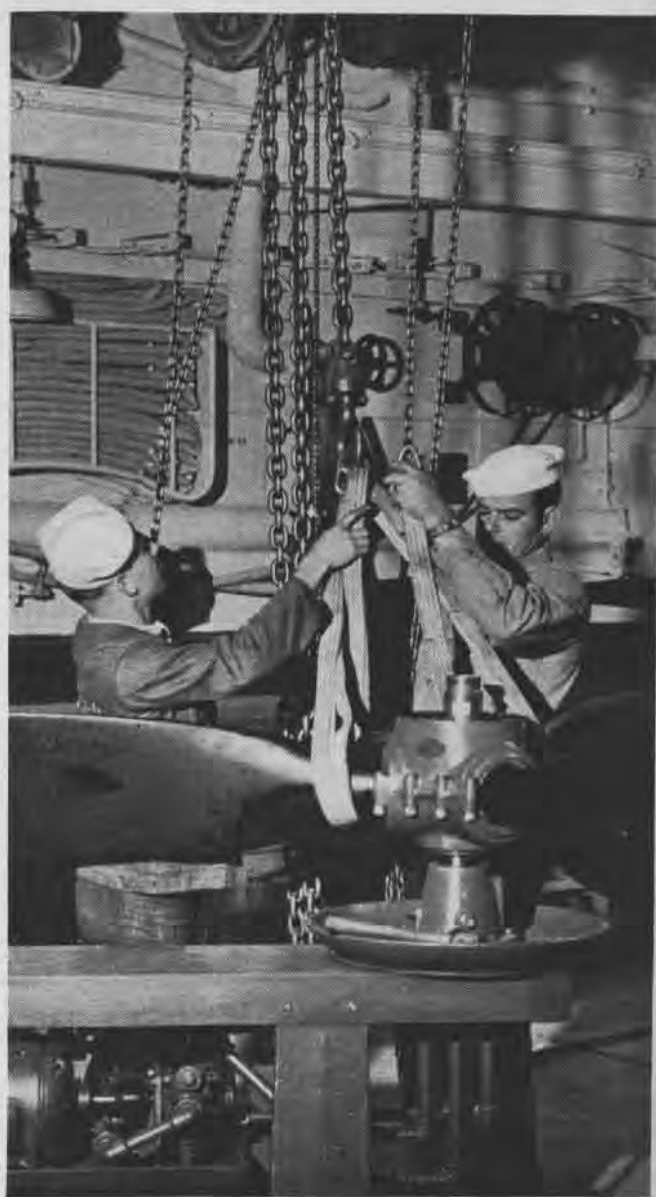
Propeller shop on ARV is equipped to do major repairs. Here crewmen adjust sling on a Hamilton Standard propeller. Overhead hoist can travel the whole length of the ship machine shop
