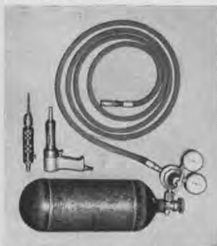
RIVET GUN WILL HANDLE SMALL JOBS WELL
