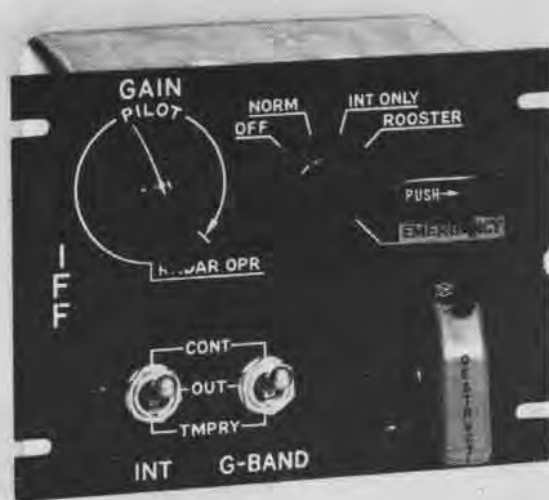
FLIP OF CODING SWITCH ON IFF TO EMERGENCY SENDS TROUBLE SIGNAL OUT 100 MILES
