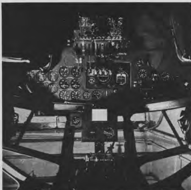
Pilot and co-pilot at their stations in PBM-3 OFT have all instruments and controls of the real aircraft, insuring realistic training that hitherto has not been possible in ground instruction
