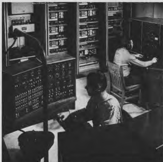
Operator's and radioman's station permits the setting up of emergency flight conditions for solution by coordinated crew action and the observation of flight and navigation techniques and errors
