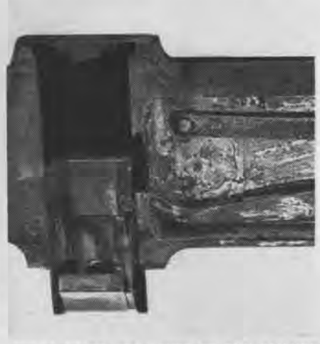
RUSTY PARTS ARE CAUSE OF GUN FAILURE
