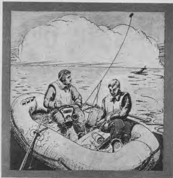
Ditched survivor holds "Gibson Girl" radio transmitter between his knees and sends international distress signal; kite holds antenna
