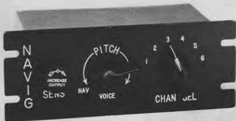
AN/ARR-2 EQUIPMENT PROVIDES SIGNALS TO LEAD THE AIRCRAFT BACK TO THEIR BASE
