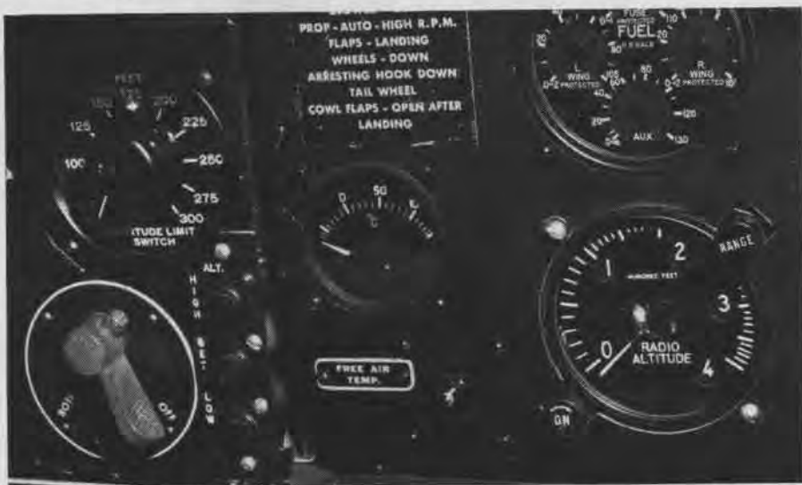
RADIO ALTIMETER HELPS KEEP PILOT OUT OF TROUBLE; RED SIGNALS WHEN TOO LOW
