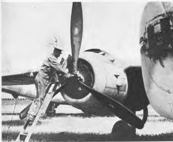
PAINTING THE PROPELLER AND ITS COMPONENTS PREVENTS RUST
