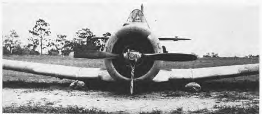
COLLAPSING WHEELS ALLOW PLANE TO SIT ON SAND BAGS, PREVENT ROCKING IN STORM
