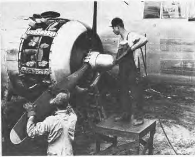
EACH ENGINE WITH LESS THAN 100 HOURS IS PICKLED ON PLANE
