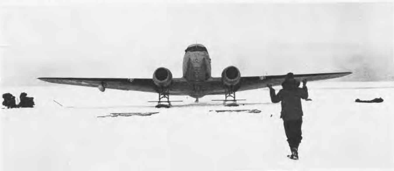
FAST TAXIING KEPT SKIS FROM FREEZING SOLIDLY TO SNOW; OIL-SOAKED PLANKING KEPT SKIS FROM CONTACTING SURFACE
