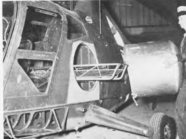
Aluminum blister caps clamp on over exposed ends of the stretcher; Plane can be loaded and caps clamped on in a matter of minutes
