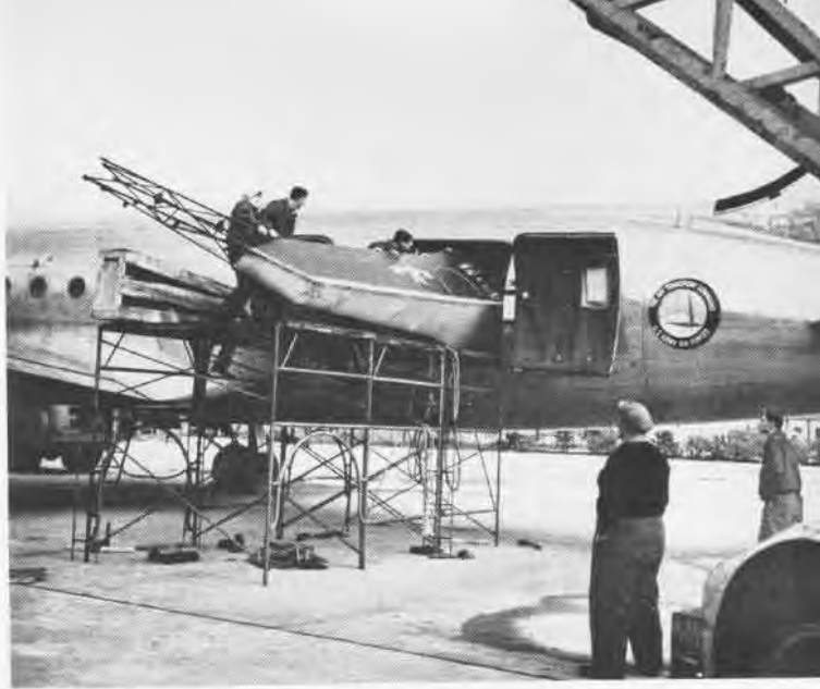
Coast Guard crew loads a helicopter aboard an Army transport plane. The loading job takes five men 90 minutes to complete
