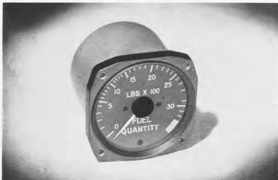
FUEL QUANTITY INDICATOR SHOWS GAS TANK CONTENTS IN POUNDS INSTEAD OF GALLONS
