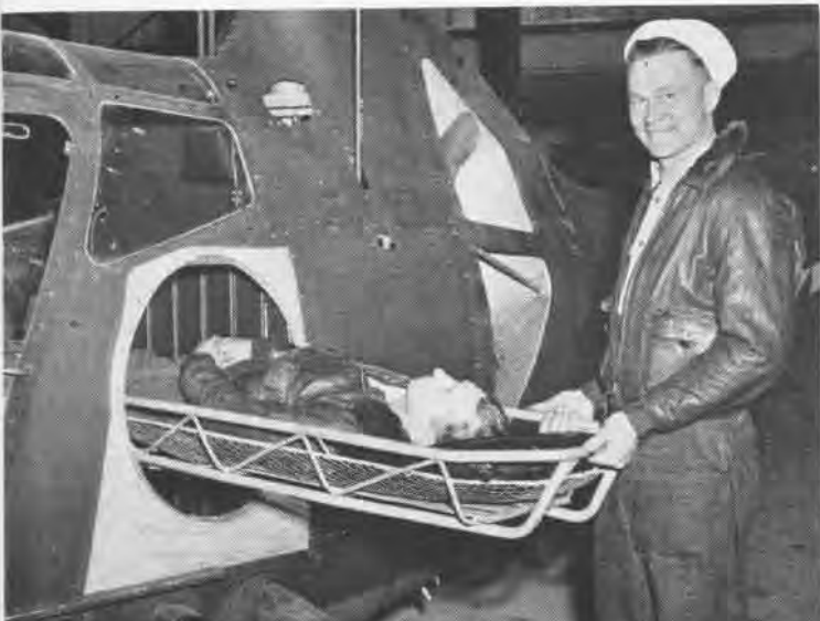
Compartment behind the pilot provides ideal slot for a Stoke's stretcher. Ends of the stretcher protrude on either side
