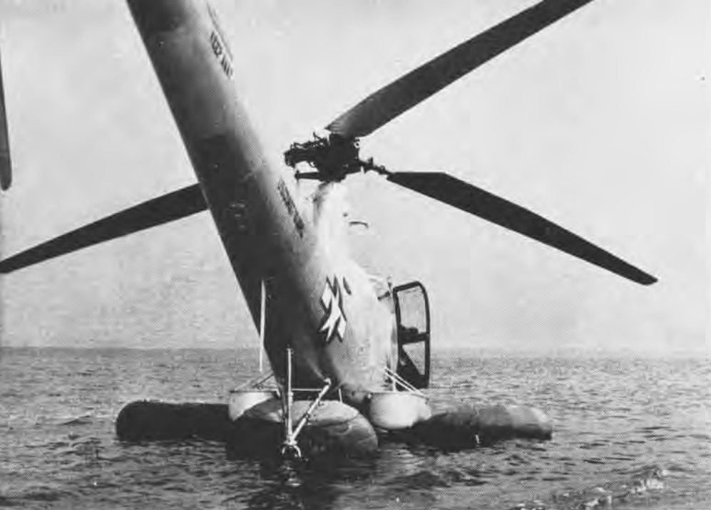
WITH ITS EMERGENCY GEAR INFLATED THE HELICOPTER FLOATS LIKE A DUCK ON WATER
