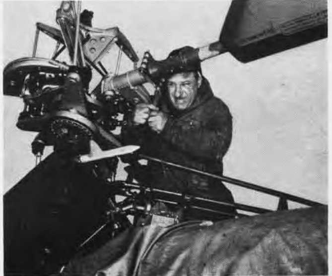
Maintenance men kept planes in flying condition regardless of the weather. Here a technician attaches blade on a helicopter.
