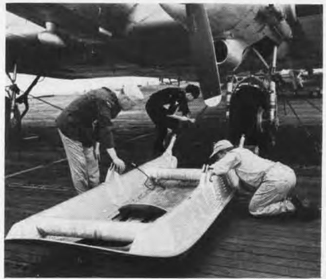
Aboard Philippine Sea technicians install metal skis on R4D-5's so airplanes can land on the snow of Ross Sea ice shelf.
