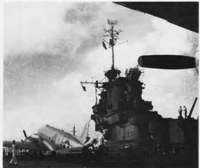
Six R4D-5's made JATO take-offs from flattop and landed on snow at Little America. These planes were left in Antarctica.
