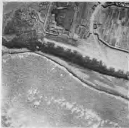
PHOTOGRAPHS OF SAME JAPANESE BEACH TAKEN AT VARYING TIDE LEVELS: THIS TYPE PHOTOGRAPH WAS USED IN WATERLINE METHOD
