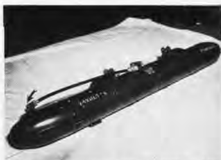
ELECTRICAL CONNECTION PUT AT END OF RACK
