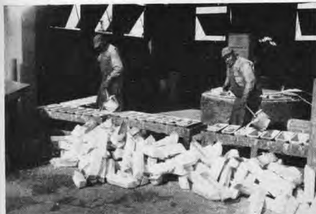
SALVAGED ALUMINUM FROM PLANES GOES INTO 17-POUND MOLDS AT YARD
