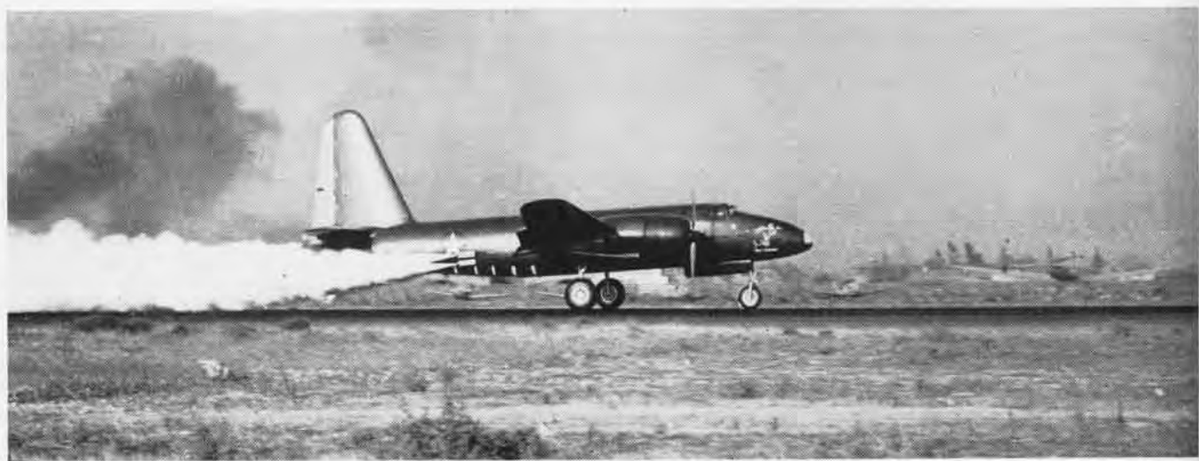
TRUCULENT TURTLE, NAVY'S MOST FAMOUS AIRCRAFT, TAKES OFF WITH SHORT RUN BY USING JATO. BELLY STRIPES MEASURE DUMPING OF GAS
