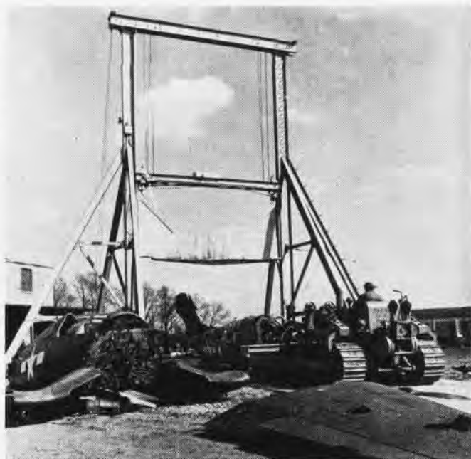
6100 POUND CHOPPING BLADE DESCENDS TO CUT FUSELAGE OF AN 582C
