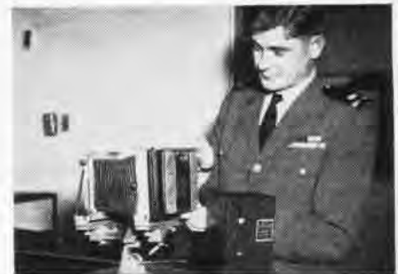
35 MM. MAGAZINE FITS INTO BACK ADAPTER
