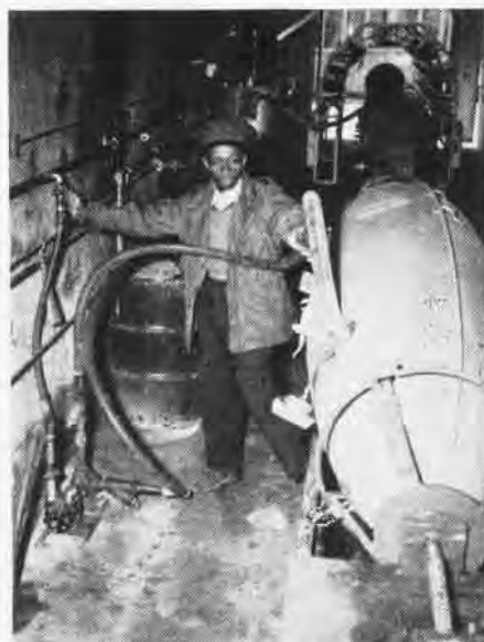
THREE DEGREASING SOLVENT BATHS ARE USED
