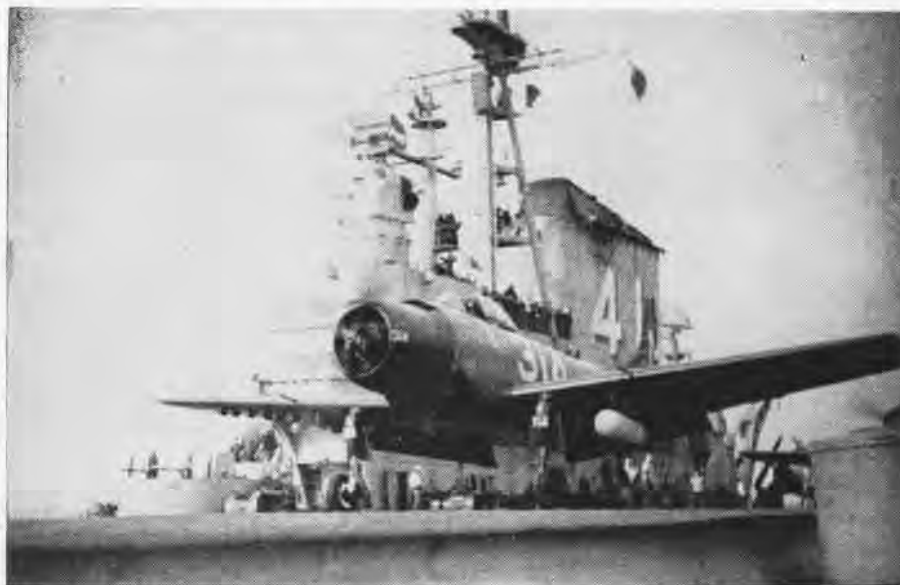
AD-1 SKYRAIDER TAKES OFF FROM MIDWAY DECK; STRENGTHENED PLANES PASSED TESTS ON CVB
