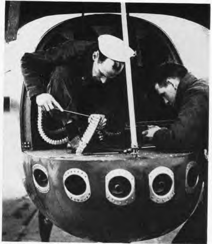
Six 20 mm cannons in nose of P2V-2 are easily accessible for ordnancemen Vickers and Sokolis of VP-ML-7 to do repairs on
