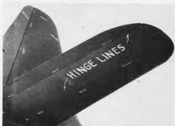
One unique feature of P2V-2 is the varicam tail, which really gives it two elevators and increases its flight maneuverability
