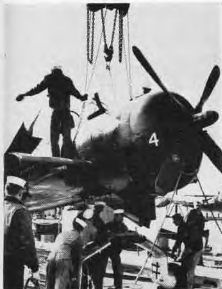
FUSELAGE IS LOWERED ONTO PLANE'S WHEELS
