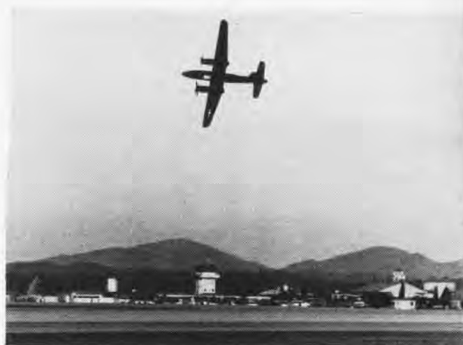
Long, thin wing and distinctive nacelles make P2V-2 easy to recognize; here it demonstrates fast rate of roll at Miramar
