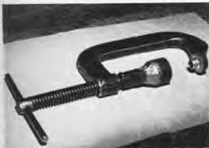
CLAMP IS ADAPTED TO REMOVE DZUS BUTTONS
