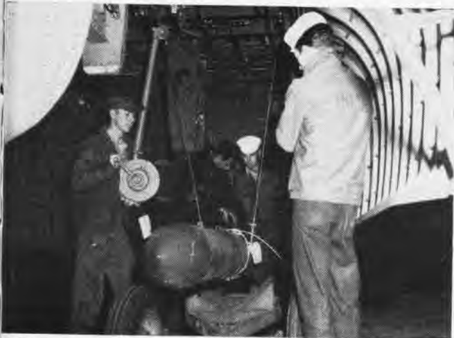
Ordnancemen like to work in roomy bomb bay of Neptune ; here VP-ML-8 men practice hoisting 11.75" rocket in bay
