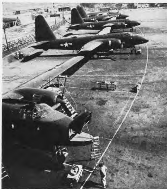
New Neptunes at Lockheed show accessibility of nose guns for rearming; three-bladed paddle props on newer models
