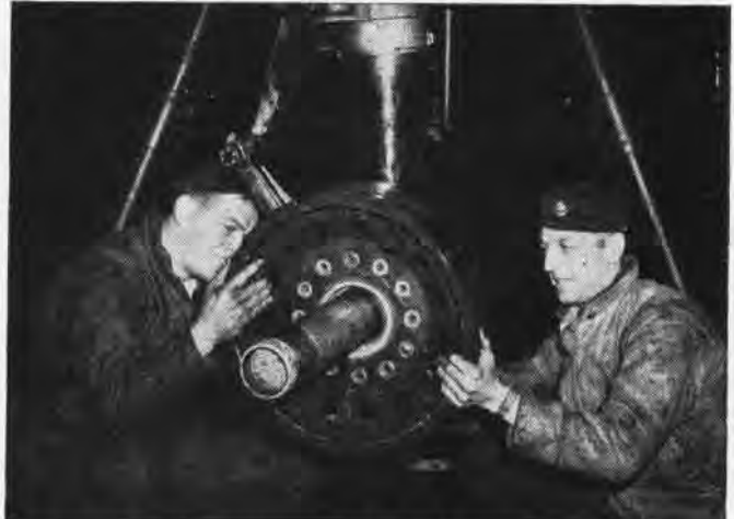
Two mechanics of VP-ML-7, J. L. Carpenter AD1, and L. G. Judas, ADC, change brake expander tube on wheel of a P2V-2
