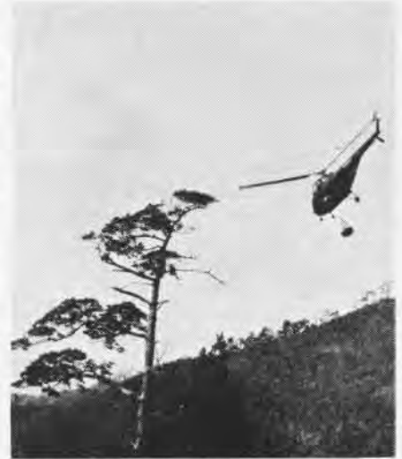
OFF GOES the salvaged engine, dangling in net slung below VMR-161 transport pinwheel
