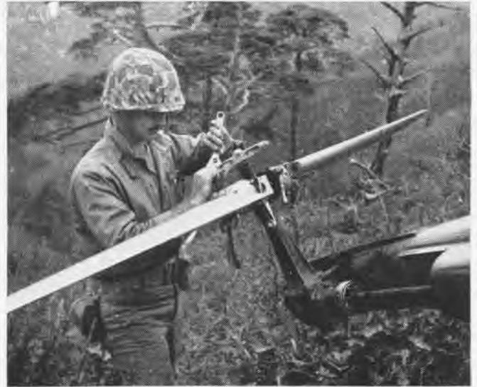
SGT. ROSSON removes tailrotor from damaged tail section of the helicopter; VMO-6 needed spare parts from the helicopter
