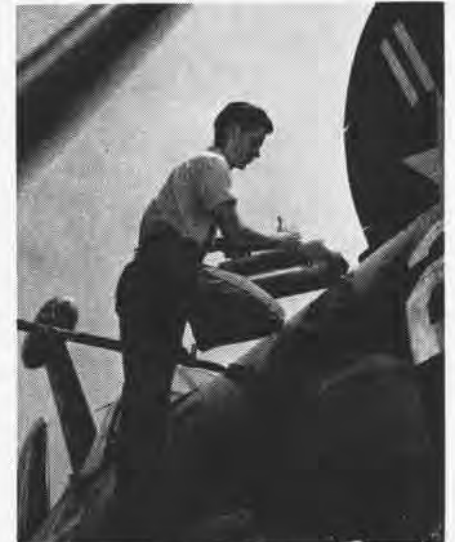
AIRPLANE engines have a habit of eating up oil; here Norris changes plane oil supply
