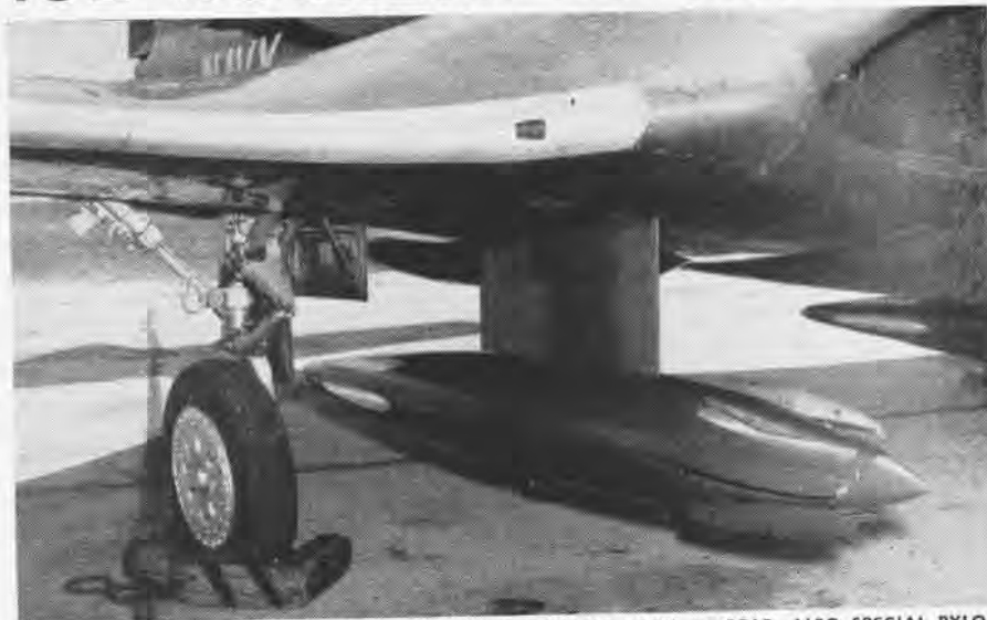
CLOSEUP OF LAUNCHER SHOWS EXIT DOORS OPEN, EXHAUST PORTS AT REAR, ALSO SPECIAL PYLON
