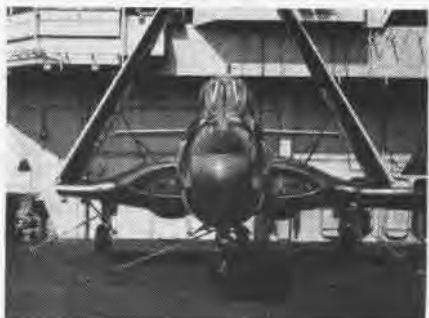
HERE AN F2H IS HELD WITH THE NEW TIE-DOWN
