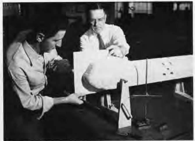
AT WORK IN THE model-making shop—Supervisor Hansen watches H. W. Klotz fit a template to the nose of a helicopter model
