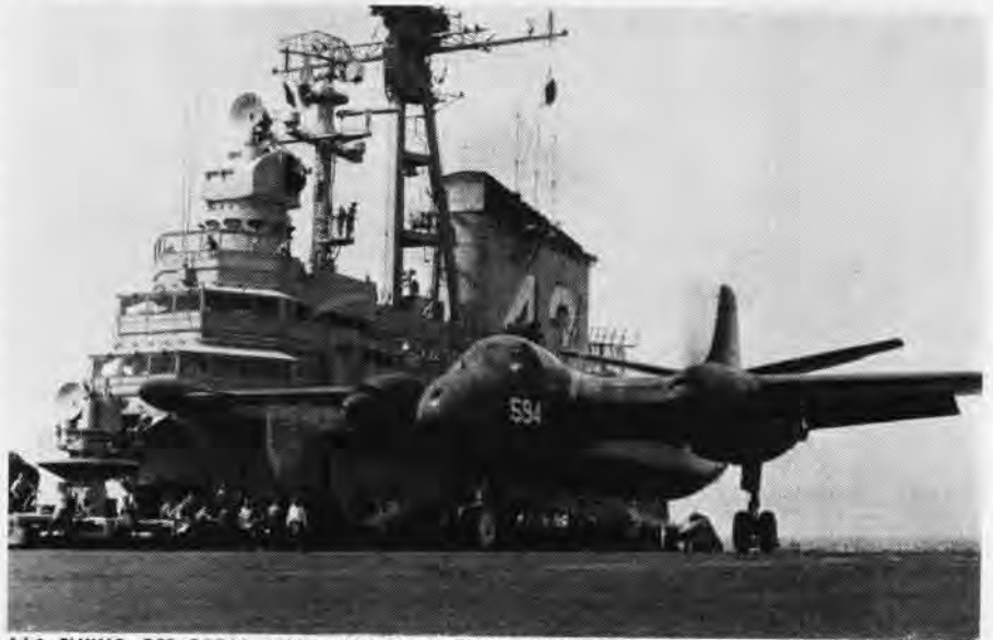
AJ-1 FLYING OFF CORAL SEA'S DECK IS HEAVIEST PLANE DESIGNED TO OPERATE FROM FLATTOP
