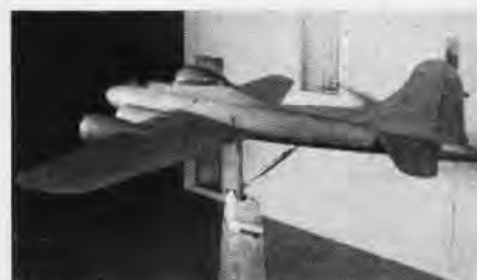
DTMB ENGINEERS found that this radome configuration worked best on PB-1W model
