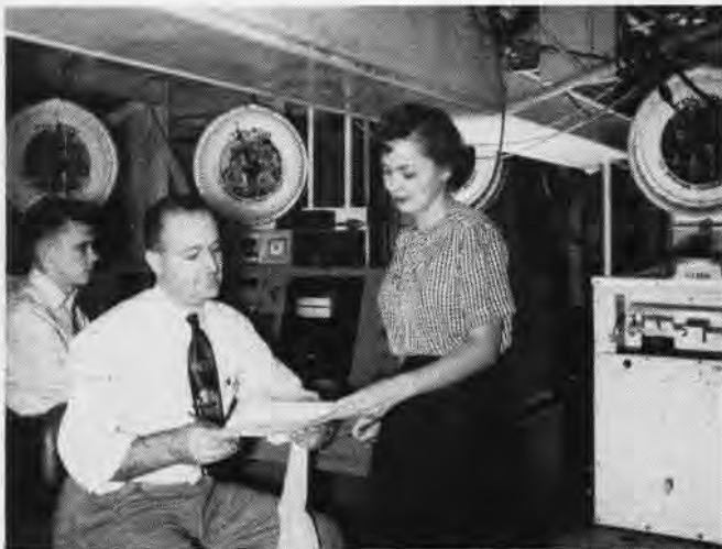
LOW-SPEED WIND tunnel control room—C. L. Benedum checks data with E. Muller (note balance ring above and scales rear)
