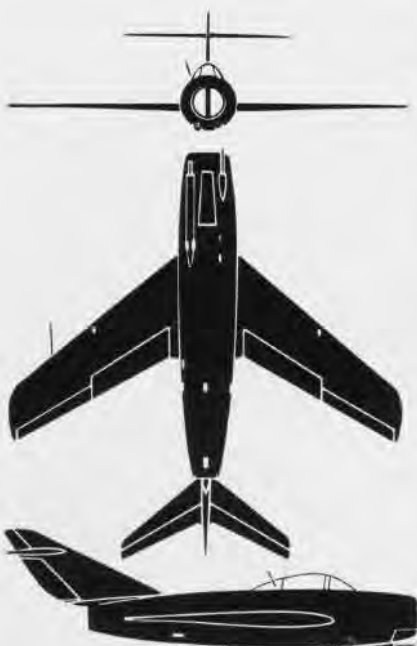
MIG-15 HAS MID-WING, DROOPY TAIL SURFACE
