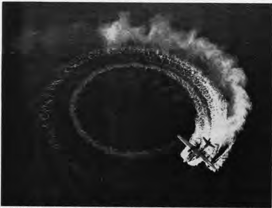
WHEN THE XP5M-1, which has a long hull that rides in the water, first came out, onlookers wondered if it would be able to turn in the water. To speed up this process, the Glenn L. Martin company installed underwater rudders and brake near the tail which operate somewhat like the dive brakes on an AD. Operated hydraulically, the hydroflaps enabled the Marlin to turn easier by using one, or to slow down by using both. The above picture employed dye marker to show the turning circle radius and was taken from a helicopter. When the hydroflap is set at 65°, the turning radius is about one and a half times the wingspan, about a third of the radius required when turning with the plane's engines alone.
