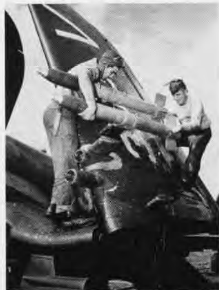
METAL STEPS HOOK INTO WING EJECTION CHUTE
