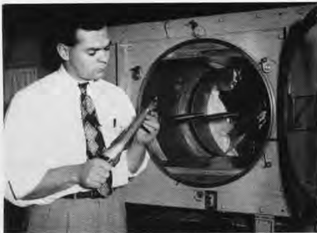
AERO-ENGINEER Patterson examines model before the 18" by 18" supersonic tunnel test section (note spherical Schlieren mirror)
