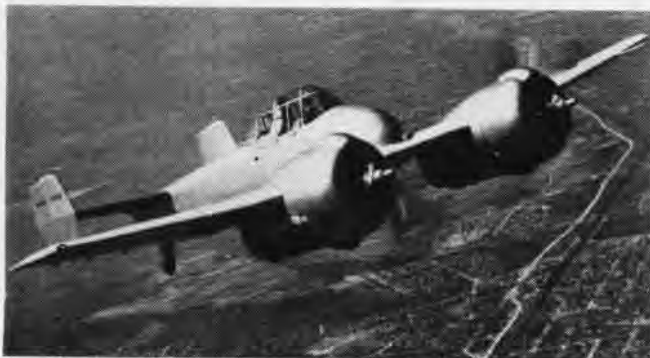
STUBBY LITTLE XF5F-1 SKYROCKET HAD HOOK BUT NEVER WAS ON A CV
