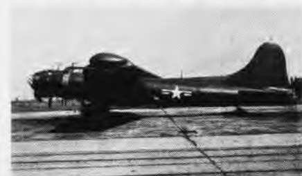
AND TODAY this Navy PB-1W (B-17) has DTMB-recommended radome configuration
