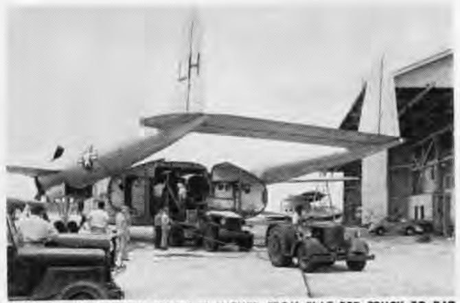
FUSELAGE IN WOODEN FRAME IS INCHED FROM FLAT BED TRUCK TO R4Q
