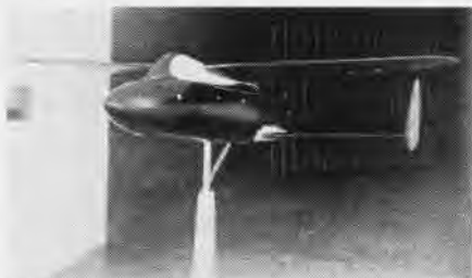
MODEL OF proposed 'wide-tail' plane—plasticine modifications show up in white
