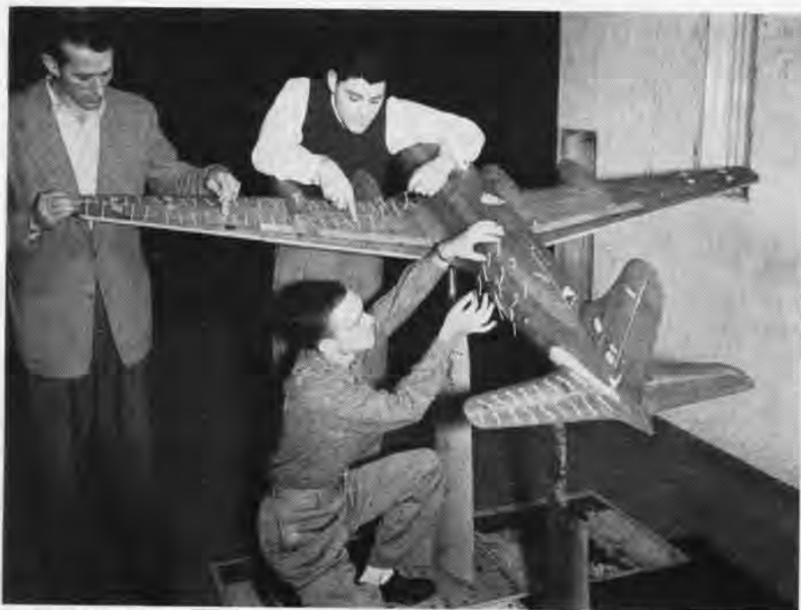
DAVID TAYLOR Model Basin engineering aides Simms, Rosenberg and Cottrill (kneeling) install tufts on R5D model for special air-flow tests in one of the 8' by 10' tunnels
