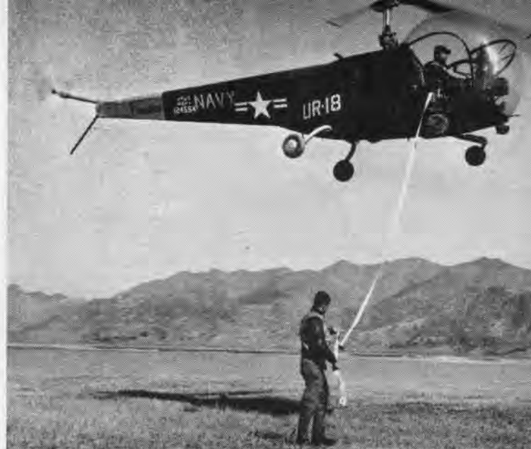
ANOTHER RESCUE sling was developed by 1st Lt. Gus Lueddeke of VMG-6 in Korea for helicopter work; Corp. McClain tries it out
