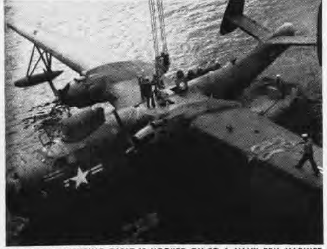
THE CURTISS' HOISTING CABLE IS HOOKED ON TO A NAVY PBM MARINER
