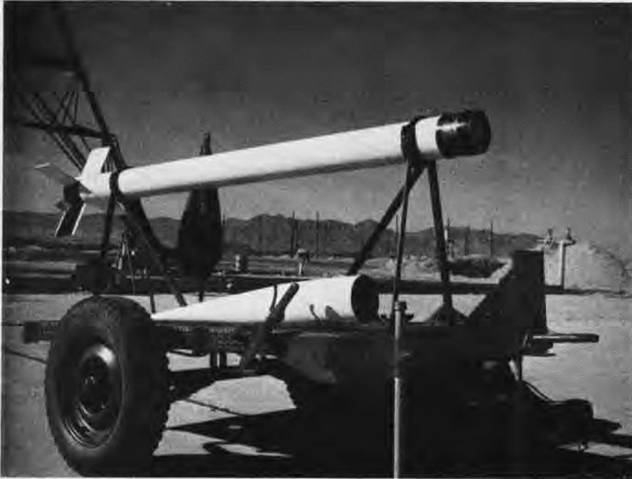
UPPER PORTION SHOWS TAIL, FIN, PARACHUTE CASE; LOWER, NOSE CONE FOR AEROLOGY GEAR
