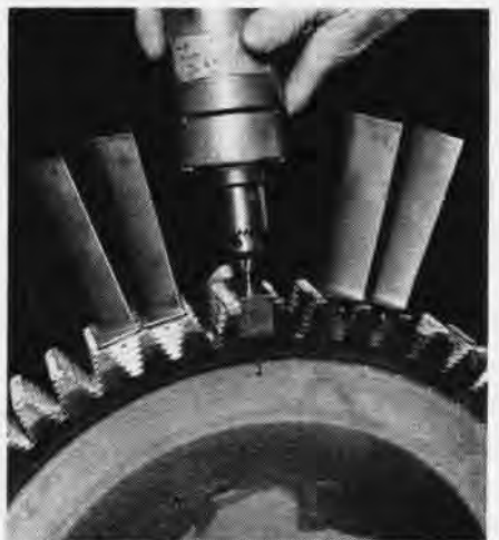
HAND JIG REMOVES TIGHT TURBINE PINS FAST
