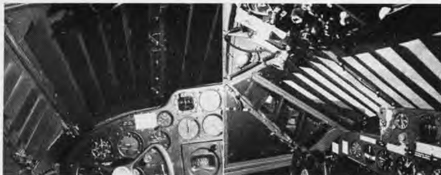
WHAT THE PILOT SEES WITH LOUVERS INSTALLED IS SHOWN, LEFT: CO-PILOT'S VIEW ON RIGHT
