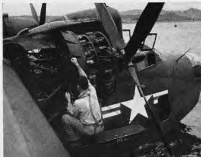
SEAPLANES ARE OFTEN REPAIRED AS THEY FLOAT AT THEIR MOORING
