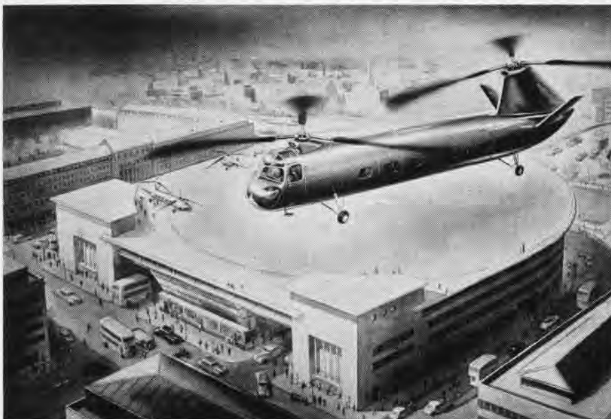
TWO ENGINES POWER THIS TWIN-ROTOR HELICOPTER IN ENGLAND: NOTE DIHEDRAL ON ELEVATORS
