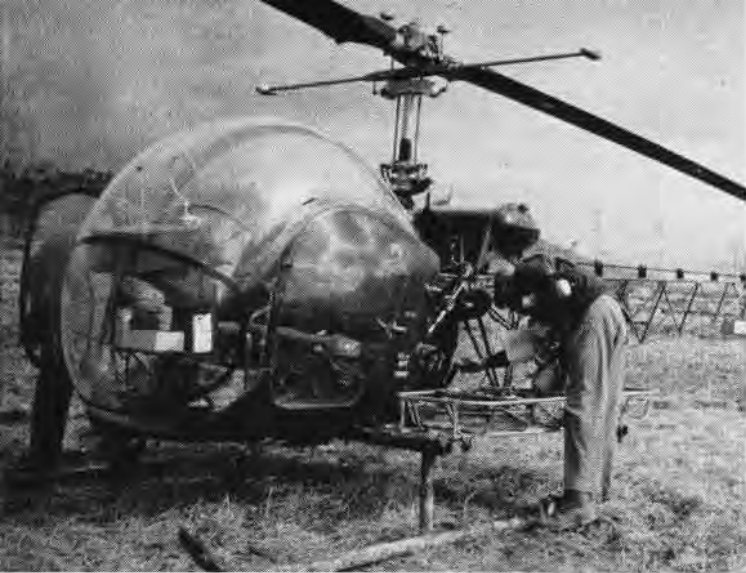
EQUIPPED WITH skids for landing on rough terrain, this Bell helicopter has two basket litters outside cockpit for carrying battle wounded
