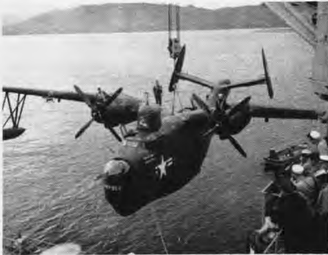
HERE THE MARINER IS IN MIDAIR DURING HOISTING PROCESS TO DECK
