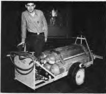
SCHINDLER AND HIS OXYGEN TRANSFER UNIT
