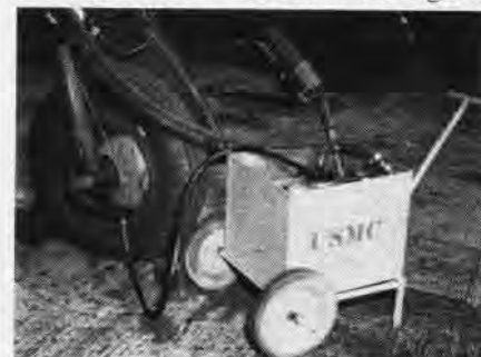
BRAKE BLEEDER DOES TWO OPERATIONS AT ONCE
