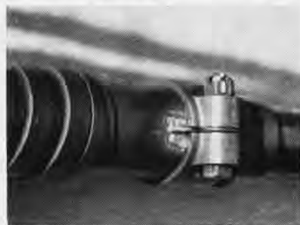
MODIFIED RECOIL SPRING SEAT OF AUTOMATIC
