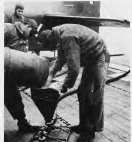
ABOARD BOXER —Navy ordnancemen mix napalm bomb solution being hosed into tank
