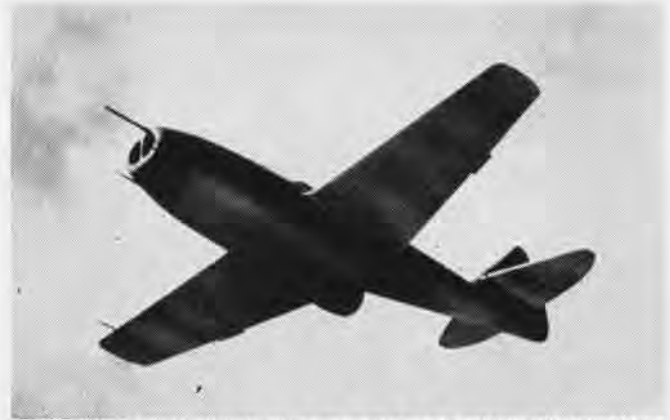
MIG-9 JET HAS TWO AIR INTAKES IN NOSE, TWO EXHAUSTS UNDERSIDE
