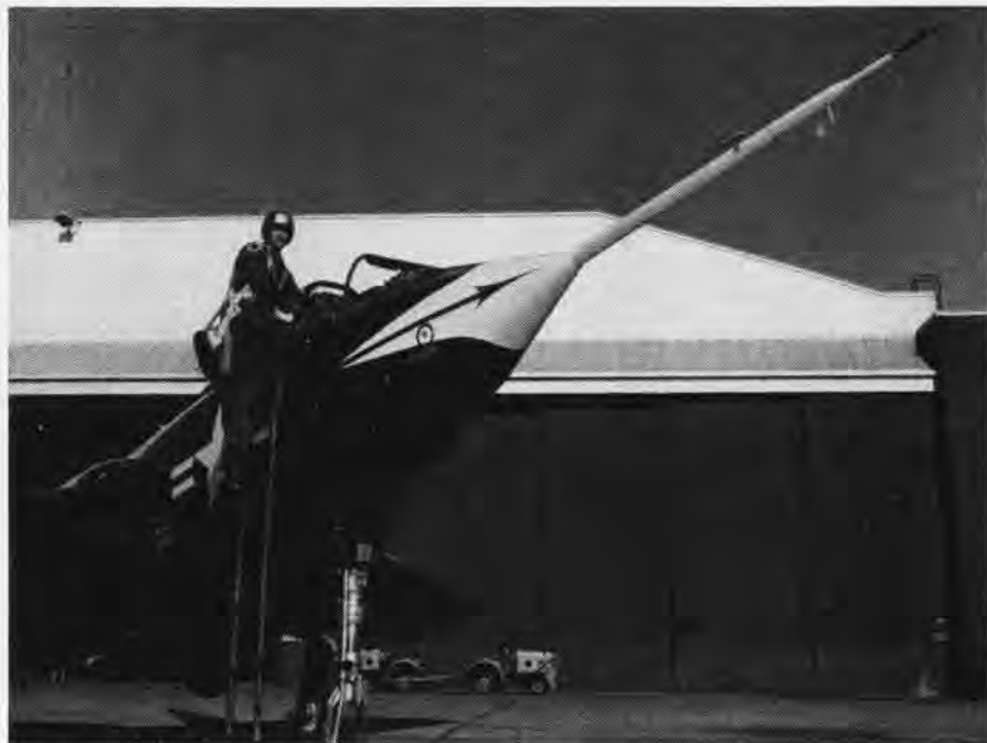
THE PILOT in the Navy's F7U Cutlasses has to be a minor mountaineer to ascend to the cockpit of his plane, via a 10-foot ladder. Here Lt. John W. Ryan, a BAR Dallas test pilot enters the cockpit of a Cutlass with a long flight test instrumentation nose tube. Various installations on it measure pitot pressure, pitot static, angle of yaw, angle of attack and temperature while the plane is in flight. The plane is a production model F7U-1.
