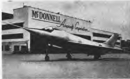
NEWEST jet plane in the Navy's fighter stable is this McDonnell XF3H-1 Demon, which made its first flight of 24 minutes in August. The plane is powered by an undisclosed Westinghouse jet engine in the fuselage.
