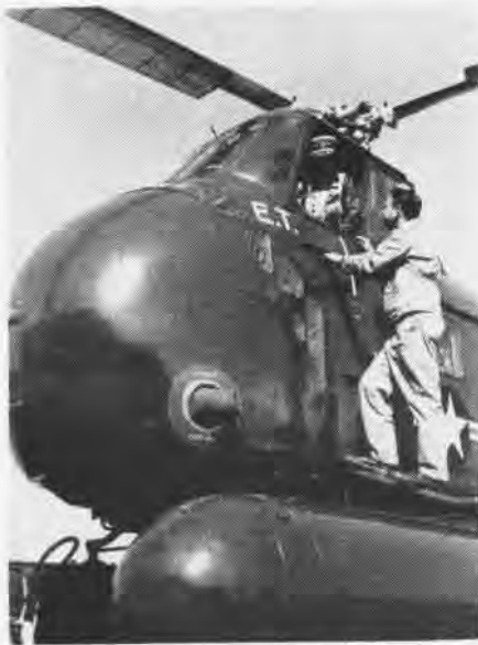
ONE OF THE Navy's newest helicopters is the HO4S, a 10-place pinwheel built by Sikorsky Aircraft. This photo, taken at NATC Patuxent River, shows the big plane with metal floats installed. Note placement of the engine in the plane's nose section.
