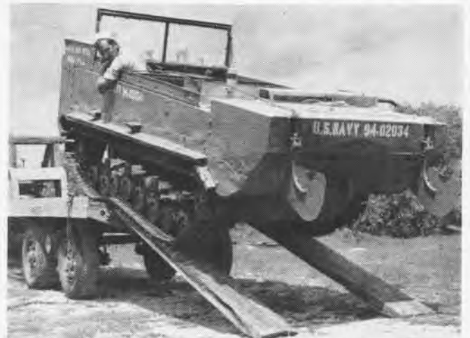
ANOTHER RESCUE unit, the Weasel, is taken as far as possible by truck and unloaded; note prop, rudders and caterpillar tracks
