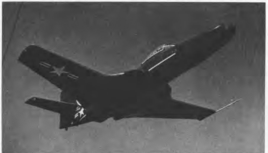
THE CYRANO de Bergerac of the airplane world is this new F2H-2P Banshee photographic aircraft. Its long nose is packed full of cameras for use in high and low-level aerial mapping. Some of the highest aerial photos ever taken were shot from a Banshee flying 51,000 feet over Washington, D. C. The Banshee night fighter version also is a long-nosed plane.
