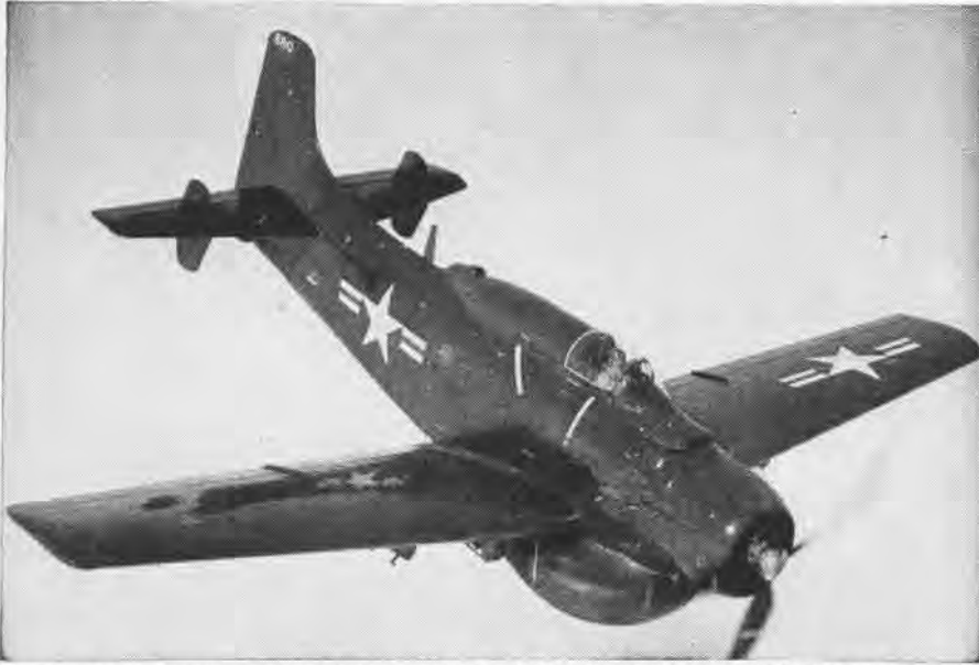
AD-4W, SEARCH PLANE OF THE DOUGLAS ANTISUB DUET, HAS THREE TAILS WHILE AD-4S HAS NOT
