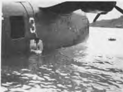
PATCH ON SIDE OF PBM RIGGED FROM A CHAIR
