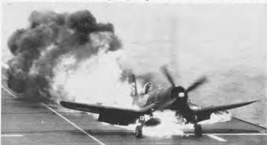
A LITTLE thing like a two-bit cap on a belly gas tank can be mighty important—especially if it comes off when the plane is making an arrested landing. Here is what happened to 1st Lt. Burcher V. L. Sheard of VMF-323 when he landed aboard the Sicily . There was just enough gas left in the tank to spray the hot exhaust stacks, resulting in the blossom of flame shown here. Needless to say, all tanks now are being emptied before coming aboard. Damage to the plane was slight and with new elevators it was in the air again in a few days
