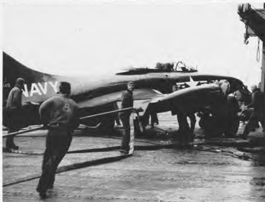
HERE IS EXAMPLE OF WHAT CAN HAPPEN TO AIRPLANE WHEN BARRIER IS LOWERED TOO SOON
