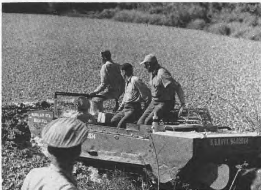
THE WEASEL operates on water as well as land and descends into a canal choked by water hyacinths; triphibious rescue facilities are necessary in marshy land of the Everglades
