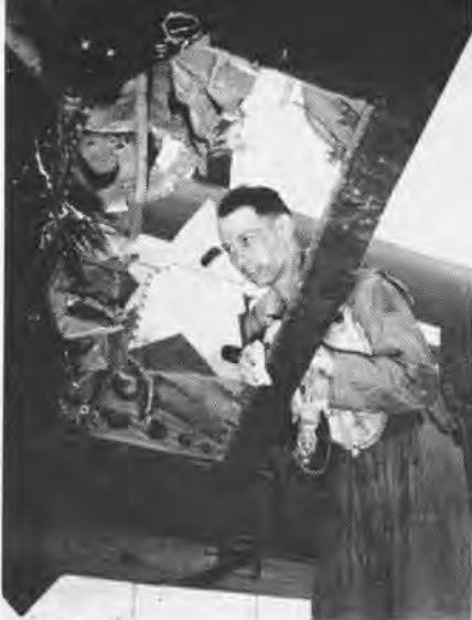
HIS FACE cut in combat, Cdr. Maulby of VA-35 inspects gaping AA hole in his flap
