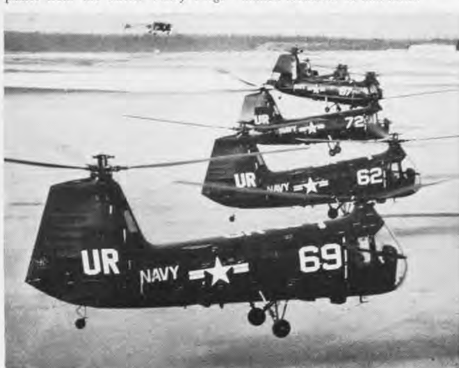
A BIT RAGGED as formation flying goes, perhaps, but still about the closest formation of helicopters ever photographed are these five HUP-1's hovering a few feet off the deck at NAS Lakehurst. Early models of the Piasecki HUP's had "elephant ear" supplementary vertical stabilizers on each side of the rudder but these were eliminated to cut down on plane's weight.
