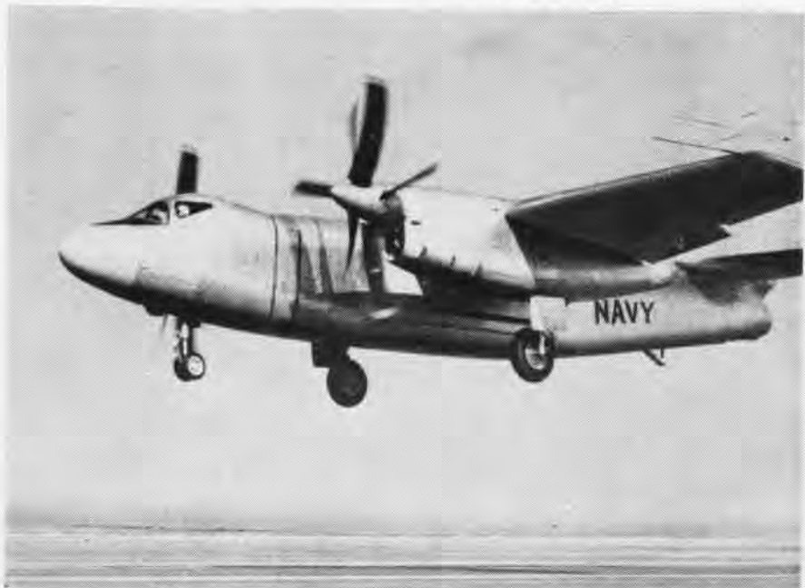
THE NAVY'S new XA2J-1 takes off from Los Angeles International Airport on its first flight. This carrier-based attack bomber, built by North American Aviation, is capable of speeds in excess of 400 miles an hour. Its maximum take-off gross weight exceeds 26 tons, thus making it the heaviest of the Navy's carrier planes. The XA2J-1 is powered by two Allison T-40 turboprop engines, turning six-bladed contra-rotating propellers. It carries 20mm armament and has a bomb load of 10,000 pounds.
