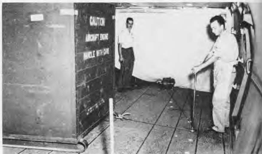
POGO STICK MAKES EASY TASK OF SLIDING LARGE CRATES ONTO AND INTO NAVY TRANSPORTS
