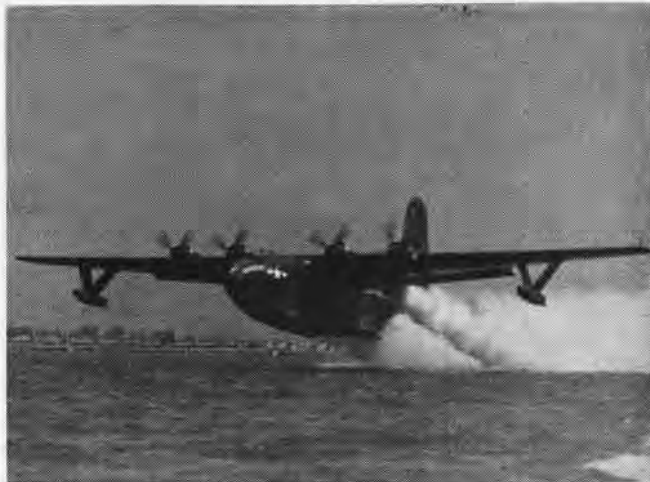
THE PHILIPPINE Mars is making a jet-assisted takeoff, a procedure used only when the sea is extremely smooth or extremely rough
