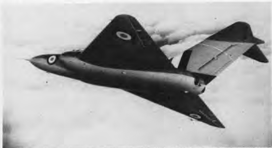
THE GLOSTER GA.5, A TWIN-JET, DELTA-WING PROTOTYPE AIRCRAFT IS BEING TESTED BY RAF
