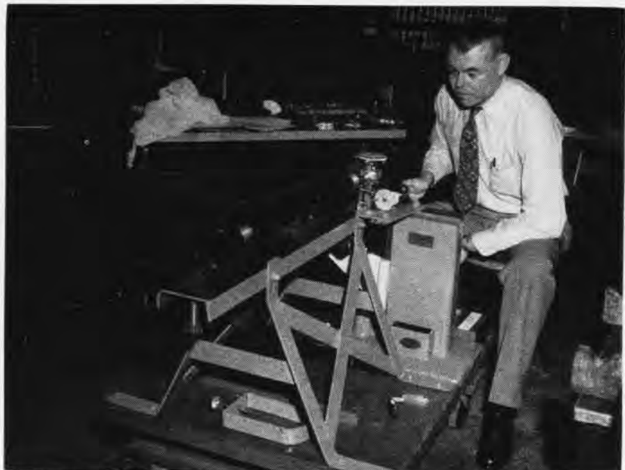
INSTRUMENT maker J. C. Weaver performs delicate job of measuring bore dimensions of 20mm gun barrel in shop of laboratory services division, Aviation Ordnance Dept., Dahlgren.
