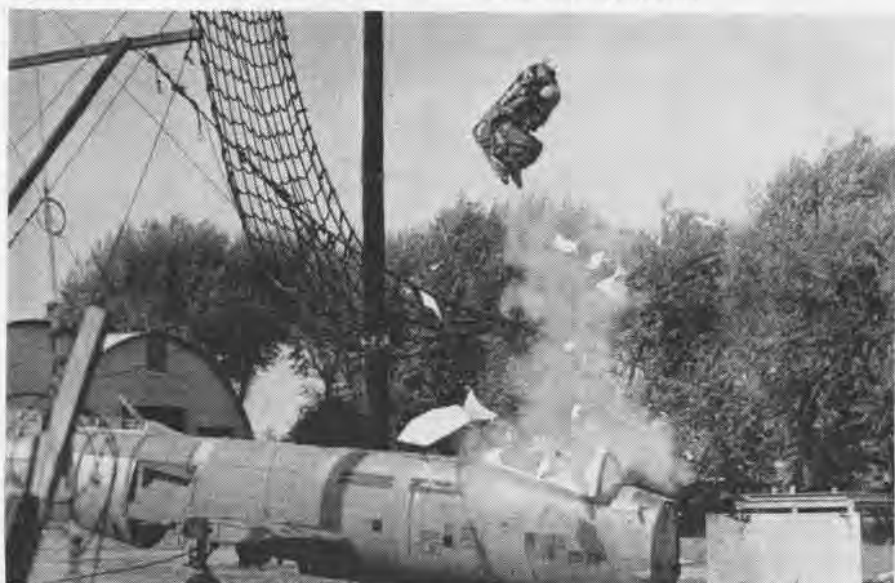
SOMETIMES jet pilots have found themselves unable to jettison their canopies so they can operate their ejection seats. Bureau of Aeronautics conducted tests at NAMC Philadelphia to see if it were feasible to fire the seat and pilot right through the plexiglas canopy. The picture above shows the dummy emerging through the shattered canopy, painted white.
