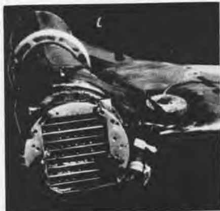
PULSE-JET ENGINE MOUNTED ON TIP OF ROTOR
