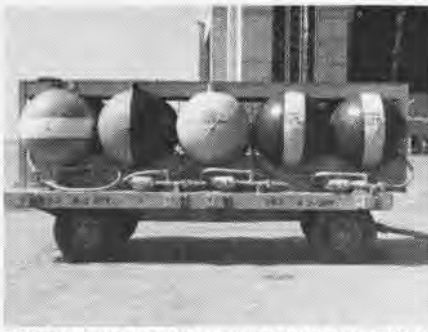
NON-SKID WOOD TOP USED AS WORK PLATFORM
