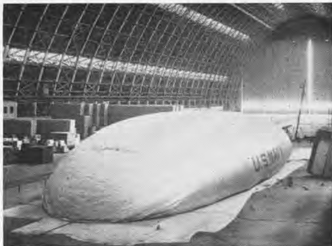
THE BIG bag begins to look like an airship as inflation begins under instruction of O&R personnel sent from Lakehurst
