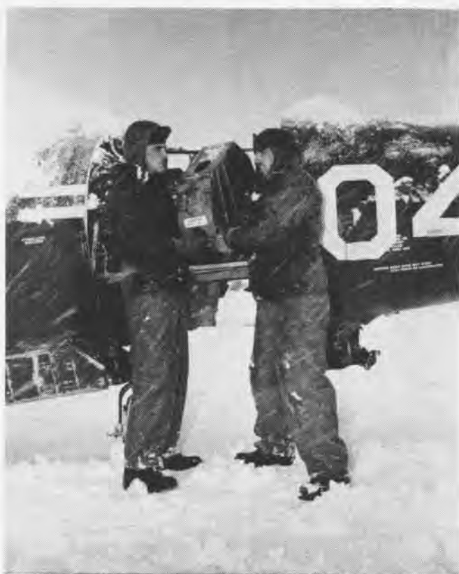
ORDNANCEMAN Cartwright, Machinist's Mate Stuvick remove ammo can from nose of F9F Panther under frigid conditions in Korea
