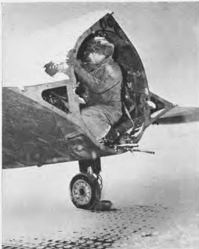
HUNDREDS of electrical, hydraulic, mechanical and fuel connections in "frosted" F9F are checked by Stevenson, aviation mech
