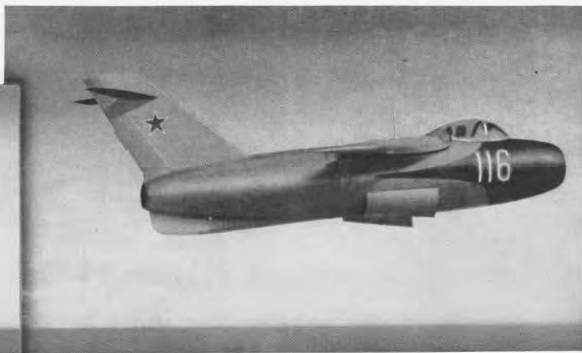
A newcomer in the Communist fold in "Mig Alley" of Korea is a high-wing jet, which may be this Lavochkin jet fighter. Because of its high, thin wing, landing gear apparently is housed in the fuselage, as shown in the series below. The tail fin is not quite so swept back as in the Mig-15 and a fin under the fuselage is a good recognition feature, as is the high wing. Photos courtesy British Joint Services Recognition Journal.
