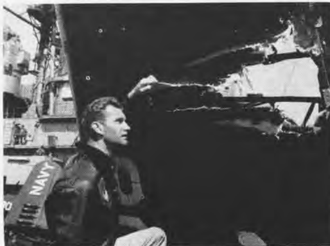
"GREAT BALLS of fire, it didn't look half that bad from the cockpit", says Lt. (jg) Rip Wilson as he views 37 mm hole in wing
