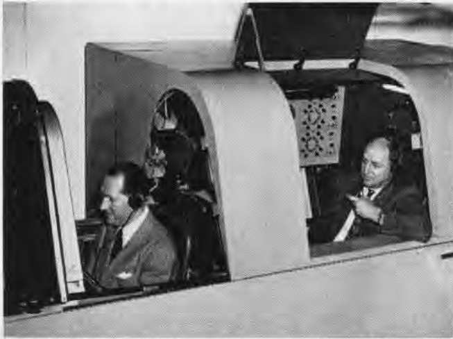
IN NEW SNJ trainer the instructor has a cockpit and dual controls; Link V. P. Williford plays student while Pres. Edwin Link instructs
