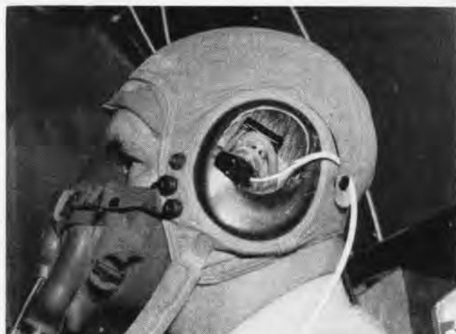
OXIMETER TELLS OXYGEN IN BLOOD BY LIGHTS SHINING THROUGH EAR
