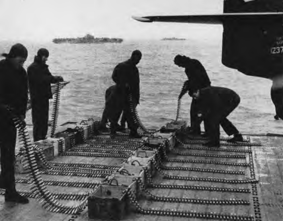
ESSEX ordnancemen check links, inspect 20 mm. ammo before rearming gun in Panthers
