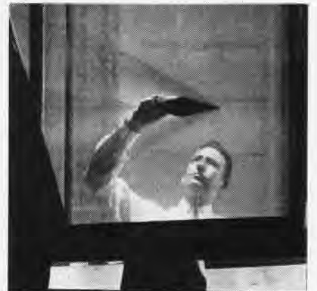
WATER FLOWS BY MODEL, MOCKS SHOCK WAVE
