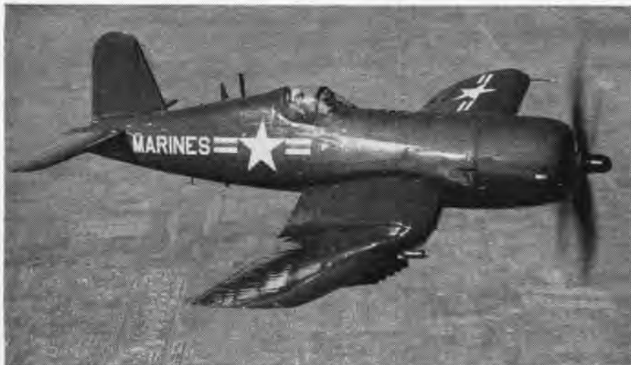
NEW VOUGHT CORSAIR, AU-1, ESPECIALLY DESIGNED FOR LOW ALTITUDE MISSIONS IN KOREA
