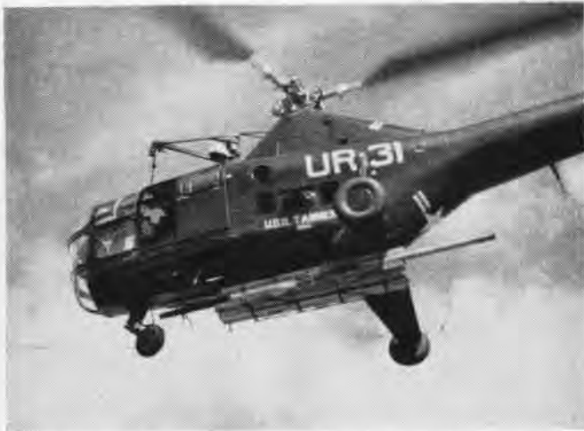
UNDER-FUSELAGE 'bomb rack' of Sikorsky helicopter was handy way to transport and drop lumber for mountain peak site work
