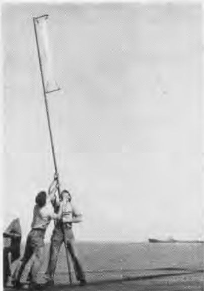
TRACKING flag aboard Maury tests rotor blade alignment of 'copter before hop
