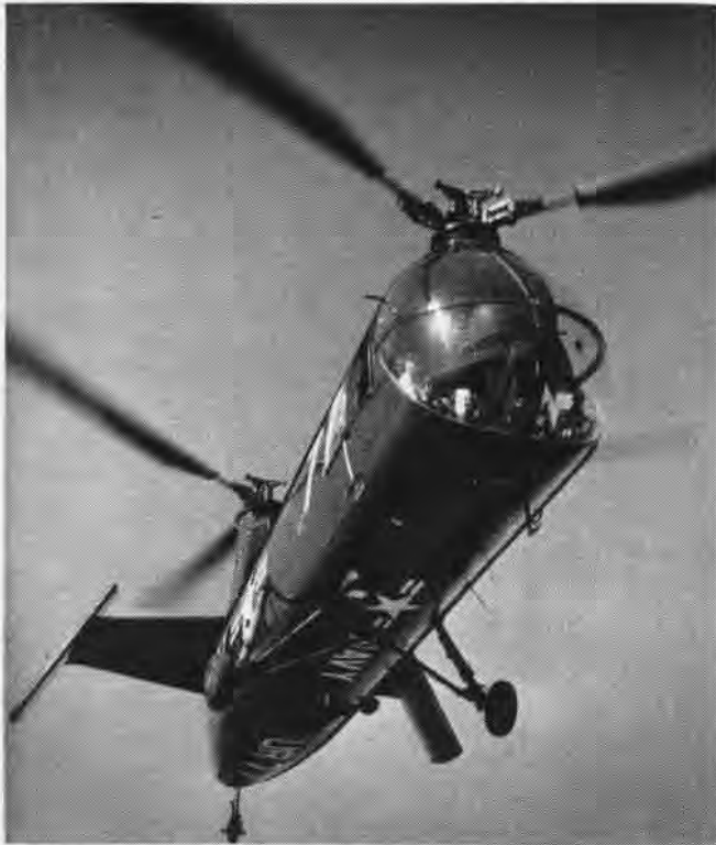
LATER model HUP-2's are minus extra tail stabilizers, but Gauthier preferred "wings" left on for stability in mountain gusts
