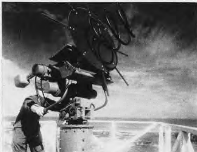
TELEMETERING radar installations like this at Patrick AFB will receive flight data from missiles all down the missile range
