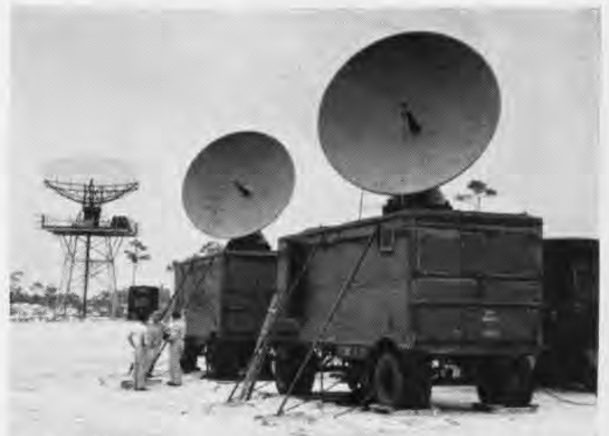
GIANT Air Force radars, SCR-584 in front and CPS-5 in rear, track the guided missiles as they fly along the island chain
