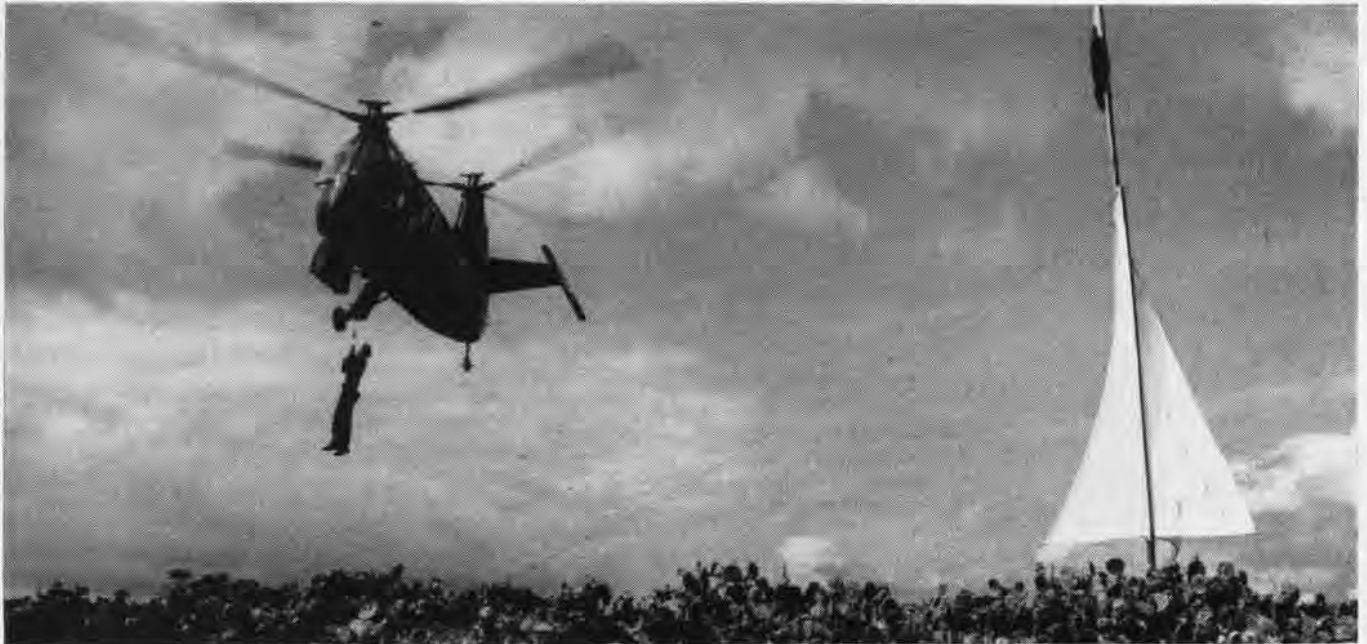
HYDROGRAPHIC survey man being lowered to center pole site from belly hatch of HUP-1 helicopter; in some areas, terrain pre-
