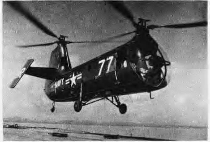
TAKING OFF from 45x60' flight platform on fantail of Tanner, HUP carries five men; low undercarriage hampers lumber carrying
