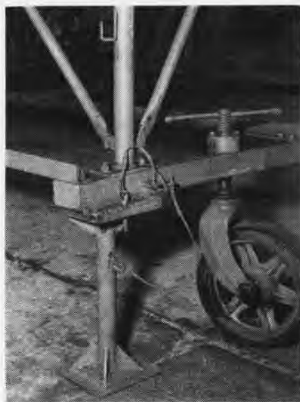
NEW STAND FOR WORK PLATFORM IS PORTABLE
