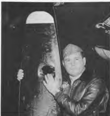
NO WONDER LCdr. DuTemple's prop made whistling shriek, with 37 mm hole in its blade
