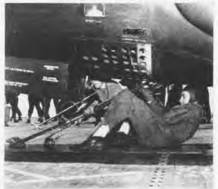
FAST WORK in close quarters as Donald Frye, AB3, adjusts catapult bridle on a Panther
