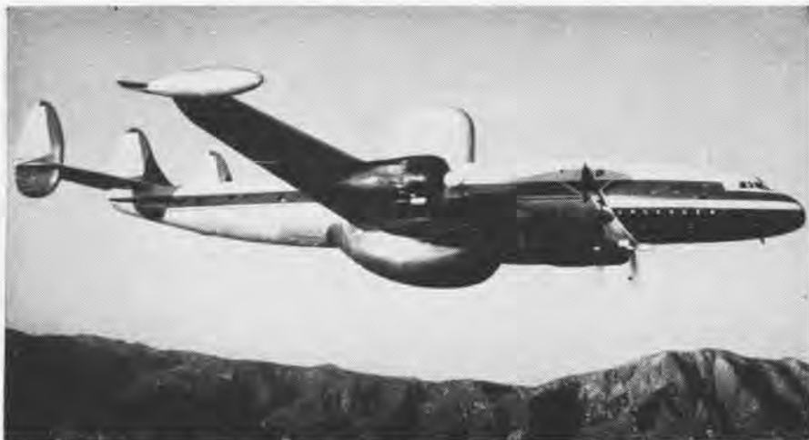
CONFIGURATION of the Navy's new high-altitude flying sentinel for radar work is revealed in this dramatic photo of the Lockheed Super Constellation equipped with finlike radar housing atop the fuselage and expanded radar nacelle below. Precise mission of the WV-2 is secret, but wingtip tanks indicate capacity for long range to do aerial radar scouting.
