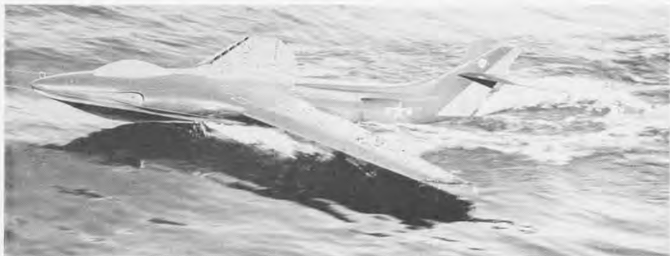
CONVAIR'S SKATE FIGHTER SEAPLANE MODEL 15 IS POWERED WITH TWO SIX-POUND PULSEJET ENGINES. IT HAS BEEN FLOWN A NUMBER OF TIMES
