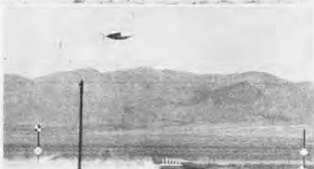
SUPERSONIC pilot escape capsule, designed by Douglas Aircraft Corp., was tested on aeroballistics track at Naval Ordnance Test Station
