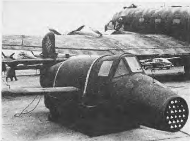
NOSE TUBE —German vertical-rising 578 mph rocket interceptor carried 24 rockets in its nose; airplane had no landing gear.
