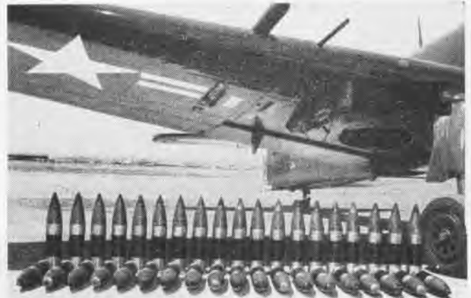
TUBES —Experimental tube in AD wing fired 38 5" spin-stabilized; note exhaust vent; fiery exhaust burned plane aileron.
