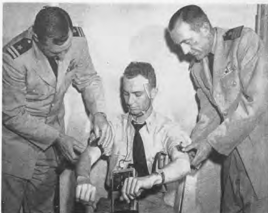
LT. HODGE (LEFT) AND CDR. BARR FASTEN TINY TRANSDUCERS ON BODY OF TEST PILOT MURRAY
