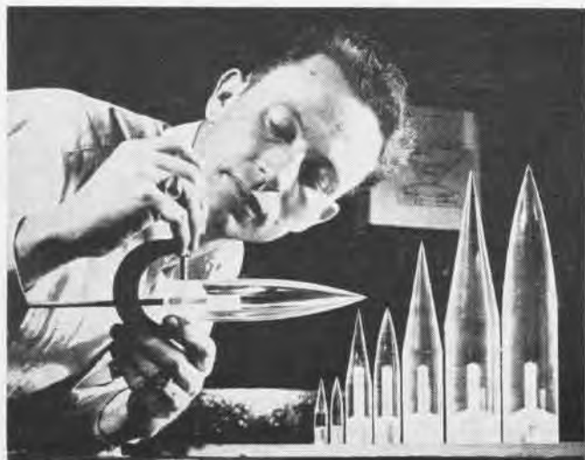
TECHNICIAN measures cones and streamlined bodies used in testing air flows at supersonic speeds in the gas dynamics laboratory.
