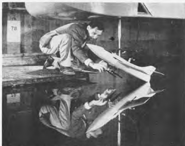
HYDRO-SKI model is fixed under carriage carrying recording instruments and movie cameras for simulated landings and takeoffs.
