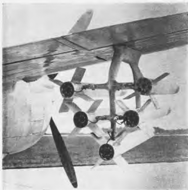
XMAS TREE —One of oddest launchers for rockets was this early Air Force development for fighters, carrying five Holy Moses.
