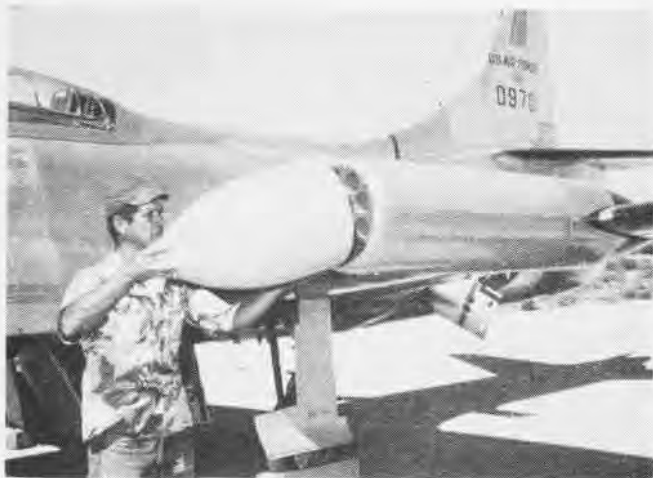
PODS —Air Force has mounted leading edge wing pods on F-94C with 12 2.75" rockets, augmenting the 24 in Starfire nose ring.
