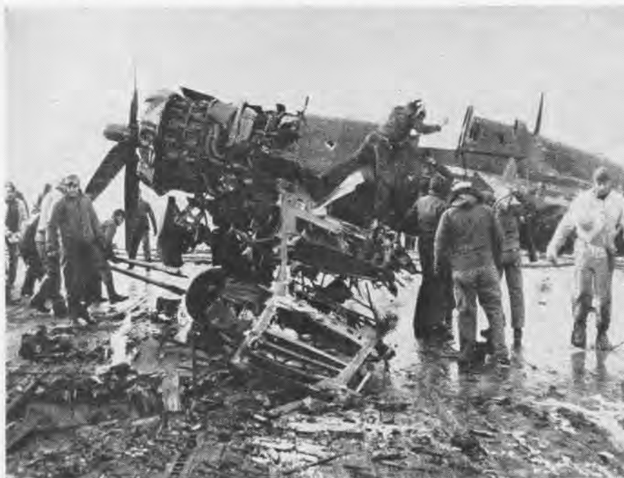
CLEAN-UP and salvage operations begin on the Oriskany after bomb explosion on the flight deck when Corsair dropped its hung bomb. The destruction of the F4U is evident in this picture taken after the rescue of the plane's pilot, Lt. Edwin Kummer, by Richard Donovan. Note ragged hole in the flight deck in the lower left portion of the picture. At right, leaving the plane, is Michael Yox who assisted Donovan
