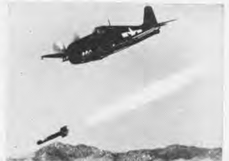
LANYARD — Tiny Tim rocket drops 16' below fuselage of F6F, then a lanyard fires it.
