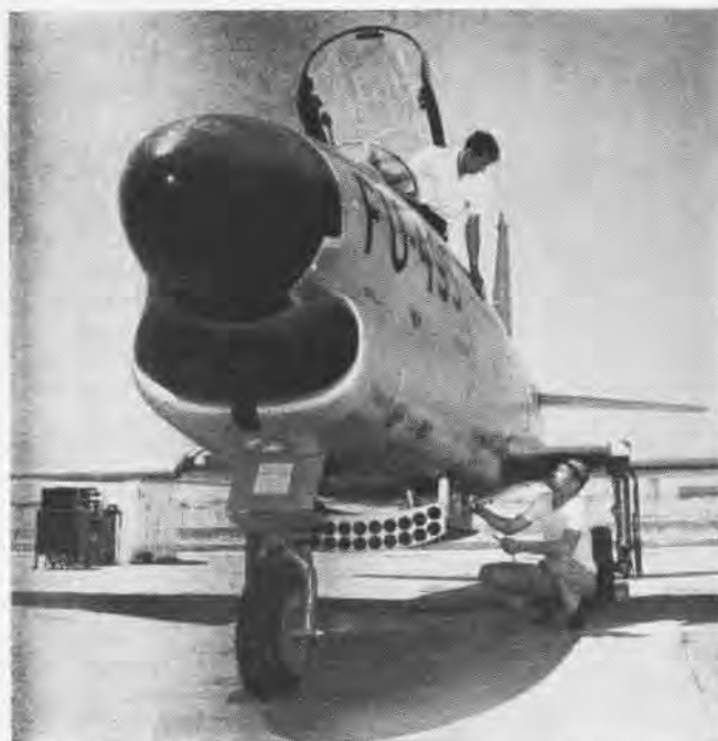
BELLY POD —Newest system of firing rockets used by the AF is the retractable 24-rocket pod slung under F-86D jet fuselage.
