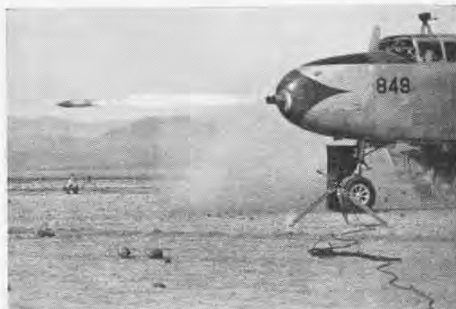
NOSE TUBE —Navy tried mounting launcher tubes in nose of PBJ and firing 5" spin-stabilized rockets; idea never worked out.
