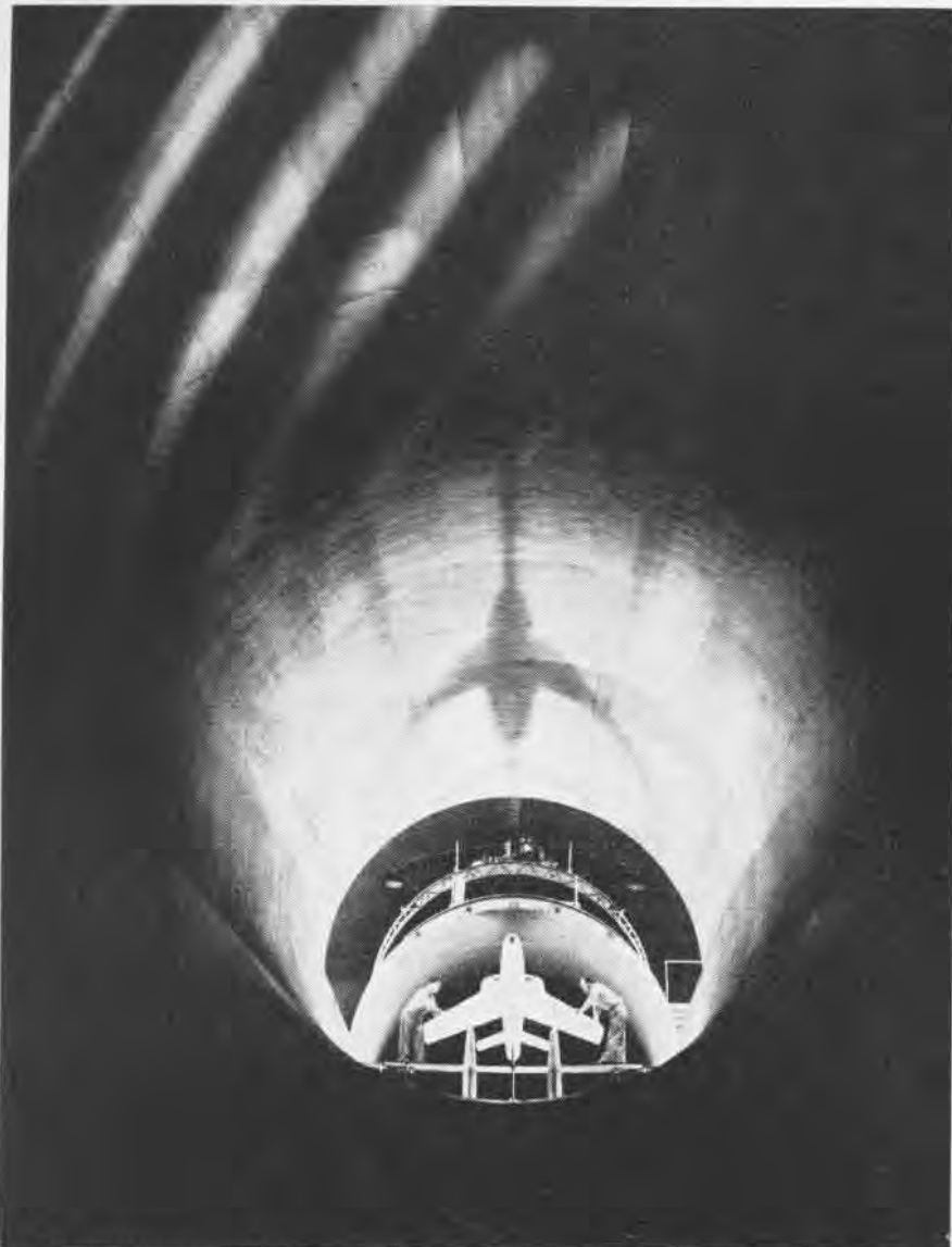
DRAMATIC NACA photo catches engineers at work on model mounted in Langley Aeronautical Laboratory's 19-foot pressure tunnel tests in which dense compressed air will be used.
