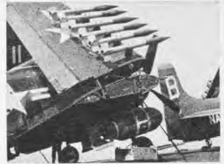
PYLON —Zero-length fixed launcher on Navy AD hold 6" Ram rockets with shaped charges.
