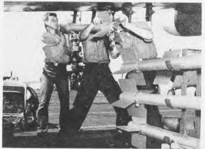
ZERO LENGTH —Two stub rocket pylons replaced heavy launching rails on Navy planes; Sangamon's men were loading 3.5" rockets.
