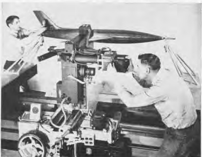
MACHINE measures key points of supersonic model destined to fly with rocket-power at NACA's Wallops Island, Virginia station.
