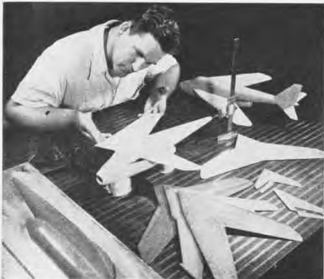
MODEL MAKER fixes wing to X-5 research plane. Varying sweep wings of reinforced plastic are used in testing model's stability.
