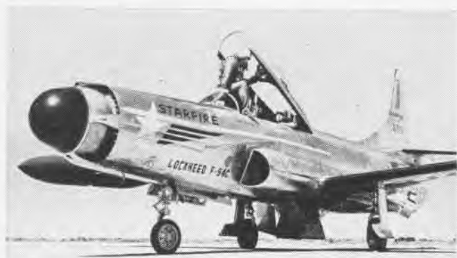
NOSE RING —The Lockheed Starfire carries 24 rockets around its nose; exhaust from rocket is contained within sealed-end tube.
