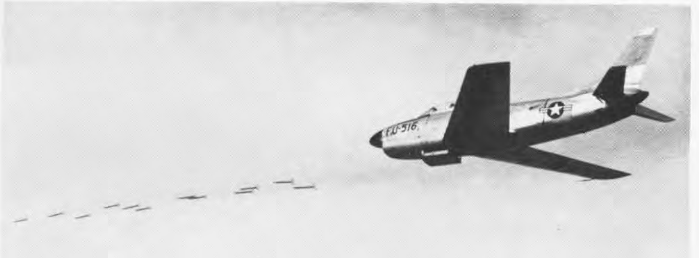
PODS —Latest Air Force idea for carrying Mighty Mouse rockets on F-86D is retractable 24-rocket belly mount
