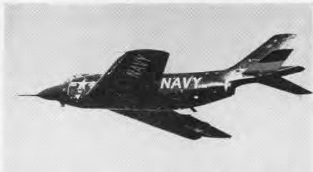
THE F3H-1N DEMON IN FLIGHT SHOWS SWEEPBACK WINGS AND TAIL
