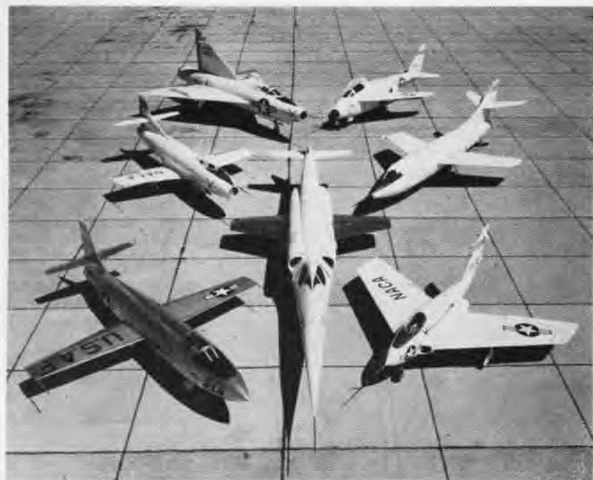
THIS CLUSTER of aircraft represents thousands of dollars in experimental research. Collected around the Douglas X-3 jet-powered aircraft designed for sustained flight at extremely high speeds are the Bell X1-A, the Navy's jet-powered Douglas D-558, the Convair XF-92, the Bell X-5, the Navy's rocket-powered D-558, the Northrup X-4,
