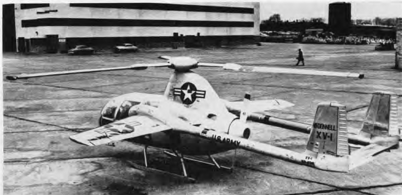
STUBBY-WINGED XV-1 CONVERTIPLANE EMPLOYS PRESSURE JET UNITS ON EACH ROTOR BLADE TIP AND A RECIPROCATING PUSHER-TYPE ENGINE
