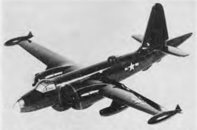
P2V-7 IS IDENTIFIED BY DOUBLE-BUBBLE CANOPY, JET POD ENGINES
