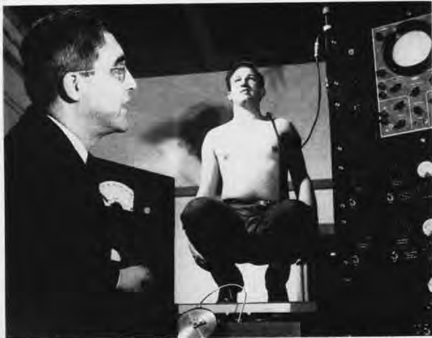
LCDR. D. E. GOLDMAN CHECKS GRAPH AS H. L. BRAUN SQUATS ON SPECIAL VIBRATOR BASE
