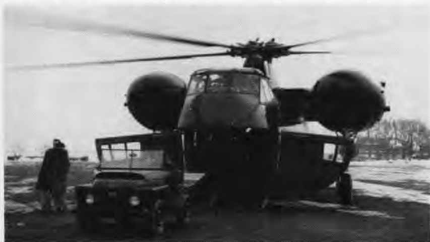
A MARINE "Mighty Mite" rolls down the yawing bow ramp of this new Marine assault helicopter. Dubbed the HR2S by the Marine Corps, this new machine is powered by two R-2800 aircraft engines which give it a speed in excess of 159 miles per hour and the capacity to lift three "Mighty Mites" or 26 fully equipped troops.
