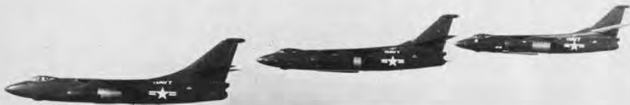
WARRIORS of the sky, three newly-christened A3D Skywarriors, are shown in an unusual picture. Early experimental and production models of any aircraft are rarely test flown simultaneously and it's even more unusual when they are together in formation. The long-range, swept-wing, twin-jet bomber is now in production at the Douglas Aircraft Company, El Segundo.
