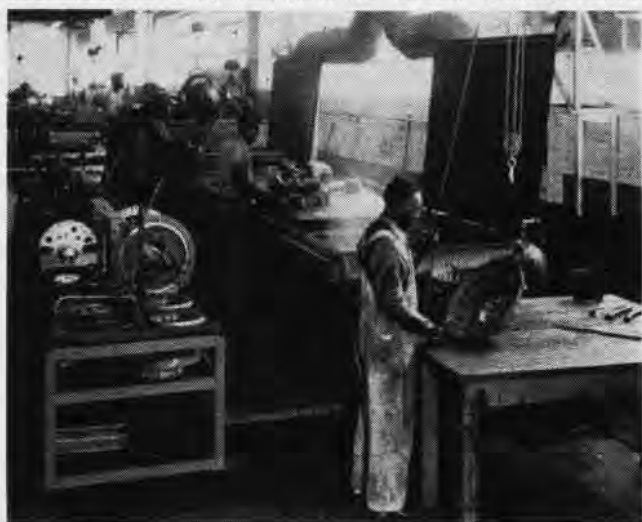
DISMANTLED parts are sent to the engine cleaning shop for solvent cleaning, grit or vapor blasting, buffing, polishing.
