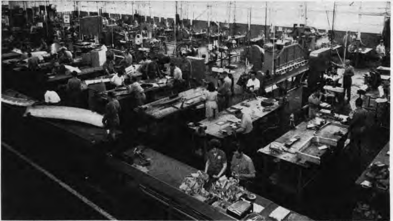
METAL SHOPS MANUFACTURE JIGS, FIXTURES, AND STEEL AND ALUMINUM PARTS USED IN OVERHAULING, MODIFYING OR REPAIRING PLANES
