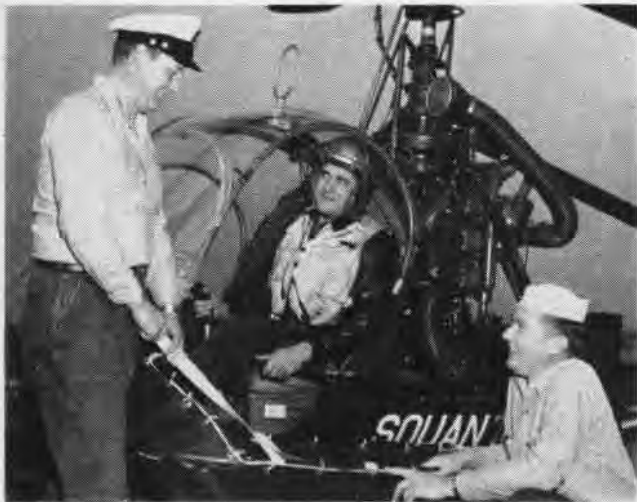
LESLIE McCullock, ALC, and James Swanson, AL2, place the improvised stretcher carrier on HTE-2 flown by LCdr. Barufaldi.
