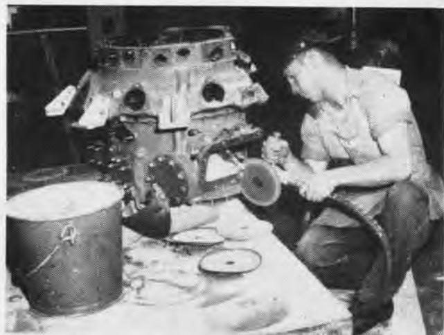
PART of first steps in preparing a cut-away is shown as D. B. Craddock, ADAN, touches up cuts on piece of engine cut-away.
