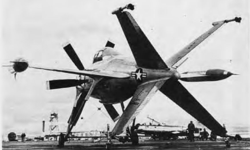
LOCKHEED'S XFV-1 vertical take-off fighter plane is shown in a "four-point" attitude as the plane rests on auxiliary landing gear during special test operations.
