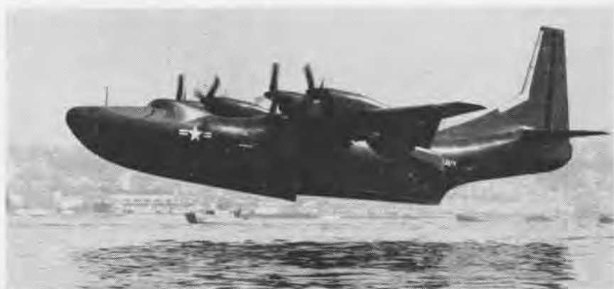
MORE THAN 22,000 hp take the first turboprop seaplane, the R3Y Tradewind, off San Diego Bay for its maiden flight. The 80-ton high-speed transport took off in less than 30 seconds and remained in the air during a shakedown test program for more than two hours. The test pilot said, "This seaplane is the best I've ever handled."
