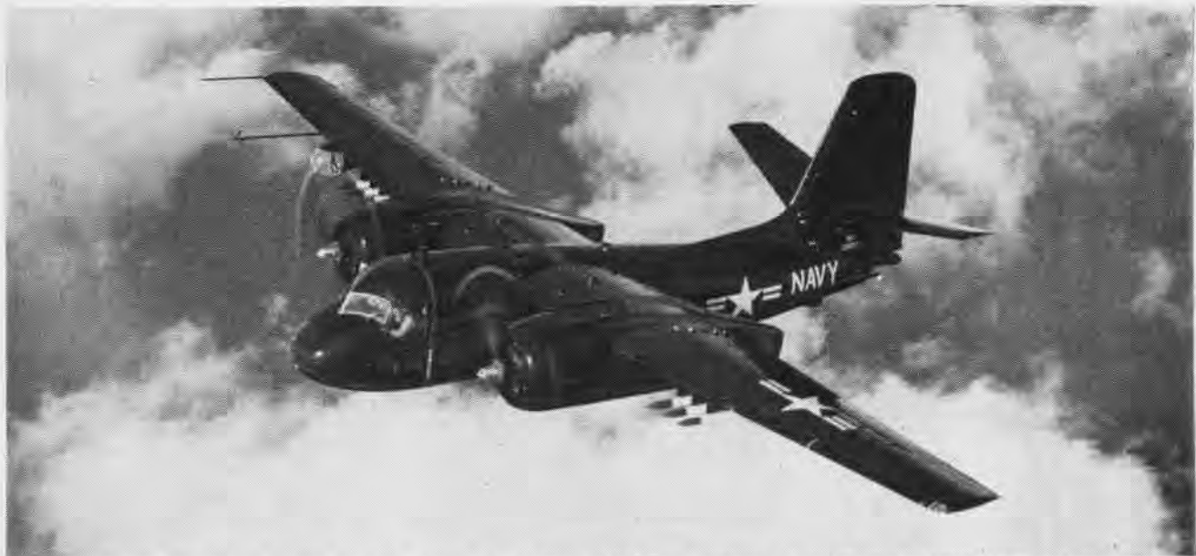
FULLY ARMED, THE S2F CARRIES EITHER ROCKETS, BOMBS OR DEPTH CHARGES AND INTERNAL HOMING AERIAL TORPEDOES. SHE CRUISES AT 130K
