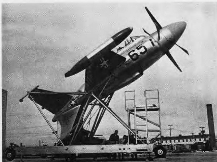
THE PROBLEM of easier maintenance was encountered by Lockheed designers on the XFV-1. This is their vehicle for transporting, raising and lowering their plane.
