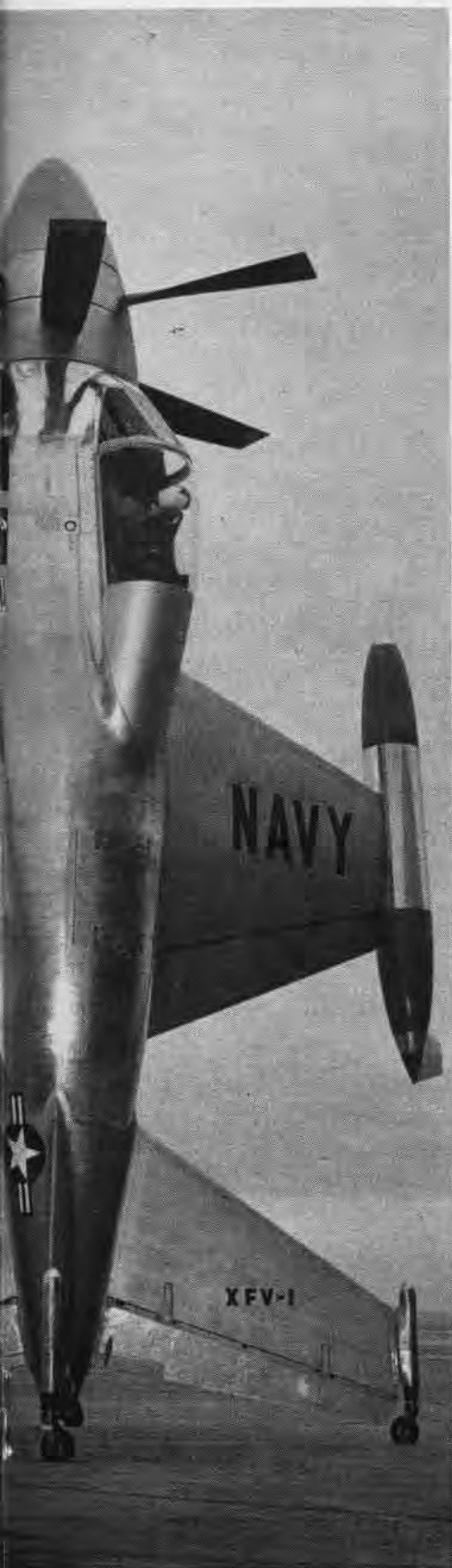
LOCKHEED'S XFV-1 vertical take-off fighter plane is shown in a "four-point" attitude as the plane rests on auxiliary landing gear during special test operations.
