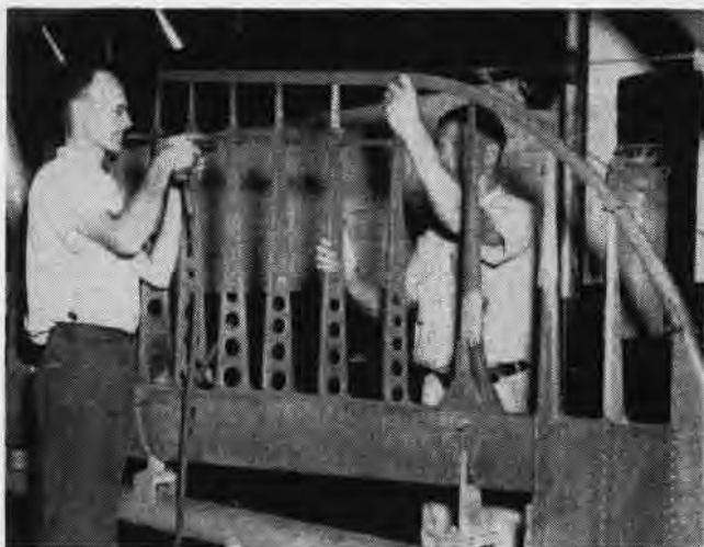
SMALL surface repair shops examine, repair, overhaul and modify small detachable metal surfaces such as rudders, ailerons.
