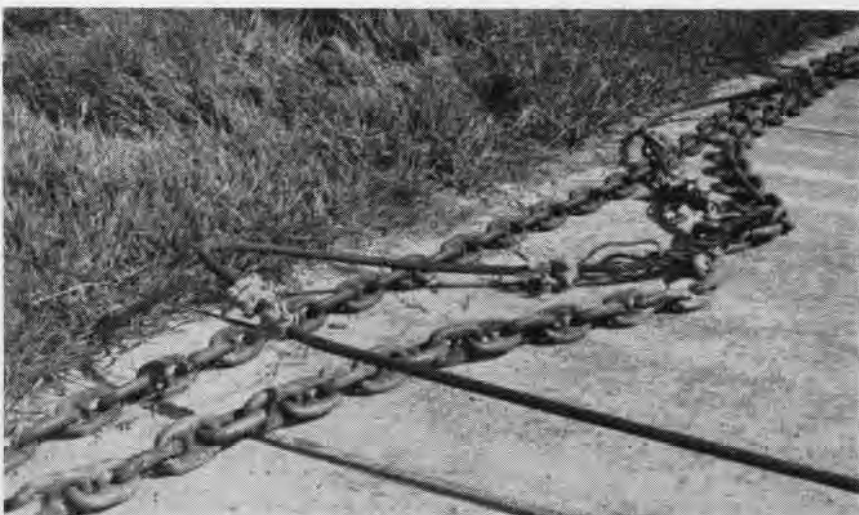
ANCHOR CHAIN produces the proper mass and surface friction characteristics to arrest a plane in a reasonable distance. Linkage with pendant is shown here.
