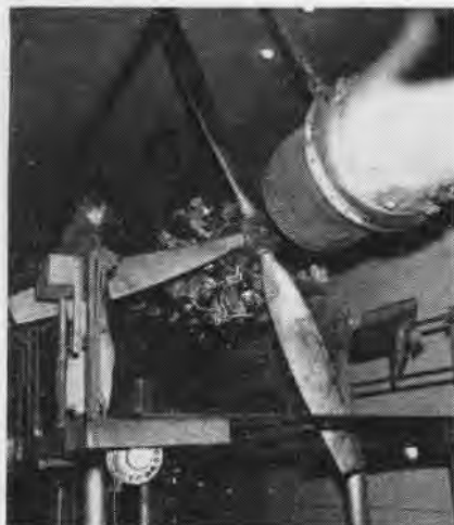
IN ENGINE test cells, assembled engines are run up to test for any malfunction.
