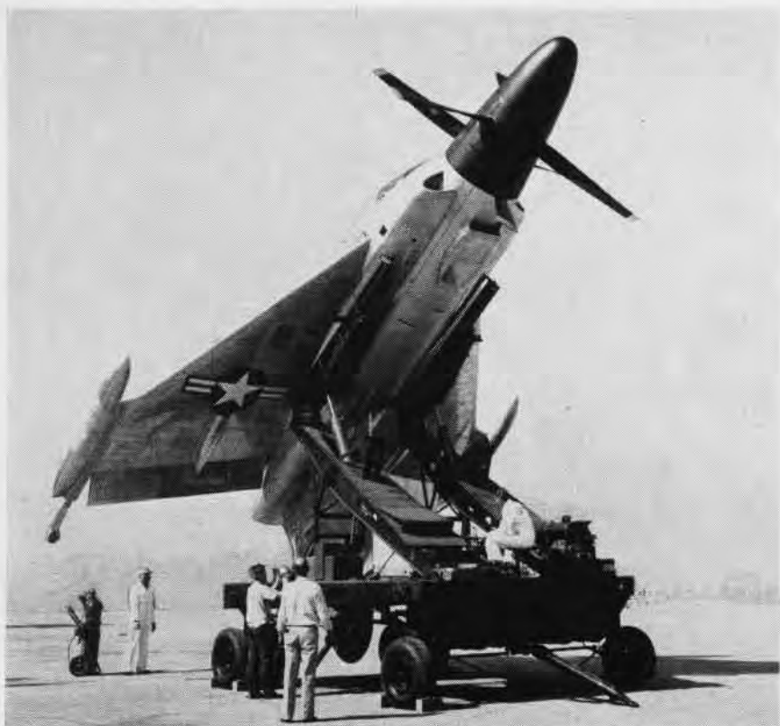
A SPECIAL mobile vehicle for transporting and raising and lowering the XFY-1 permits the plane to be tilted into various positions, making its maintenance easier.
