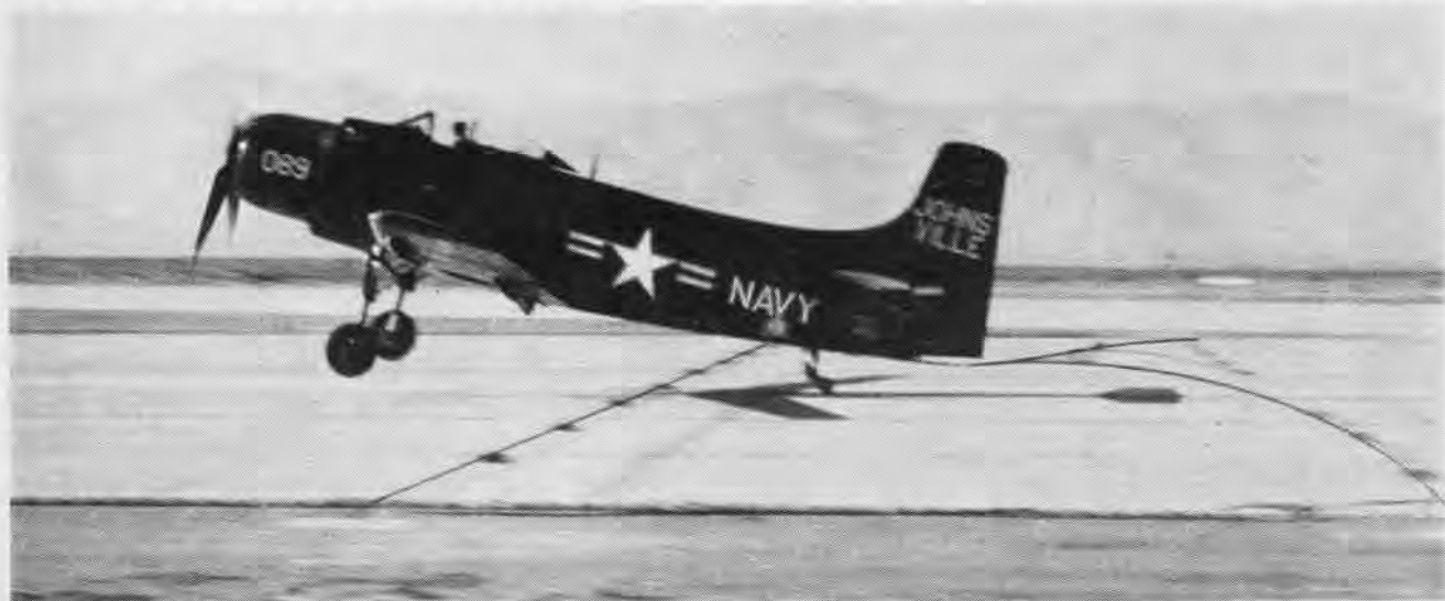
SKYRAIDER catches the wire of emergency aircraft arresting gear rigged across the runway. This flight deck principle has been applied to airfield use at about 35 naval and Marine stations and is expected to save between 200-300 planes a year.
