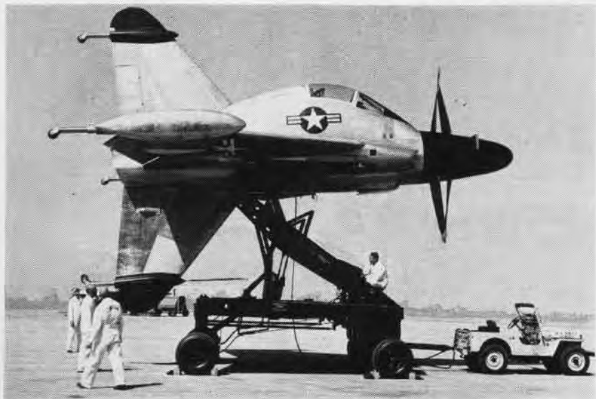
THE NAVY'S Convair XFY-1 vertical take-off fighter plane is shown in a horizontal position as the plane will appear in straight and level flight when it is airborne.
