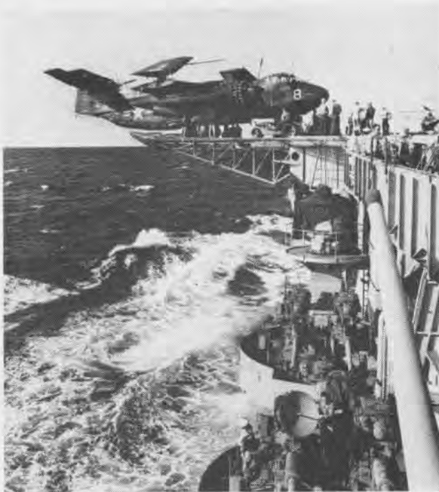
PERCHED on carrier's deck-edge elevator, A1 is ready to be taken below. Vertical stabilizer folds to clear the hangar deck overhead.
