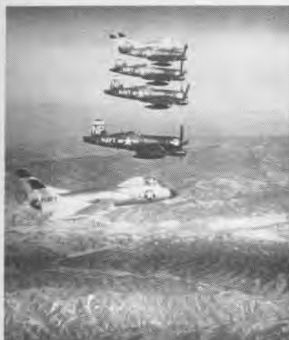
TWO F4U-3's flank the last four of VC-3's famed F4U-5N Corsairs as the old standby is readied for pasturing. The F4U-5N was used as a night 'heckler' in the Korean War.
