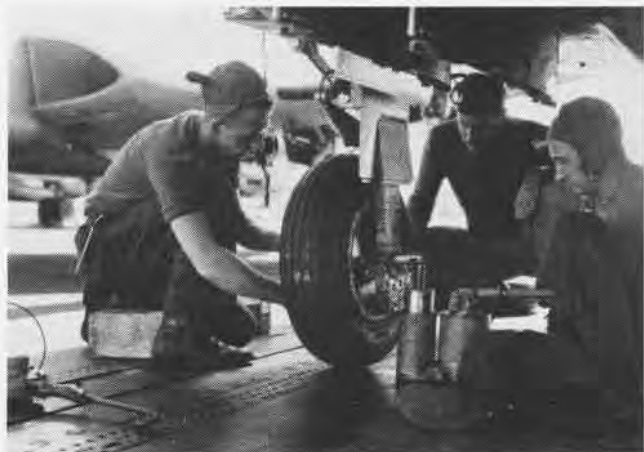
UNDER the fuselage of an F2H-4 aboard the USS Midway , VX-3 members, W. B. Baker, G. B. McNulty, and Joseph E. Thudcau, change a tire.
