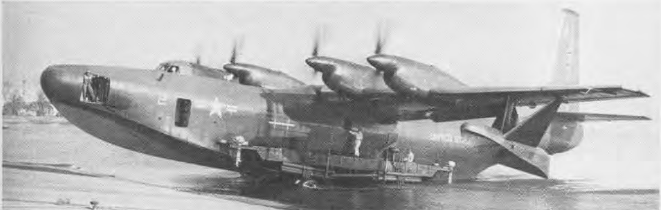
CRADLE FOR BEACHING OR LAUNCHING HAS FOUR PROPELLING 25-HP OUTBOARD ENGINES FOR INDEPENDENT WATER MANEUVERING
