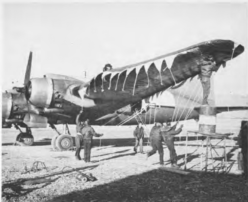
SPECIAL wing covers being positioned into place against the high arctic wind were a part of the winterizing given the B5D's in preparation for the polar weather. Made from experimental plastic cloth, the covers prevented formation of ice while the airplanes were on the ground.
