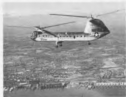
LARGEST of tandem-rotored helicopters—the US Air Force's YH-16 Transporter—made its first altitude flight when the 42-place, 15-ton aircraft was flown at speeds exceeding 130 mph at altitudes between 3,000 and 4,000.
