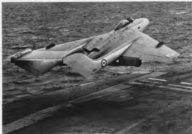
POWER IS displayed as the DH 110 is catapulted. Originally designed for shore bases, it is now an all-weather carrier fighter.
