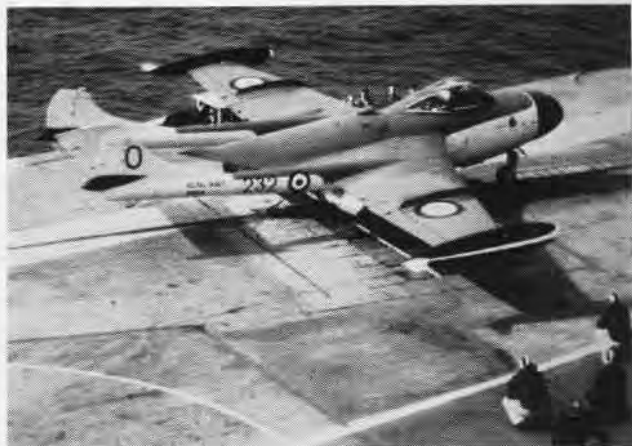
A SEA VENOM is set and ready to go on the steam catapult of HMS Ark Royal. This two-seater night fighter is powered by a Ghost engine.
