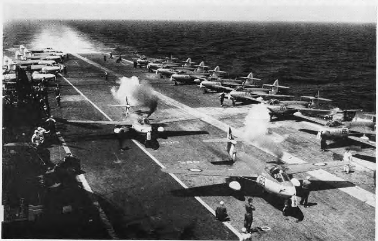
BUILT BY Hawker, Ltd., and Armstrong Whitworth, these Sea Hawk day interceptors on board the Eagle may be compared to our Panthers. This fighter is powered by a single Rolls-Royce Avon and was first flown 31 August 1948. Here Sea Hawks are made ready for take-off.
