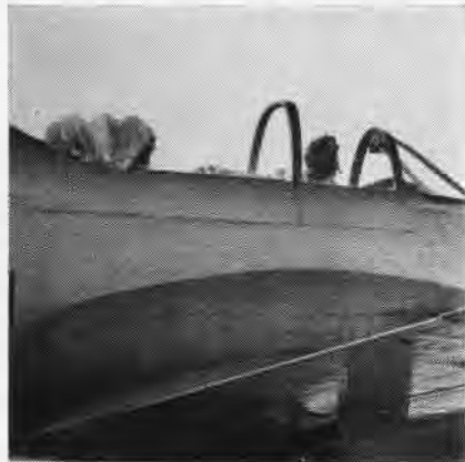
UNDER THE HOOD in the back cockpit, the student does the flying by use of instruments.
