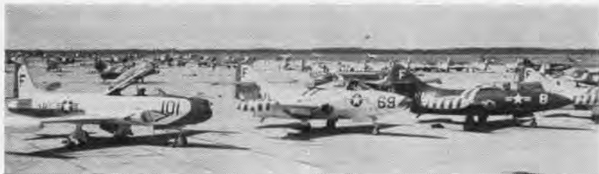
THREE F9F'S at ATU-206 Pensacola display old and new paint jobs. The all-blue design of Panther 8 (far right) dating from WW II, was superseded last year by combat gull gray and high gloss white, exhibited by Panther 69. At left, TV-2 #101 demonstrates the new international orange and high gloss white with which all training jets will be painted. The striking color scheme provides maximum "see ability" necessary in crowded training areas.
