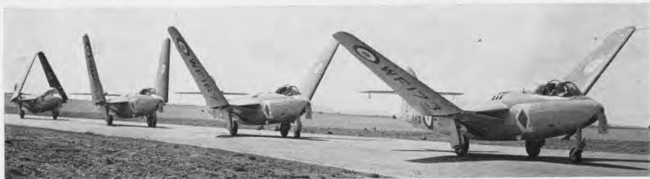
AT AN UNDESIGNATED naval air station, these Sea Hawks taxi out, preparatory to a training exercise. These fighter aircraft feature a folding wing for stowage aboard carriers. At the Farnborough 1954 show, one Sea Hawk had rockets installed for jet-assisted take-off.
