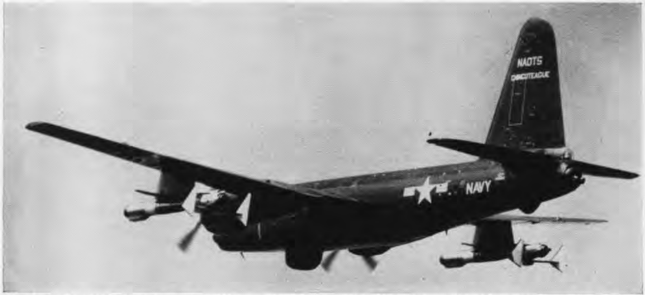
NAVY'S AIR-TO-SURFACE GUIDED MISSILE PETREL IS SHOWN SUSPENDED FROM THE WINGS OF A LOCKHEED P2V NEPTUNE
