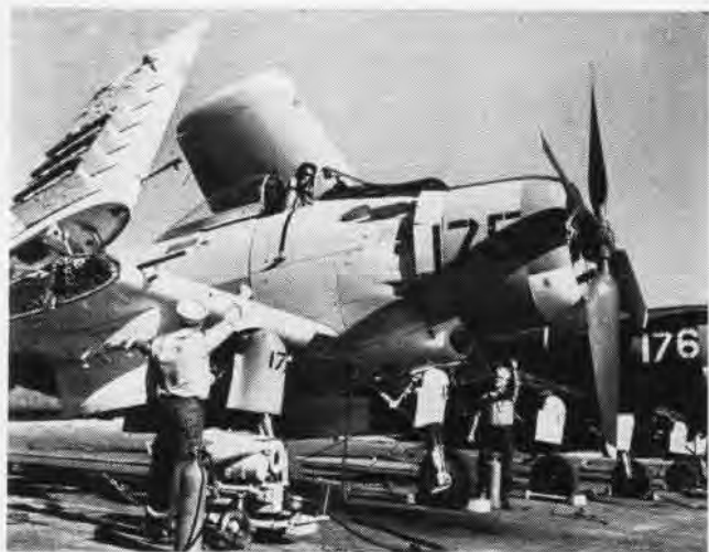
'THUMBS UP' gives line crewmen signal that pilot is ready to start engine. C. E. Brittin and R. L. Hotman, AA's, man APU and fire bottles.
