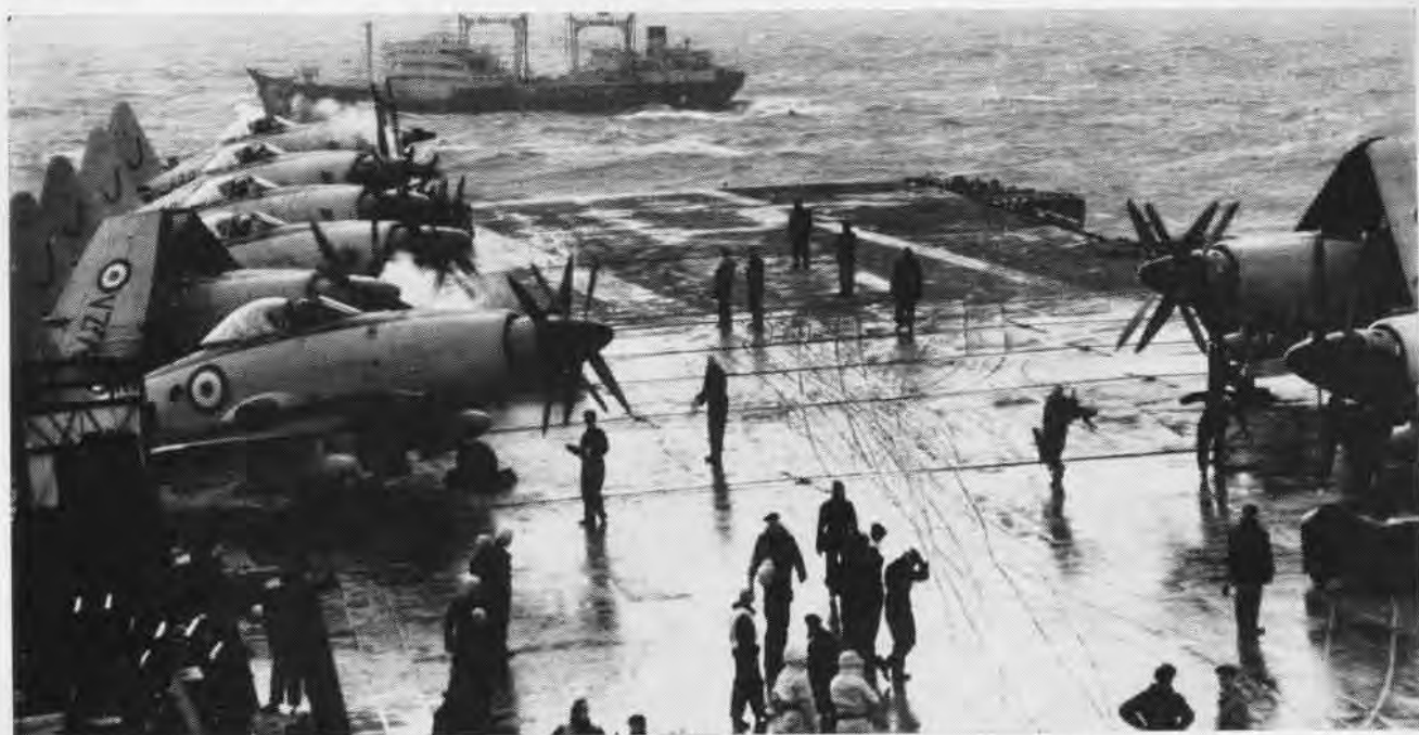
THESE TURBOPROP Wyverns, Navy antisubmarine and strike fighters, are starting up on HMS Eagle during rough weather on a NATO exercise. The Wyverns are powered by single Armstrong-Siddeley Pythons. First flight of the aircraft was made during March of 1949.
