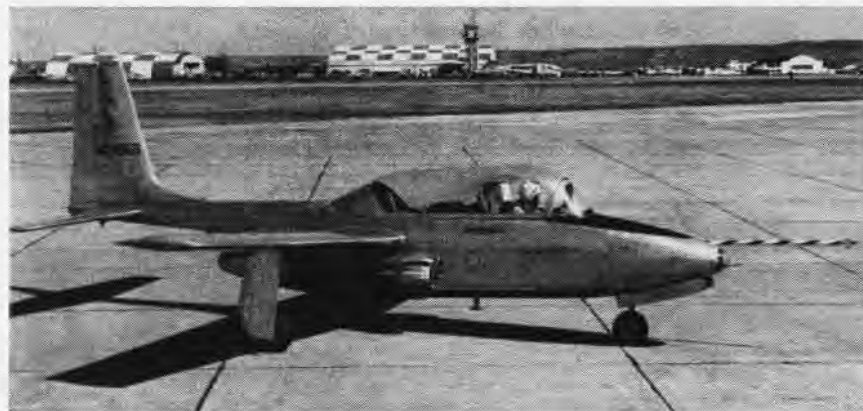
TEMCO'S NEW trainer, the Model 51, on the strip at Dallas, Texas, is awaiting take-off. Powered by a Continental YJ-69-T-9 turbo jet engine which supplies 920 pounds thrust at sea level, the trainer has an overall length of 30.6 ft., and a height of 10.82 ft. The wing area is 150 square feet; normal gross weight is 4137 pounds. Normal fuel load is 119 gallons.
