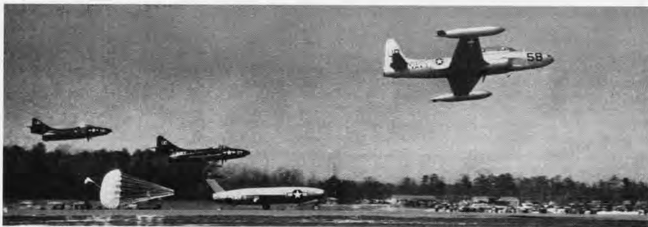
A REGULUS MISSILE IS LANDED AFTER TEST AT NAOTS CHINCOTEAGUE WITH DRAG PARACHUTE BRAKING THE WEAPON TO SAFE ROLL-OUT
