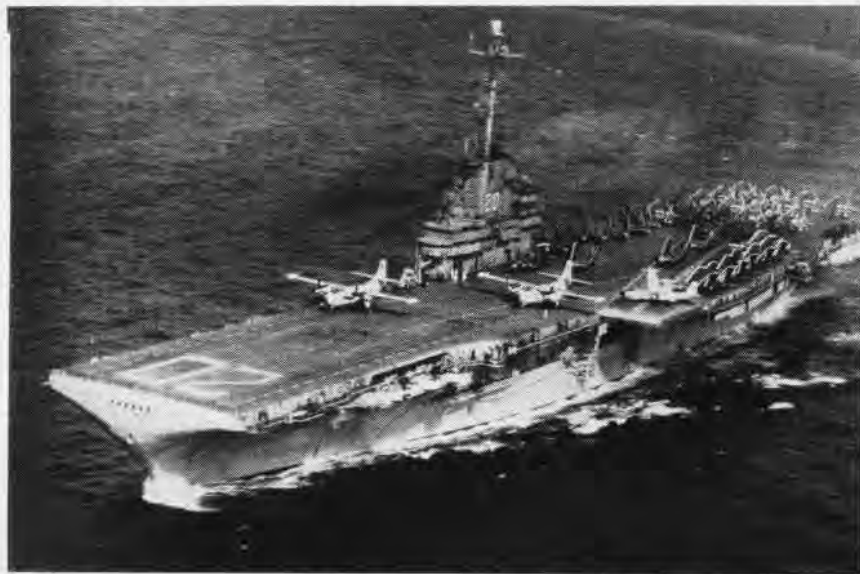
TWO AJ-2 SAVAGES from VC-62's Detachment of ATG-201 set on the catapults ready for immediate launch as the aft end of the flight deck is arrayed with Panthers, Banshees, Cougars, Skyraiders.
