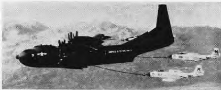
THE NAVY'S R3Y-2 Tradewind is shown in its latest role as an aerial tanker as three thirsty F2H-3 Banshees from VF-23 hook on to the drogues for inflight refueling. The big Tradewind , powered by four T-40 turboprop engines, was originally built as an assault seaplane transport.
