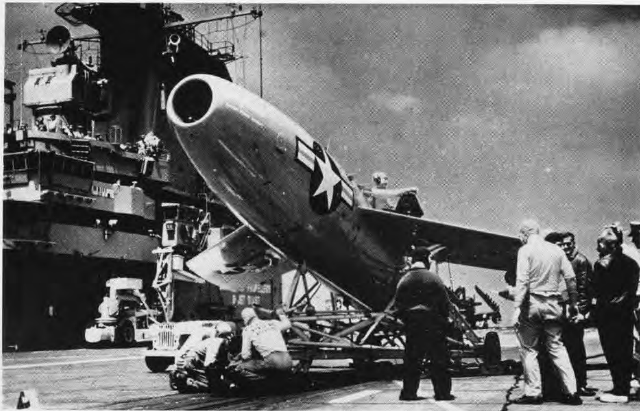
REGULUS DESIGNED FOR LAUNCHING FROM SUBMARINES, SURFACE SHIPS AND SHORE BASES IS A TURBOJET POWERED MISSILE
