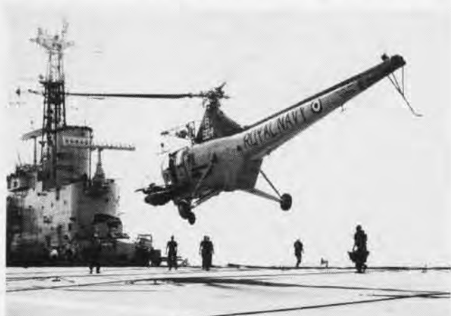
DRAGONFLY , a search and rescue helicopter, comes on board a carrier. Note its scoop net which was designed to rescue injured pilots.
