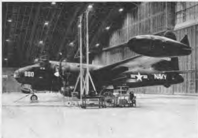
INSIDE SHIELDED HANGAR, A P2V-5 UNDERGOES A NOISE TEST
