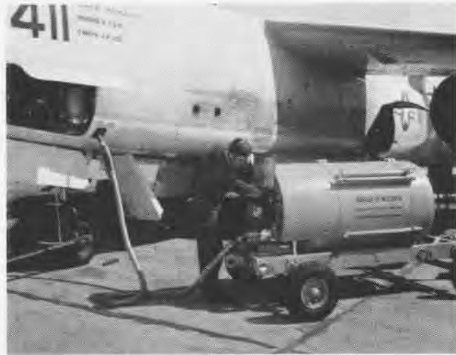
A3D IS BEING serviced with liquid oxygen from a standard, shore-based, 50 gallon transfer trailer. Plane has a ten-liter flask.
