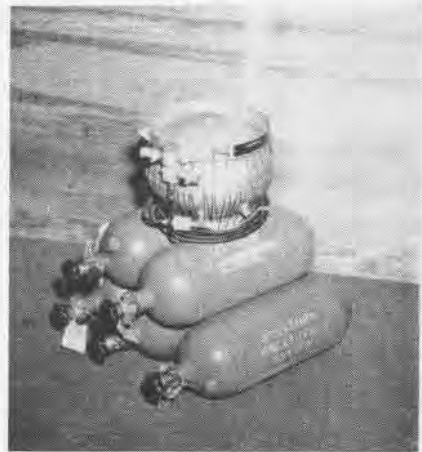
FIVE-LITER converter, fully charged, is about equal to five 514 cu. in.-gaseous cylinders.
