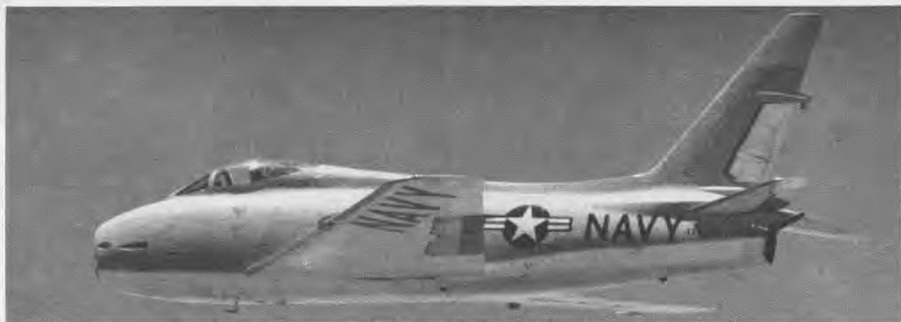
FJ-4 FEATURES DESIGN ELIMINATING WING FUEL CELLS. FUEL IS STORED IN SPACE BETWEEN UPPER AND LOWER WING SKINS
