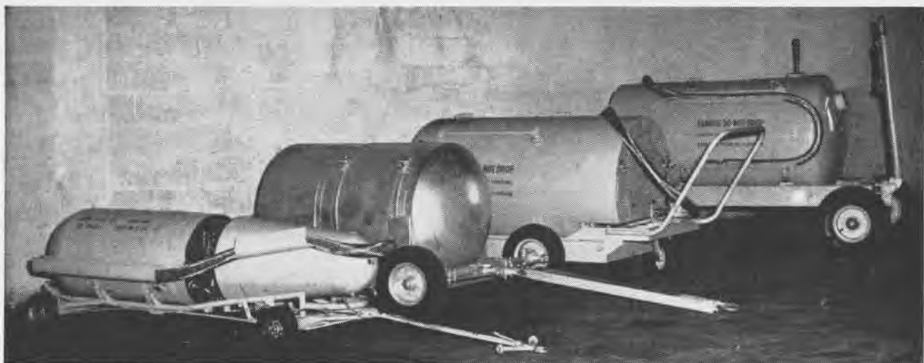
LIQUID OXYGEN transfer trailers under evaluation are lined up for inspection. First is a 15-gallon shipboard unit, followed by a 30-gallon trailer for either ship or shore base. Next are the 50-gallon shipboard and the standard 50-gallon shore-based transfer units.
