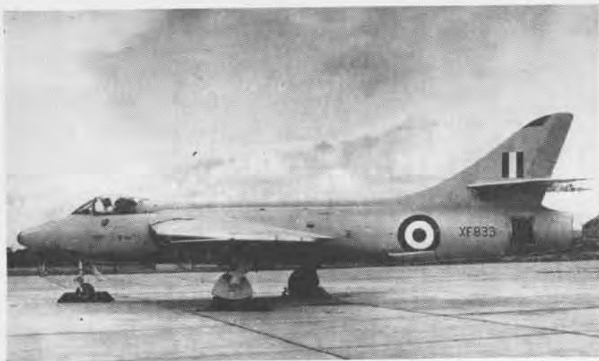
ONE OF THE highlights of the show at Farnborough was the Rolls-Royce reverse thrust unit installed in a Hawker Hunter Mk. 6 which makes it possible to reduce the ground runs.
