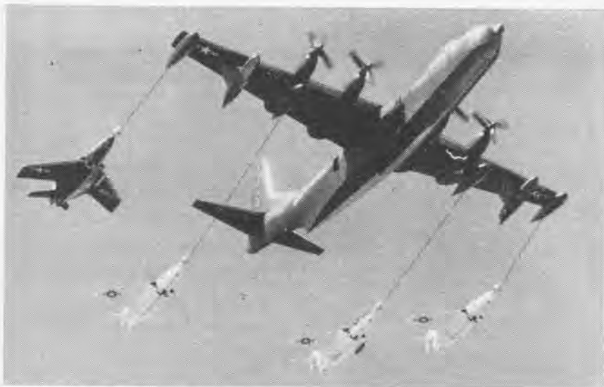
BREAD-WINNER for this family of four Congress is a Convair R3Y-2 Tradewind. This is the first instance of multiple refueling operations conducted from a seaplane. The 80-ton Tradewind transport carries enough fuel in its wing tanks for eight fighter "bread-baskets."
