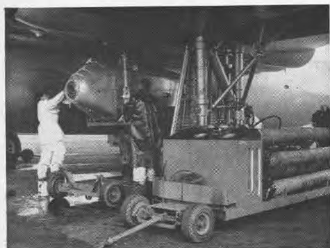
A VALIANT bomber is fitted with two de Havilland Super Sprite rocket engines. Engines are in canisters which permit jettisoning them.
