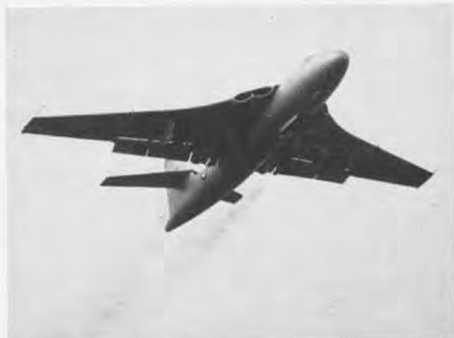
THE SUPER Sprite engine enables the Valiant to carry an additional load or take off from much shorter runways with a standard load.
