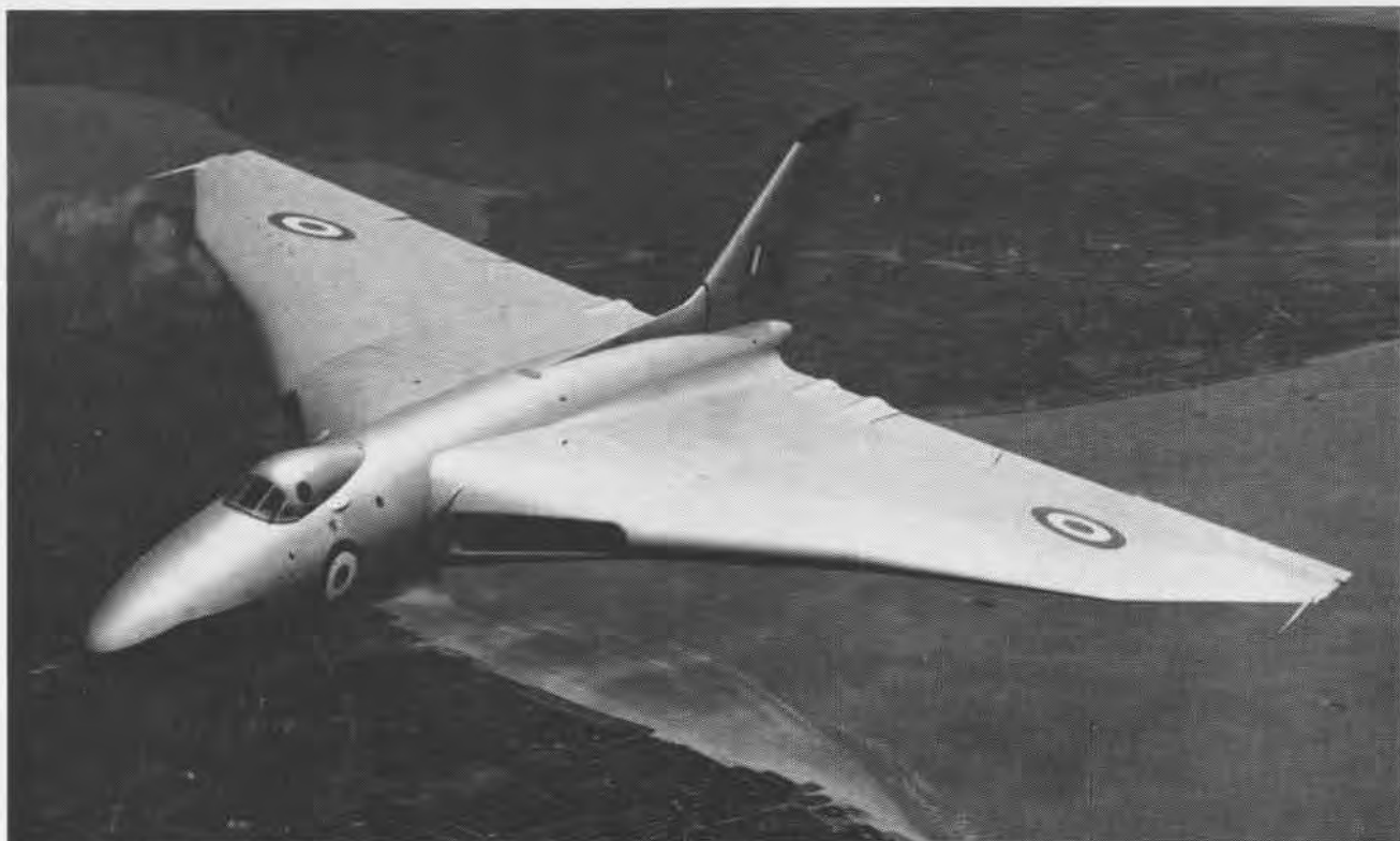
ON ITS FIRST flight overseas, this RAF Avro Vulcan, a delta-wing, four-jet bomber, landed at Melbourne, Australia, in September. The medium bomber is equipped with a new wing with a slight bend in the leading edge. It is scheduled for operational service very shortly.
