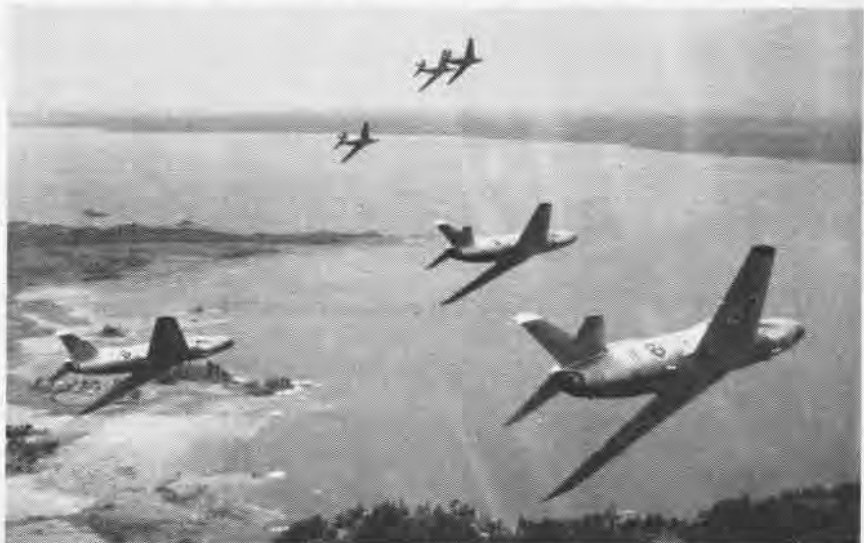
A FORMATION of Saab-32 Lansen transonic all-weather attack aircraft is flown by Royal Swedish Air Force pilots. The Lansen are coming off production lines on the double, and within a short time, the Lansen will become the mainstay of the SAF's attack force. Fitted with a Rolls-Royce Avon RA7 engine with afterburner, the Lansen is an over-700 mph. combat plane.
