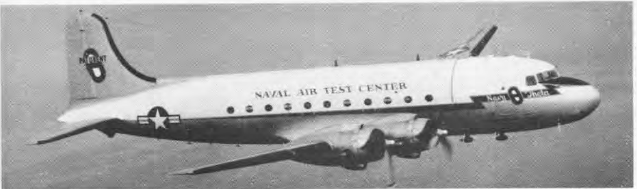
MUCH TEST DATA IS GAINED FROM THIS EXPERIMENTAL R5D, AN ELECTRONIC FLYING LABORATORY CAPABLE OF LONG RANGE FLIGHTS
