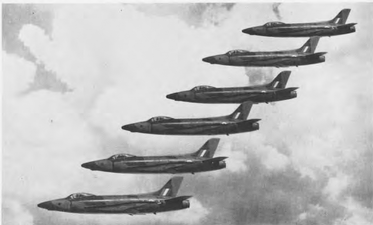
RAF NO. 2 SQUADRON flies the Supermarine Swift Mk. 5 aircraft in formation. This plane flew at Farnborough. It was originally designed as a jet interceptor, but its role has been changed to photographic reconnaissance and ground attack. It is equipped with an afterburner.
