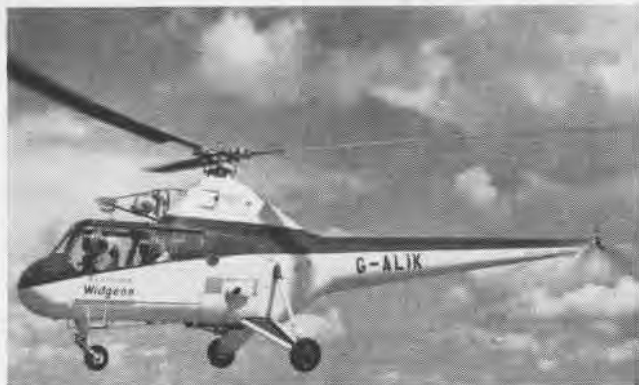
WESTLAND WIDGEON is an executive vehicle which carries a pilot and four passengers. It is a variant of a Sikorsky design built in Britain.
