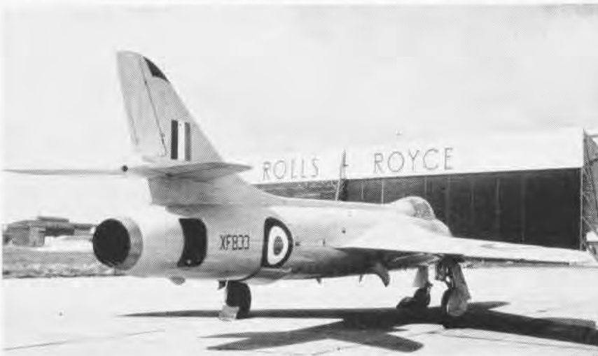
ROLLS-ROYCE IS USING A HAWKER HUNTER TO TEST-FLY ITS THRUST REVERSAL UNIT
