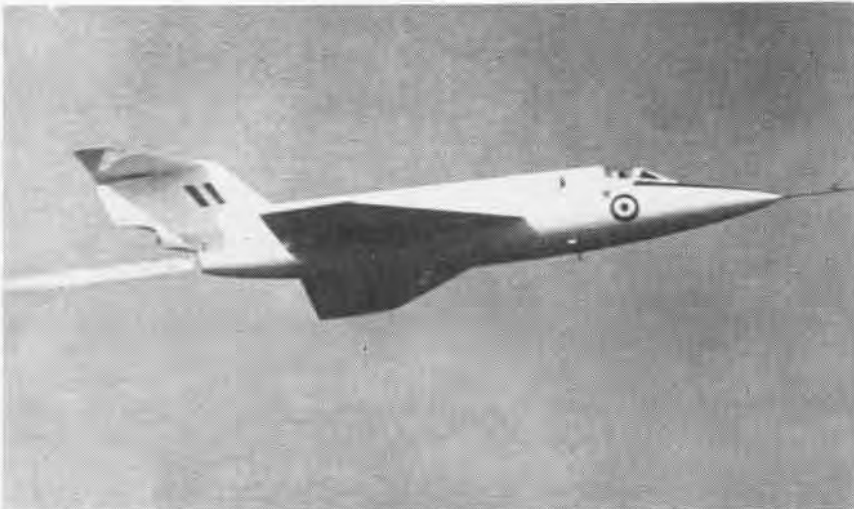
SAUNDERS-ROE 53 IS POWERED BY ONE SPECTRE ROCKET ENGINE AND ONE VIPER JET
