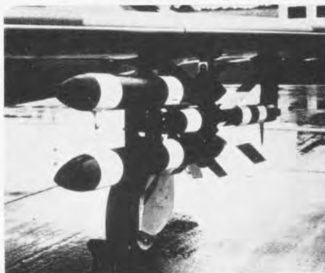
FIREFLASH guided missiles were displayed at Farnborough mounted on a Hawker Hunter F.4. Fly tests had been made in North Wales.
