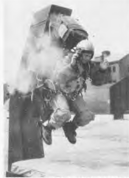
DEVICE WORKS \frac{3}{4} SEC. AFTER CLEARANCE
