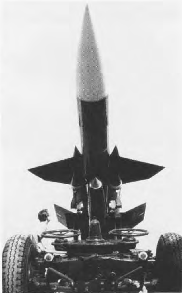
THE BLOODHOUND made its first appearance at Farnborough this year. This guided missile is powered by two Bristol Thor ramjet engines.
