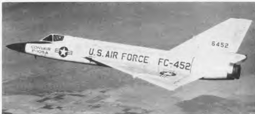
DELTA DART , Air Force F-106A interceptor, flies over the Mojave Desert in California. The supersonic, delta-wing, all-weather plane has been undergoing flight tests at Edwards AF Base. First production models are being flown for use in further tests. The Delta Dart, which is equipped with advanced fire control system and armament, is capable of stratospheric altitudes.
