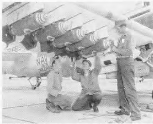
NEW ORLEANS MAR Reserve contingent loads practice bombs under wing of an AD Skyraider for use on close air support training mission.
