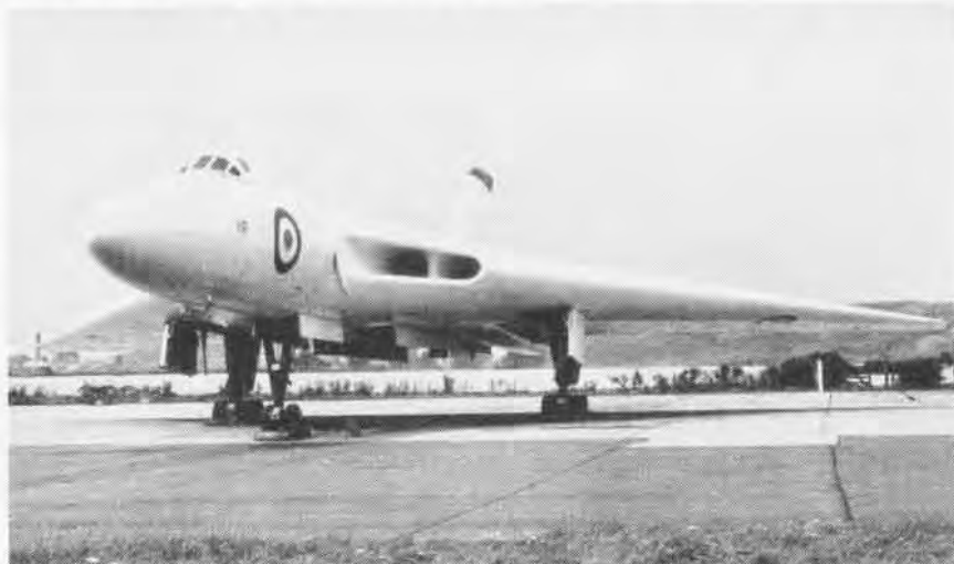
AVRO VULCAN IS BEING USED BY ROLLS-ROYCE TO TEST CONWAY BY-PASS TURBOJETS
