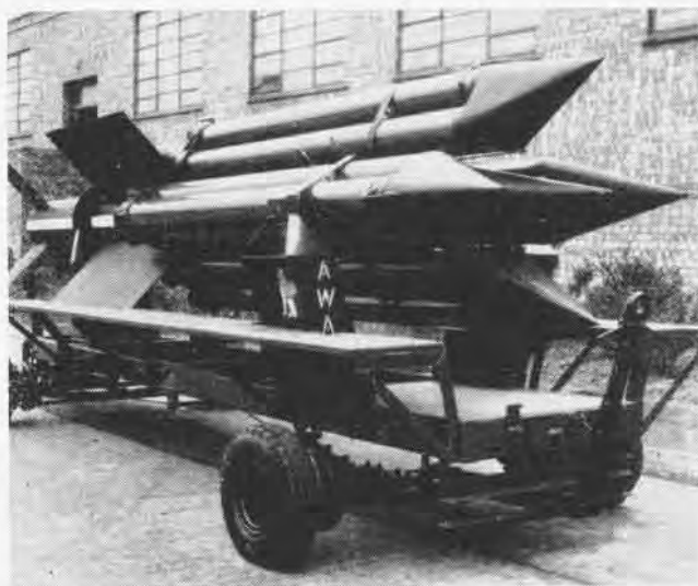
SEA SLUG , a naval AA weapon designed by Armstrong Whitworth, has four clusters of triple boosts which fall clear after burning out.
