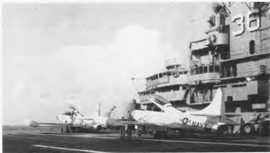
LINED UP on the flight deck of the big attack carrier, USS Antietam , these two T2V-1 SeaStar jet trainers shared topside billing during carrier suitability tests conducted recently off the Atlantic coast. The trainer underwent extensive fleet catapult takeoffs and arrested landing tests.
