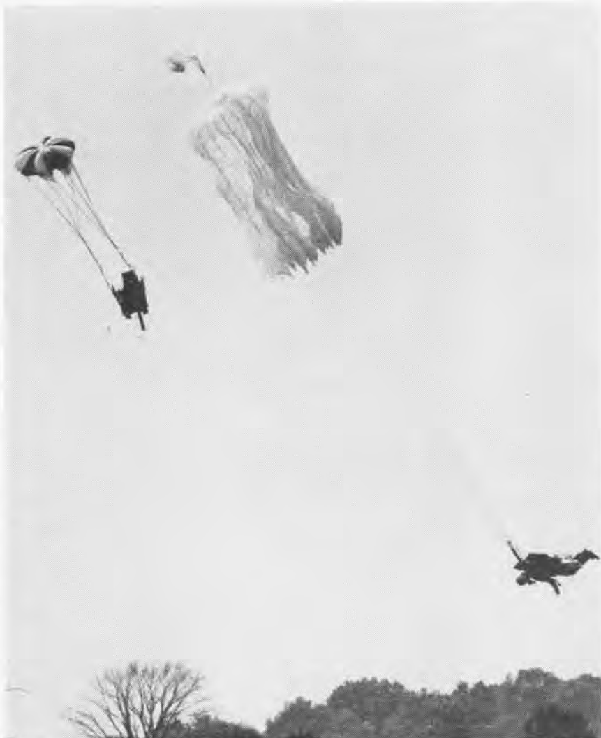
FROM ZERO ALTITUDE, ZERO SPEED, A T2J ROCKET CATAPULTS TEST DUMMY SAFELY
