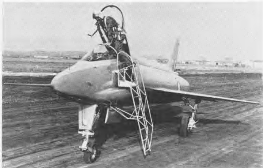
THE FRENCH BREGUET, the Br-1100, is a lightweight jet fighter equipped with two turbojet engines. A similar aircraft, but with one engine, the Br-1001, was designed for NATO. The Br-1100 was designed for the French Navy and Air Force. It has a take-off weight of 14,600 pounds, a maximum speed of Mach .92 and was designed to operate from 3000-foot grass strips.
