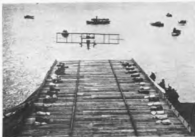
ELY BRINGS HIS Curtiss machine aboard USS Pennsylvania in January 1911. Lines and sandbags on the platform check the aircraft's run.
