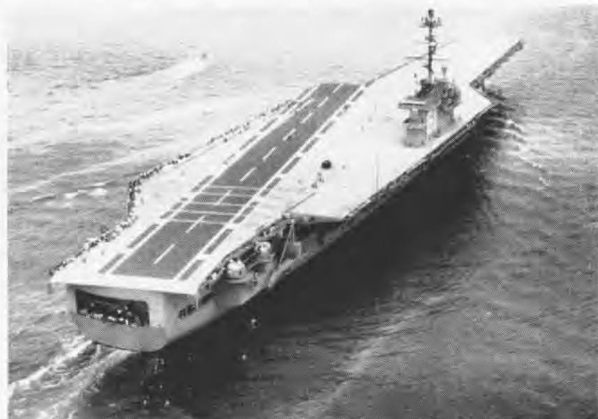
EIGHTH of a long line of ships to bear the illustrious name, the USS Ranger , CVA-61, is shown following commissioning ceremonies at the Norfolk Naval Shipyard. New flight deck marking pattern is dark grey with white lines and has been adopted as a result of human engineering studies. The 60,000 ton giant will be the first of the Forrestal class to join the Pacific Fleet.
