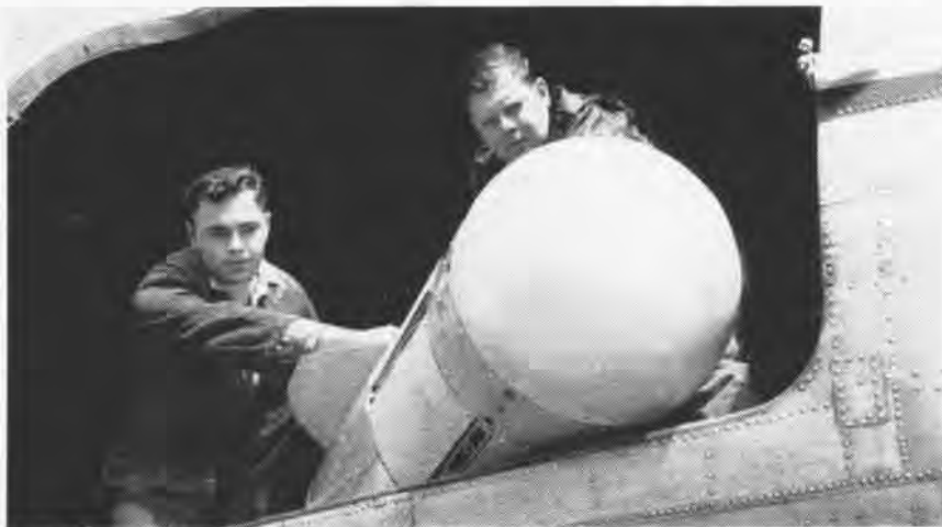
WHEN DROPPED FROM PLANE, GRASSHOPPER WILL TRANSMIT IMPORTANT WEATHER DATA
