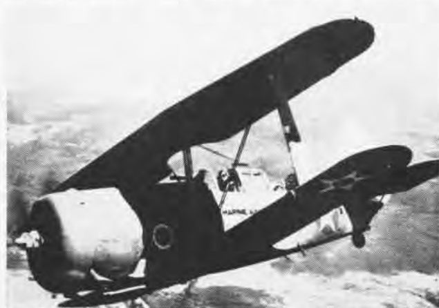
THE SBC, EARLY Helldiver , a two-seat scout bomber, was used by both the Navy and Marine Corps, aboard carriers and from land bases.
