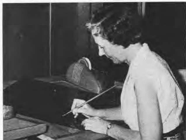
IN PRODUCTION , Miss Blanche Rodgers makes an opaque correction to a photo-offset negative before new technical manual goes to press.
