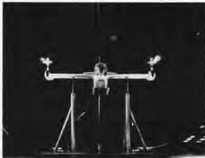
WIND TUNNEL tests on Bell Helicopter's XV-3 convertiplane have been successfully completed at NACA's Ames Laboratory. Developed for the Army, the XV-3 is a tilting rotor type with rotor propellers at each wing tip.
