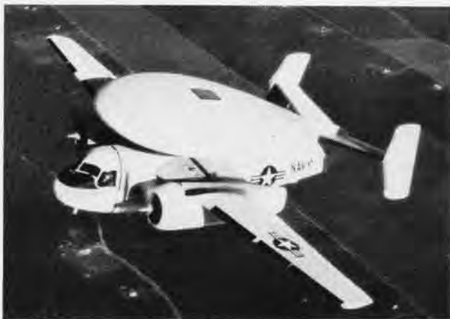
NEW EARLY WARNING carrier aircraft, the WF-2, features a large saucer-like radome which houses the long range radar antennae.
