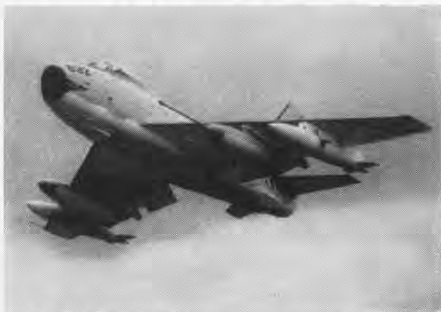
THE FJ-4B , a Fury modified to carry a variety of bombs externally, added offensive power when it joined the operating forces in June.
