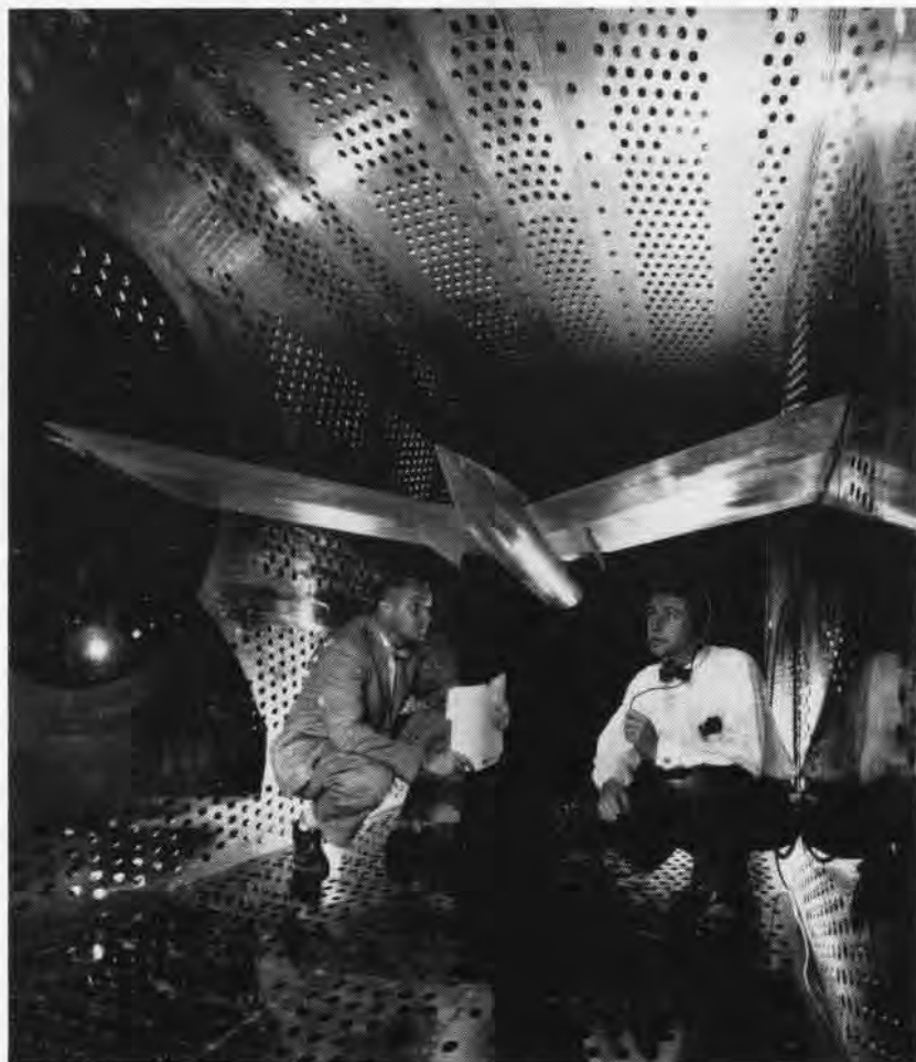
PERFORATIONS shown in tunnel serve to eliminate shock and pressure disturbances at transonic speeds. Either aerodynamic runs or burning engine tests can be conducted.
