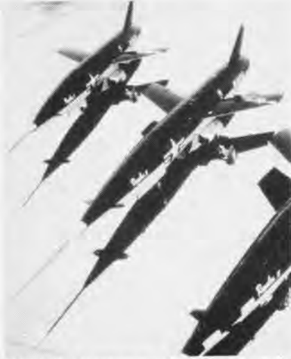
REGULUS II , supersonic long range missile, on tricycle landing gear used during tests.
