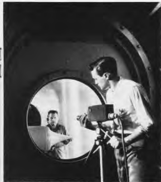
CLOSED-CIRCUIT television of engine model operation enables the research scientists to study ramjet tests.
