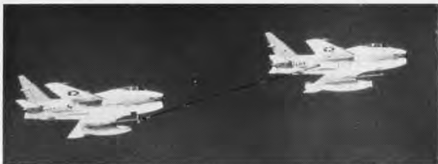
TO EXTEND the range of the F1-4B attack aircraft, the "buddy tanker" refueling system is being tested by the Columbus Division of North American Aviation, Inc. Two F1-4's are being used. After climbing to altitude, the received aircraft meets the buddy tanker at 25,000 to 40,000 feet. Engineering work being done will permit transfer of fuel from either external or internal tanks.
