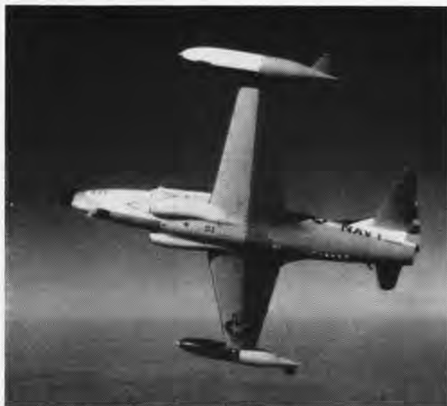
T2V SEASTAR , a two place single engine jet trainer designed for land and carrier operations, was assigned to the Training Command.
