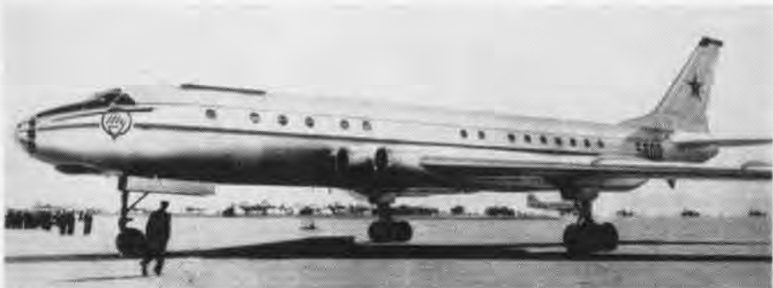
COOKER (TU-110) is a four turboprop aircraft, a development of Camel (TU-104). The major difference between the two Soviet planes is that the fuselage has been lengthened, and the Cooker has four engines instead of two. The transport can accommodate 78 passengers travelling first class, 100 travelling tourist. The aircraft has a 1850-nautical mile range at 440 knots.
