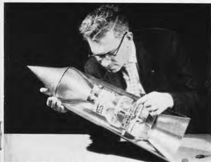
REDUCED COMPRESSION blade section, short primary burner and afterburner in futuristic turbojets are planned to take advantage of new fuels.
