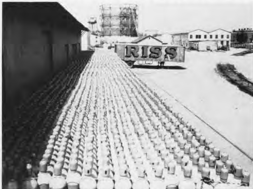
SOME OF THE 50,000 CYLINDERS USED TO SHIP HELIUM; STORAGE TANK IN BACKGROUND
