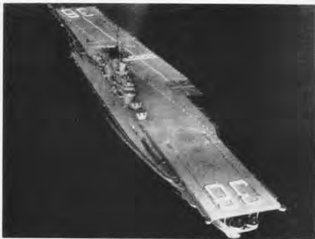
USS ANTIETAM first angled-deck carrier in the U. S. Navy and now the first angled deck to report for duty with the Air Training Command.
