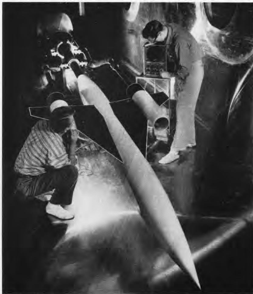
AT CLEVELAND, Ohio facility, wind tunnel testing of advanced design aircraft engines and their components is conducted at speeds of 1500-2500 mph by NACA scientists.
