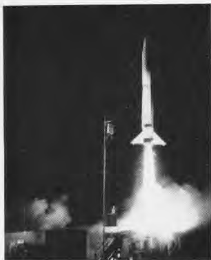
THE FIRST stage rocket Viking roars off in first test of the satellite launching vehicle.
