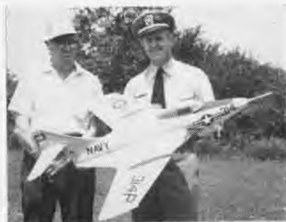
THIS COUGAR-ETTE is an exact scale model of the F9F-8. It took two years to build. A Dyna-Jet engine develops 4½ pounds thrust, over 100 knots. LCdr. W. H. Weimer, NAS Akron, admires Harold Beamer's handiwork.
