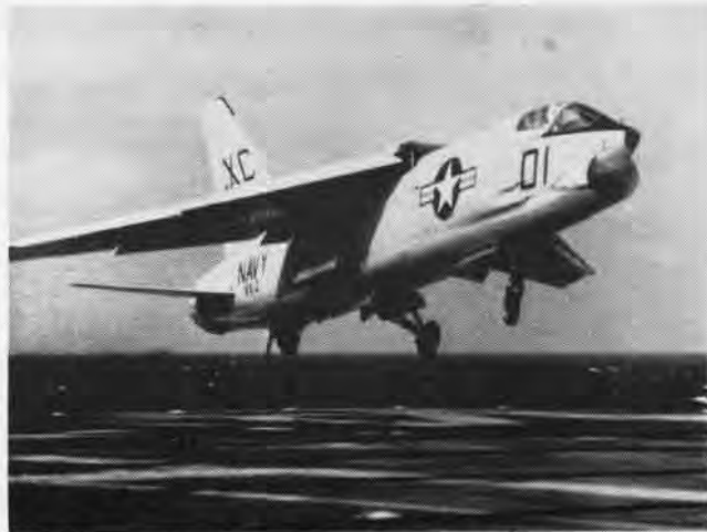
VARIABLE INCIDENCE WING PERMITS SLOWER LANDING, TAKE-OFF
