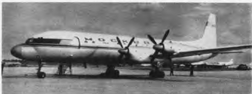
THE USSR'S COOT (IL-18) , a modification of Clam , is an aircraft designed by Ilyushin. It is powered by four turboprop engines which produce 4000 ESHP. This transport can carry 75 to 100 passengers, cruise 2700 nautical miles at 325 knots at an altitude of 26,000 to 33,000 feet. Coot has a low, straight wing, two passenger entrances on port side, and radar located in the nose.
