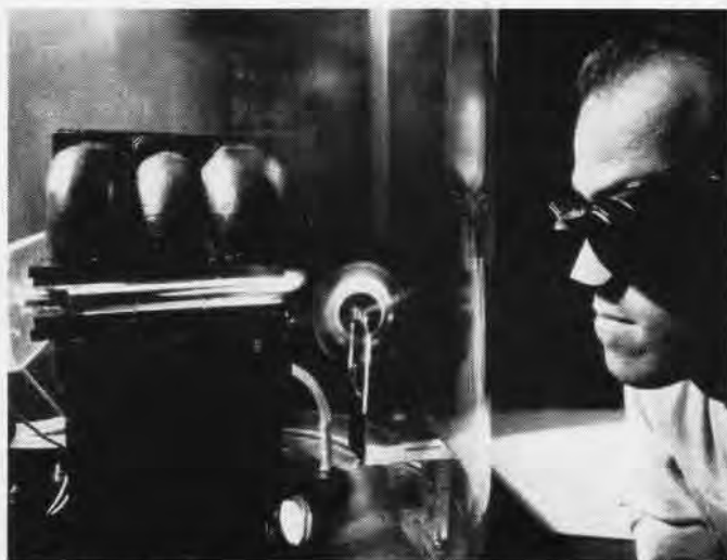
ION PROPULSION studied. Charged particles resulting from disassociation of matter are accelerated by magnets and demonstrated as thrust force.
