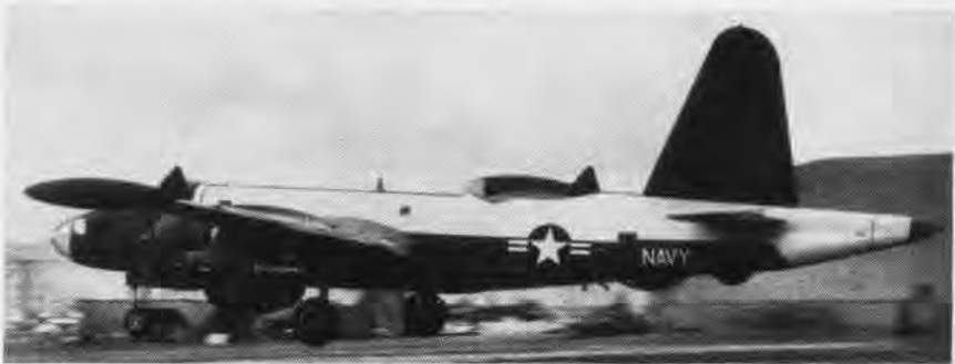
TWO-TONE PAINT job, white top with dark gray under-fuselage, wings and tail, replaces former dark blue exterior of P2V Neptunes coming off production line. New paint job, originated by Airborne Equipment Division in BuAer, gives more temperature comfort in plane.
