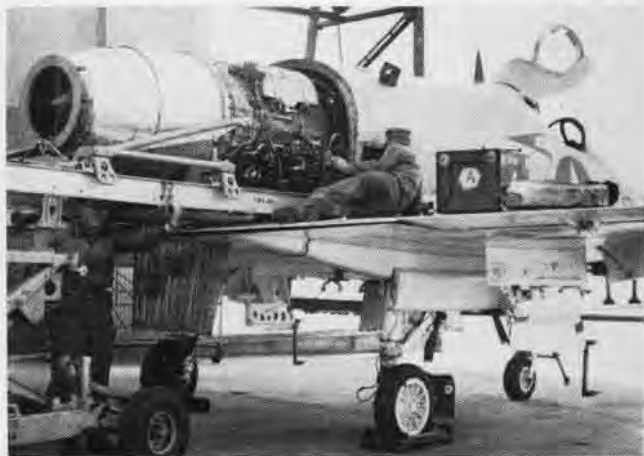
THE FINISHED PRODUCT of the jet shop is a newly renovated engine which is carefully rolled into the waiting Douglas A4D Skyhawk.
