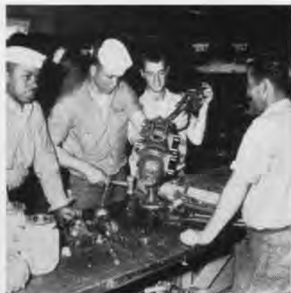
AERIAL TARGET POWERPLANT IS REPAIRED
