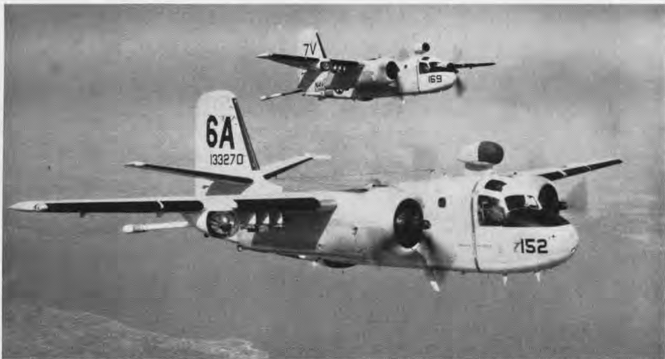
TRACKERS FROM NARTU ANACOSTIA AND NAS GLENVIEW, WITH MAD GEAR STINGER EXTENDED, ARE OFF ON A SUB-SEEKING PATROL
