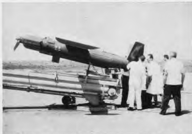
RECOVERY SYSTEM INSTALLATION BEFORE LAUNCH FROM AT-3 CAT
