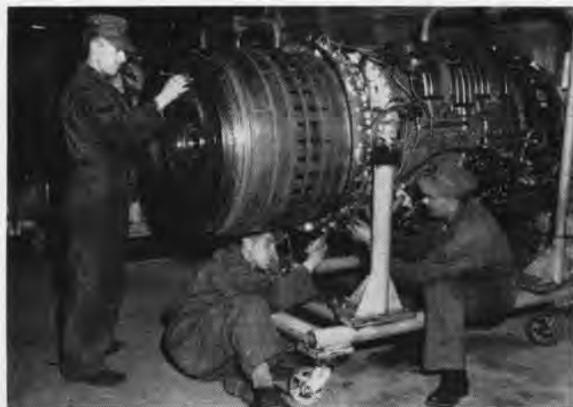
HIGHLY TRAINED personnel in four major jet engine types insure accurate service. Here finishing touches are put on a J65 engine.
