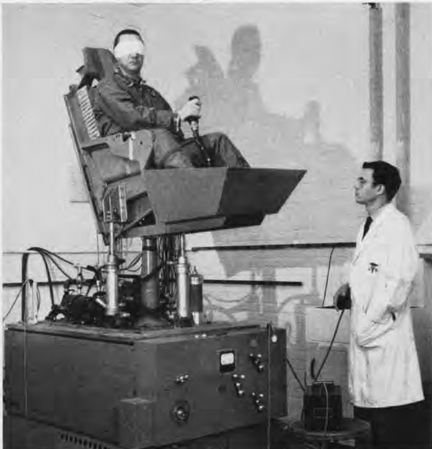
ONE METHOD of testing equilibrium for the seven Mercury Astronauts was to make candidates keep chair on even keel as it rotated on two axes at once. Capt. Grissom, USAF, is being tested.
