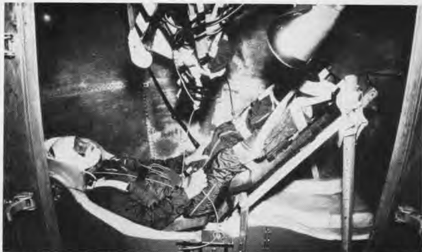
PROJECT MERCURY SPACE COUCH CENTRIFUGE TESTS CARRIED THE SUBJECT TO 25 G'S
