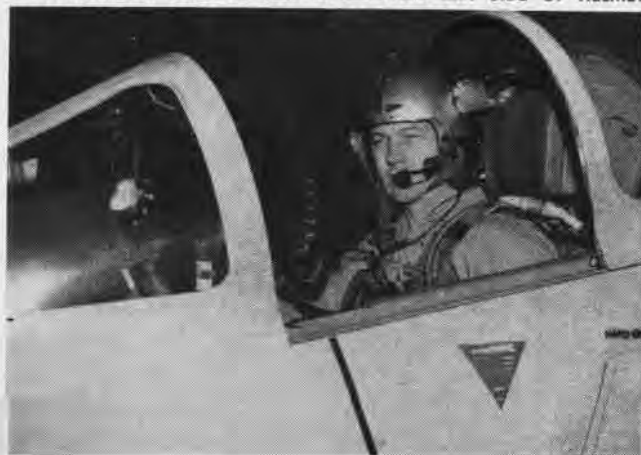
ACCELEROMETER USED IN TEST IS SEEN ON LEFT SIDE OF HELMET
