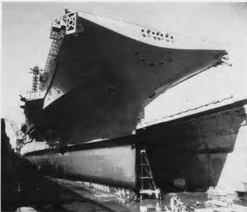
BIGGEST EVER! The USS Kearsarge (CVS-33), biggest ship ever to be put in the drydock at the U.S. Naval Shipyard, Long Beach, Calif., gets her hull cleaned. The 43,000-ton carrier is the yard's first complete carrier overhaul; the project is scheduled to take four months. The big ship, once an attack carrier and now an antisubmarine carrier, is homeported in Long Beach.
