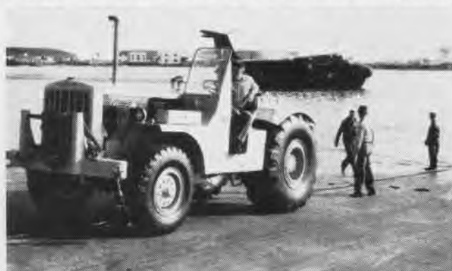
BEACH CREW USES TRACTOR, STEEL CABLE TO TOW P5M UP RAMP
