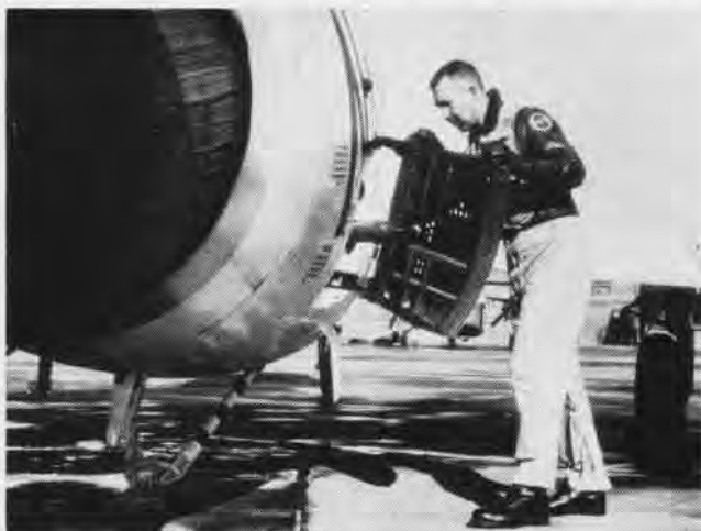
MSGT. TODD is the only enlisted pilot assigned to the Overhaul and Repair Department. He has a total of 395 test flight hours to his credit. He leaves nothing to chance as he makes his thorough pre-flight inspection. He carefully checks the speed brakes on the Demon.
