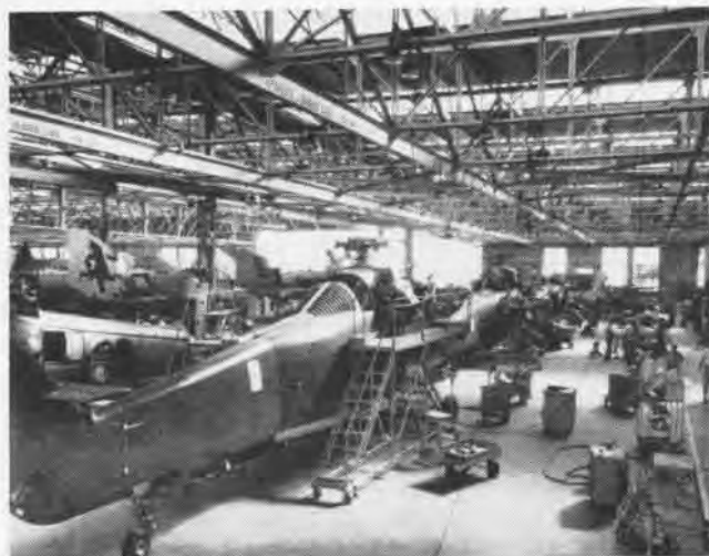
ROTARY-WINGED aircraft are relatively young in the aircraft family. Here a Sikorsky HSS-1 helicopter is undergoing its final assembly.
