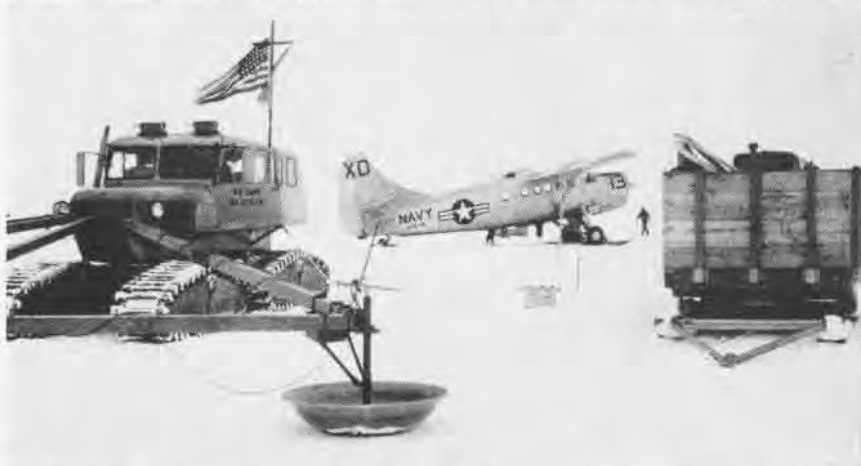
SKI-RIGGED UC-1 OTTER DELIVERS FUEL, FOOD, LAUNDRY TO TRAIL PARTY ON ICECAP
