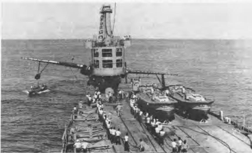
SAFETY LINES IN PLACE AND LINE HANDLERS READY TO MANEUVER PLANE ON BOARD
