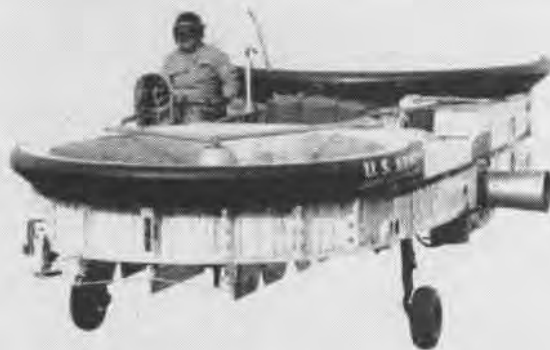
PIASECKI'S JET-POWERED aerial jeep flies at Philadelphia. The VZ-8P "Sky-Car" was developed and built for the U.S. Army. The wingless ground and air machine can ride along the highway, take off vertically and fly over road obstacles such as bombed-out bridges, traffic jams, unimproved terrain, all the time maintaining a close-to-the-ground altitude. Its compact design makes it safe for flying close to buildings and using rooftops for landings and take-offs.
