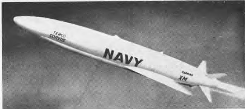
A TEST VERSION of the air-to-surface Corvus, a liquid propellant rocket-propelled missile, has been successfully flown at the Pacific Missile Range Test Center, Point Mugu. The test vehicle was fired from the A4D Skyhawk. Corvus was developed by the Temco Aircraft Corp., Dallas.
