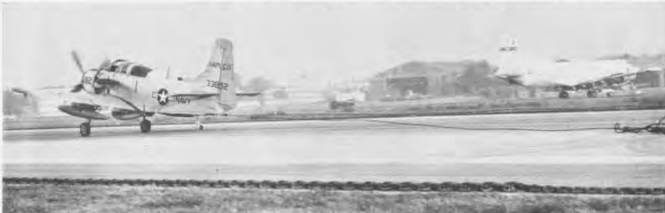
FIRST OFFICIAL ARRESTED LANDING at the U.S. Naval Air Facility, Naples, Italy, was made by LCdr. A.B. Blesener flying an AD-5. He initially engaged the wire while travelling at a speed of 87 knots, and the aircraft came to a smooth stop after 1200 feet. The completion
