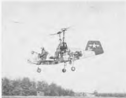
FIRST NAVY -evaluated Kaman helo's were K-223's. This one had Boeing gas turbine.
