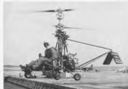
BUILT BY Gyrodyne, XRON-1's feature coaxial rotors, are designed for same use as XROE-1.
