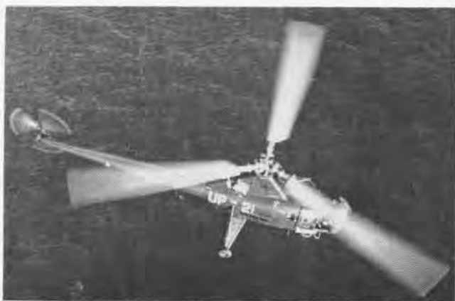
FIRST WIDELY used Navy model was Sikorsky HO3S-1, equivalent to the commercial S-51. With 450 hp P&W engine it weighed 5000 lbs.
