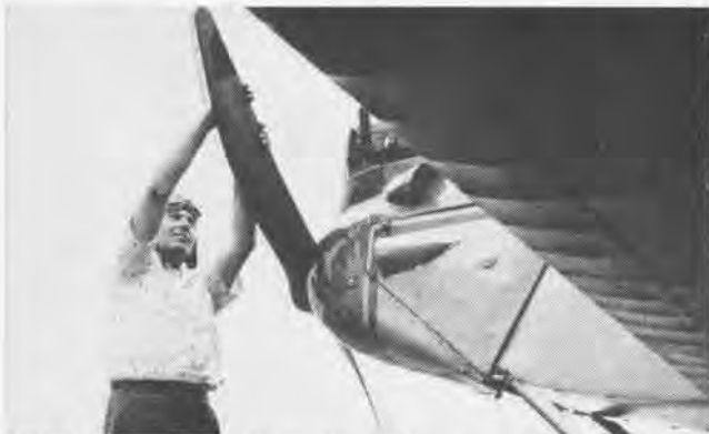
BERT B. BROOKS props his English-made engine installed in American-built de Havilland Gipsy Moth. Note unusual direction of prop-turn.
