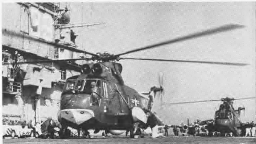
SIKORSKY TWIN T-58 powered HSS-2 is currently going into ASW service. Incorporating all-weather and latest ASW equipment, amphibious HSS-2 set helicopter speed record of 192.9 mph.
