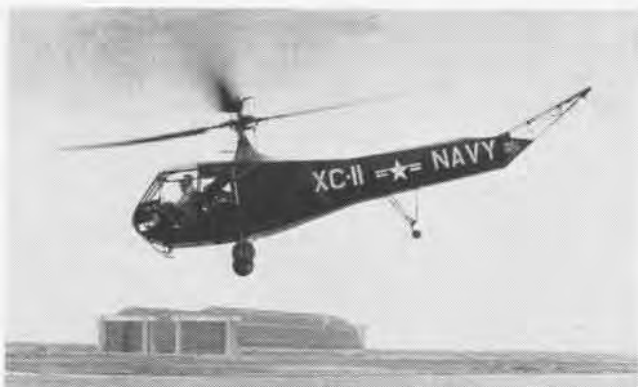
FIRST HELICOPTER design to reach operational status was Sikorsky's Army R-4; Navy/Coast Guard HNS-1, with 200 hp, weight 2550 lbs.
