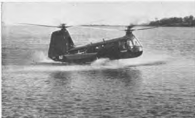
WHILE HELO'S have been capable of flotation using inflated bags since HNS's, Edo-modified HUP-2 Seacopter pioneered water-based design.
