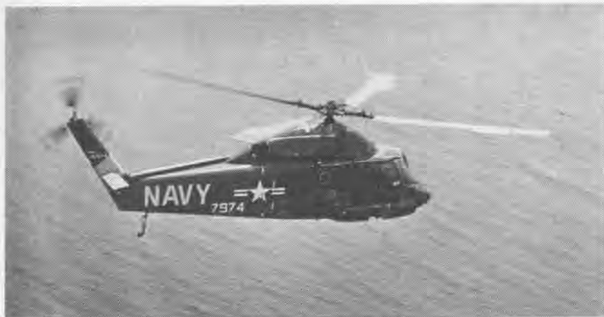
SOON TO ENTER Navy service is the Kaman HU2K-1 Sea Sprite. This new utility helicopter is powered by a single GE T-58 turbo-shaft engine, will replace piston engine utility models.
