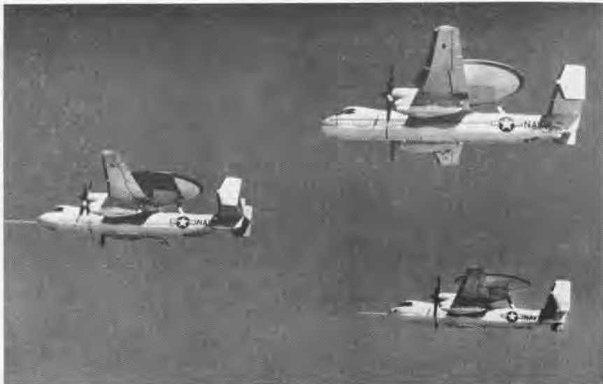
THREE GRUMMAN W2F-1 Hawkeyes fly together in the course of the flight development program of the Navy's newest airborne AEW/CIC weapons system. Many aircraft are used to allow simultaneous testing and development of airframe, power plant, avionics and equipment.
