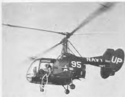
TYPICAL Kaman syncopter design was feature of HTK-1, procured in limited numbers.
