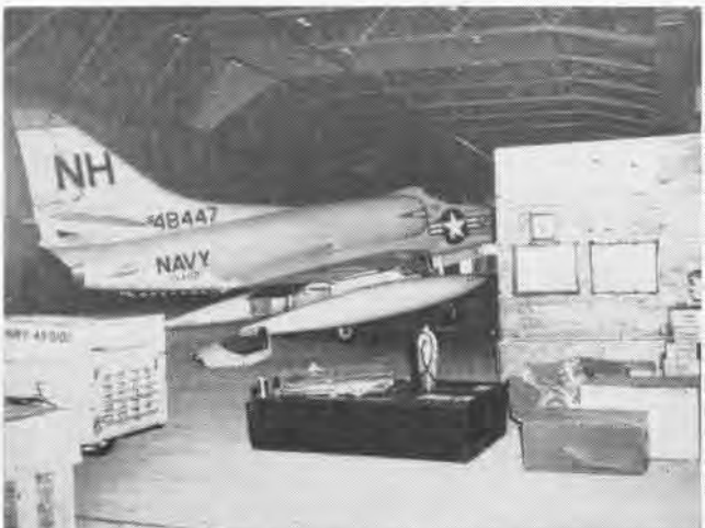
SQUADRONS moving into Lemoore found facilities of most modern design. Note lack of internal support posts in 800+ ft. long hangar.
