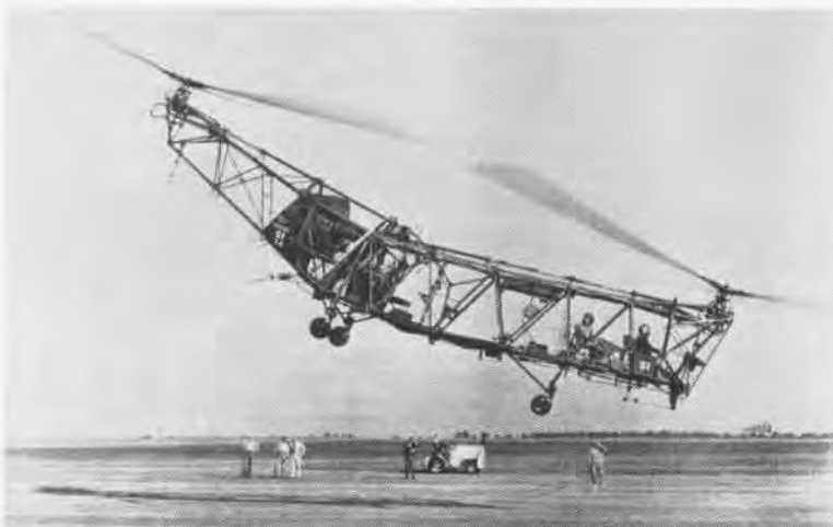
WEIGHT PLAGUED early helo operations. Piasecki HRP-1's flew with fabric covering removed for usable performance with added equipment. HRP-1 carries VX-1 markings.
