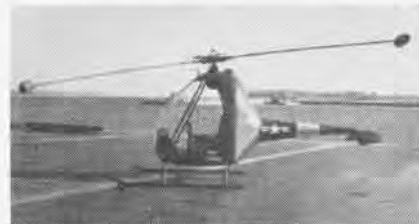
RAMJETS on both rotor tips powered this small two-place Hiller HOE-1 (Army YH-32).
