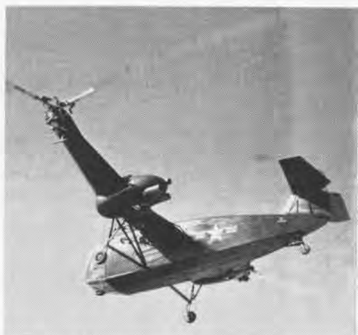
MCDONNELL'S first helicopter was twin-engine XHJD-1, like the XHRP it was a Navy sponsored WW II design.
