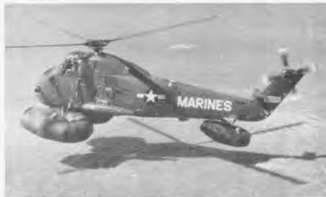
WITH SAME airframe as HSS-1, HUS-1 serves as utility-transport helicopter. HUS-1A shown has bags inflated to provide flotation
