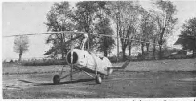
ORIGINAL NAVY Autogiros, Pitcairn XOP-1's, had wings. One was subsequently revised to a new wingless configuration as the XOP-2.
