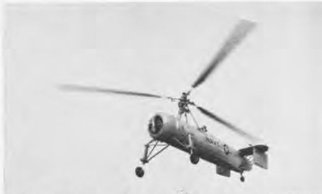
LITTLE KNOWN research and development project was Kollett KH17A, modified Autogiro, designed to test partially loaded rotor systems.
