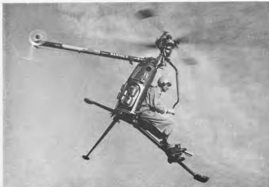
SIMPLE, ONE-MAN helicopter, requiring minimum pilot training for Marine field use, was goal of mid-Fifties program. Hiller XROE-1 was developed for service evaluation of concept.
