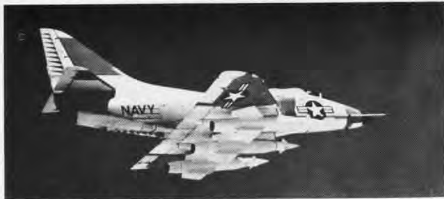
THREE BULLPUP B AIR-TO-SURFACE MISSILES ARE CARRIED IN A TEST FLIGHT ON A4D
