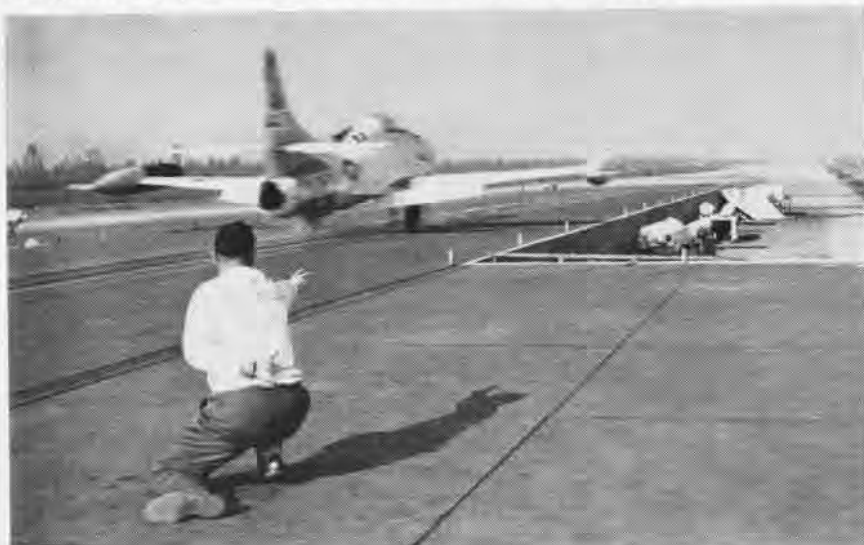
THE 10,000TH TEST shot on the TC-15 catapult was made 17 October at the Naval Air Test Facility (Ship Installations) at Lakehurst, N.J. The new steam catapult is now installed on the CVA-63, -64 and -65 and will be installed on the CVA-66. The test program of 2½ years corresponds to a five-year period of catapult operation under normal fleet use. The 10,000 test shots included more than 1000 live aircraft launches of such naval aircraft as the A3D, A4D, F4D and the F3H.
