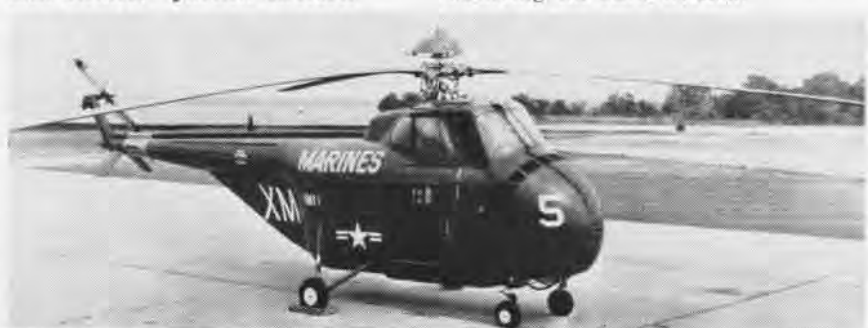
DOME-SHAPED ROCKET FUEL TANK IS MOUNTED ON THE ROTOR HUB OF HRS-2 HELICOPTER
