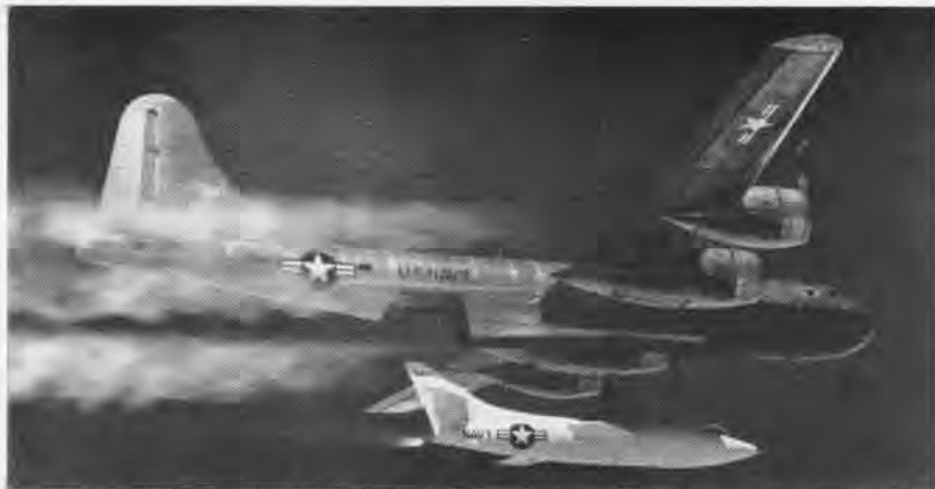
DOUGLAS D558-2 SKYROCKET IS BEING LAUNCHED FROM B-29 'MOTHER' PLANE
