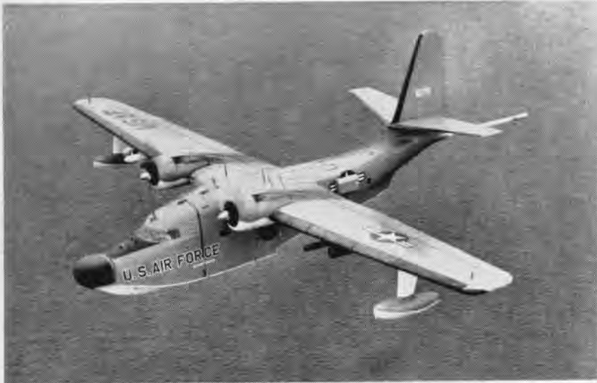
CONVERSION OF THE ALBATROSS into an anti-submarine patrol plane for use by one of the NATO countries is the result of a cooperative venture entered upon by Grumman, the Air Force and the Navy. Using Navy and Grumman ASW know-how, the Air Force sponsored Grumman's latest development of the versatile Albatross. Basically an SA-16B (UF-2), new bumps and protrusions mark the ASW additions. NATC is testing the NATO version.
