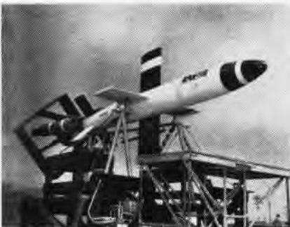
LARK MISSILE IS SHOWN WITH LAUNCHER
