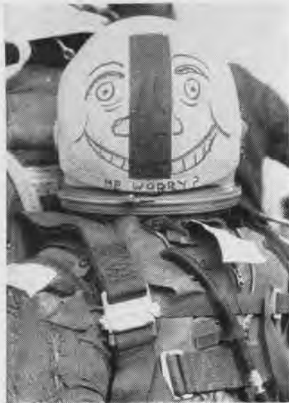
A DUMMY knows something—the value of a low-level ejection suit! When Ling-Temco-Vought conducted ejection seat tests using a couple of dummies, a wag with a grease pencil put a smile on and words "Me Worry?"
