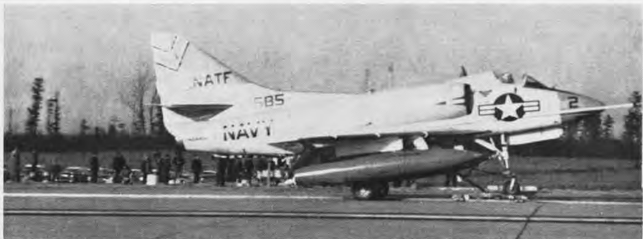
FIRST TAKE-OFF OF AN AIRPLANE BY AN XRE-1 CATAPULT WAS MADE AT LAKEHURST IN AN A4D JET PILOTED BY CDR. W.J. WELTY
