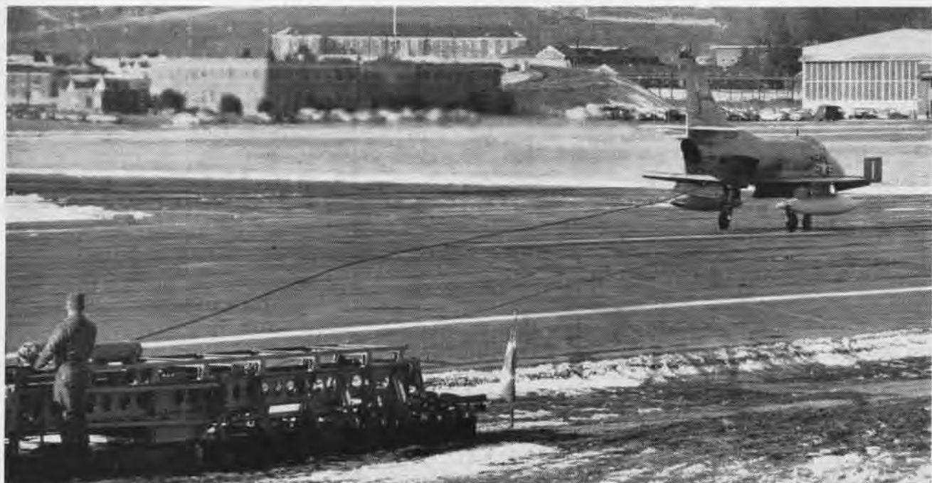
MOREST GEAR MAKES IT POSSIBLE FOR COL. BURNS, C. O. AT MCAS QUANTICO, TO LAND A4D SKYHAWK ON 4200-FOOT RUNWAY
