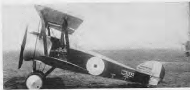
SILHOUETTE of Sopwith Camel shows machine gun installed on engine cowling. Synchronizer developed by Germans permitted this system.
