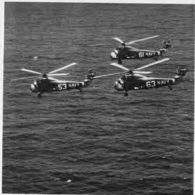
HS-8 FLIES SIKORSKY HSS-1N EQUIPPED WITH DIPPING SONAR
