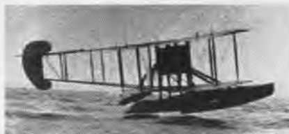
BATBOAT , developed by Sopwith in 1914, was inadequate. It was powered by 90-hp engine.
