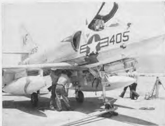
VA-56 PERSONNEL have been untiring in their efforts to keep the A4D Skyhawks available. Here two men check the wheel-well.
