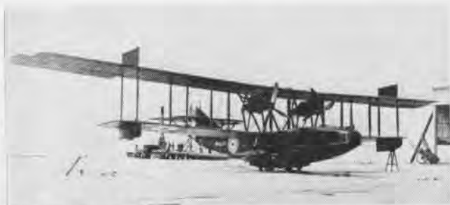
THE FELIXSTOWE F.5, called "Large America," was a British improvement of Curtiss' flying boat built before U.S. entered World War I.
