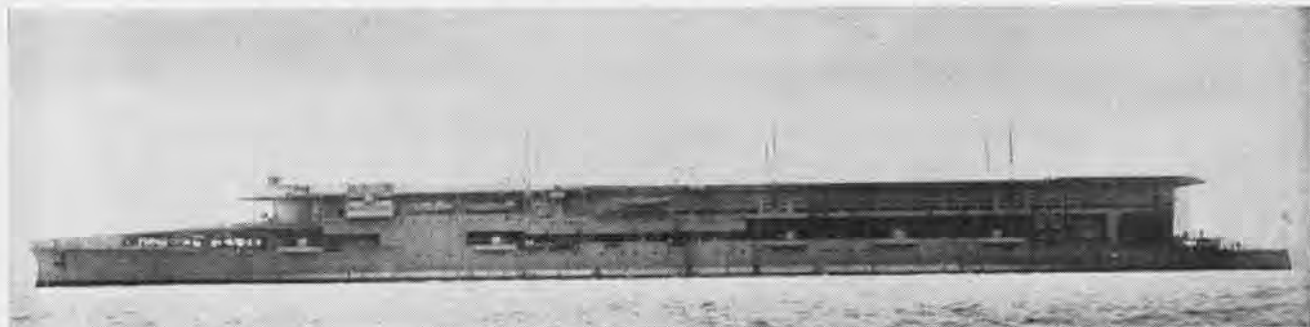
HMS FURIOUS was originally a light cruiser, refitted to operate aircraft, and recommissioned in July 1917. Flying deck was 228 feet long, 50 wide. Hangars beneath held seaplanes and landplanes. Later, she was provided a landing deck aft, fitted with arresting gear.
