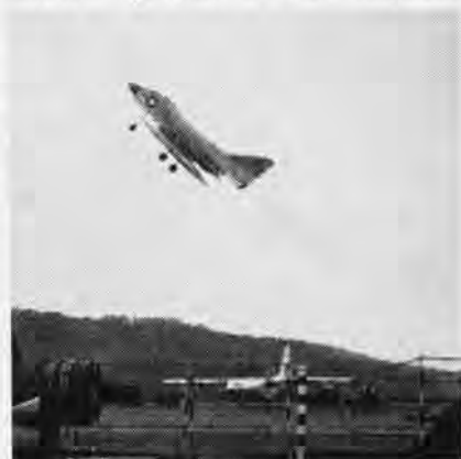
AN A-4 'ZOOMS' high after JATO launch from a short airfield. The maneuver was demonstrated at MCAS Quantico, Va., as part of air show staged for members of the First Marine Aviation Force Veterans Association.
