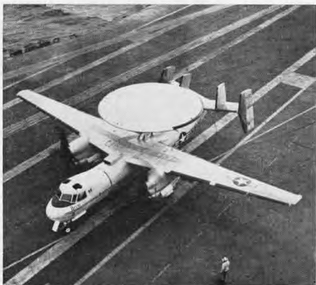
TWIN T-56'S MAKE HAWKEYE MOST POWERFUL CARRIER PROP PLANE
