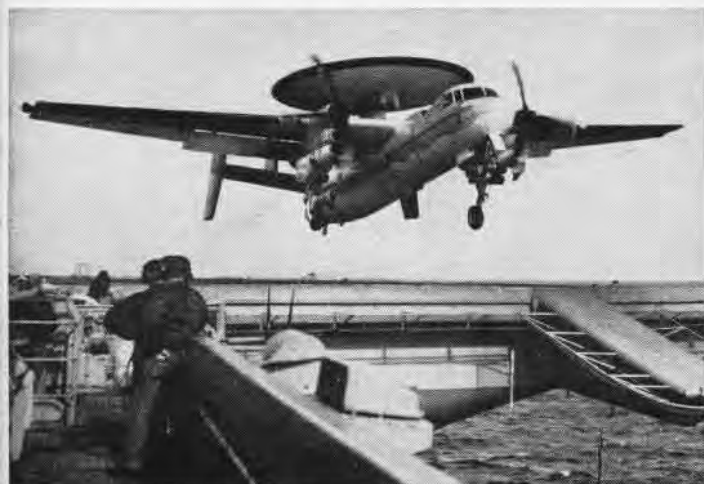
FLAPS AND DROOPED AILERONS DOWN, E-2A IS OFF AFTER TOUCH-AND-GO
