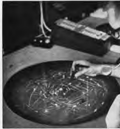
'SHRIMP BOATS' showing call and altitude of each flight, help controllers keep track.
