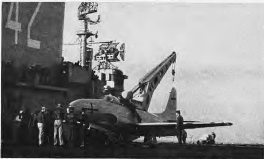
THE LOCKHEED P-80 Shooting Star , modified for catapulting and arrested landings, was tested for carrier suitability on board the USS Franklin D. Roosevelt (CVB-42) in November 1946.
