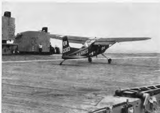
BOXER REVERSED normal operations in 40-knot winds. Marine O-1 took off as "wrong way" carrier steamed with wind off port quarter.
