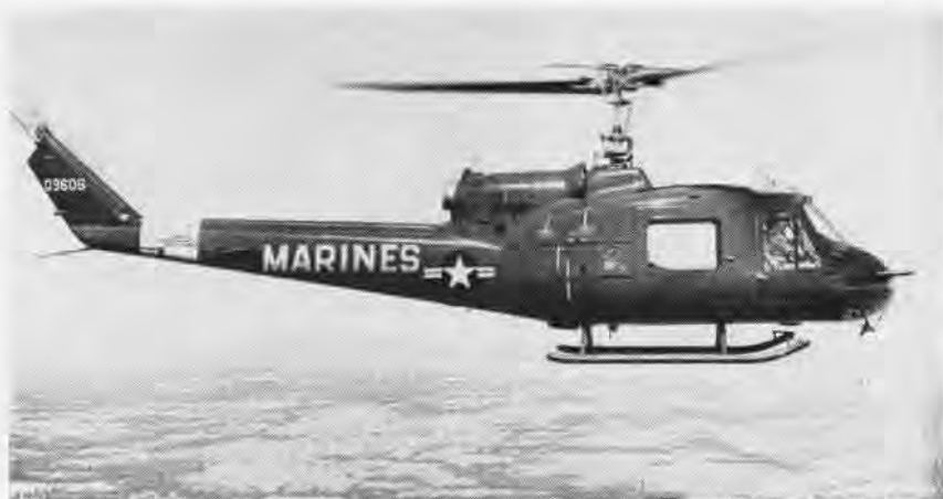
BELL UH-1E (HU-1E) helicopter is scheduled to replace the OH-43D (HOK) and O-1B (OE-1) aircraft now operated in Marine Observation Squadrons. Army version is operated in S. Vietnam.
