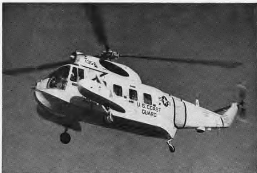
THIS IS ONE of 28 Sikorsky HH-52A helicopters being delivered to USCG air stations ringing continental USA. The Coast Guard selected the single-turbine, boat-bulled HH-52A last year after lengthy evaluation. It carries the latest in electronics gear, including automatic stabilization equipment. In evaluation tests, this helo model flew 230 miles on a simulated rescue mission, picked up six survivors and returned without refueling. It has a GE T-58-8 gas turbine engine.
