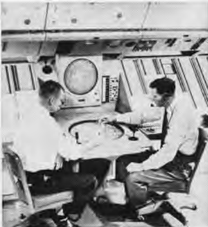
BRIGHT DISPLAY system gives controllers TV type display of area and air traffic.
