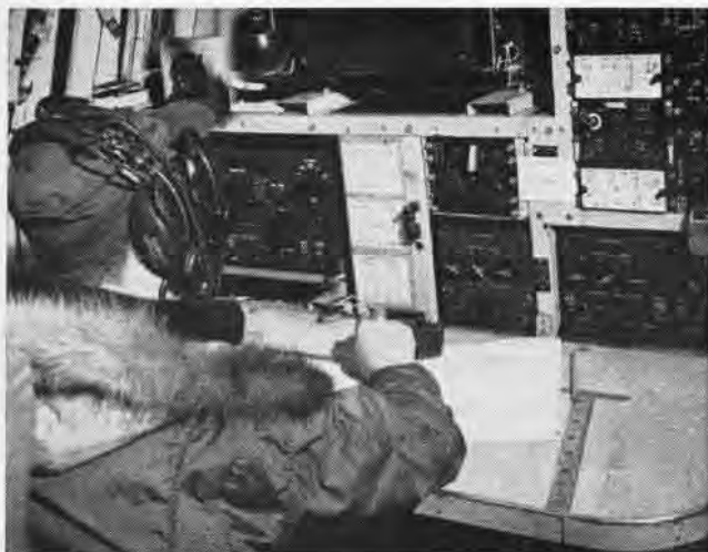
CW RADIO —dots and dashes—are normal communication link between planes on Barrier and OpCon Center at ComBarForLant Headquarters.
