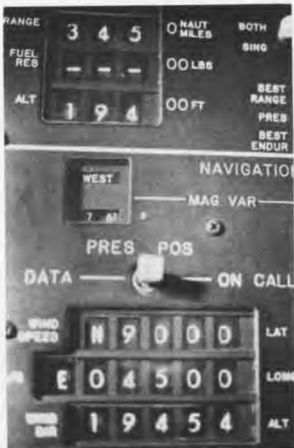
THIS IS Intruder's navigation panel read-out on flight of attack plane over the North Pole.
