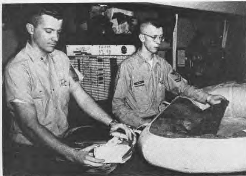
AVIATION SURVIVAL equipment is checked by D. B. Johnson, PR2, and Sellers during periodic 90-day inspection of one-man survival liferafts and associated gear installed in CVA-31 aircraft.
