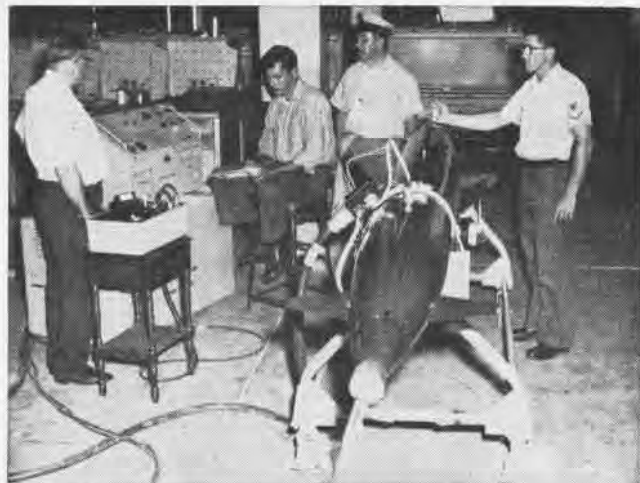
THE MISSILE CREW at NS Roosevelt Roads runs through 41-step check-out on a console to determine readiness of target missile—AQM-37A.
