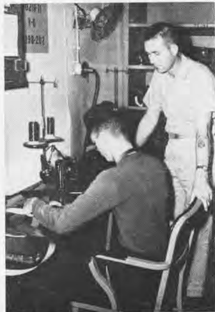
MEADOWS watches L. E. Walker, PR2, reinforce stitching in the harness of a parachute.
