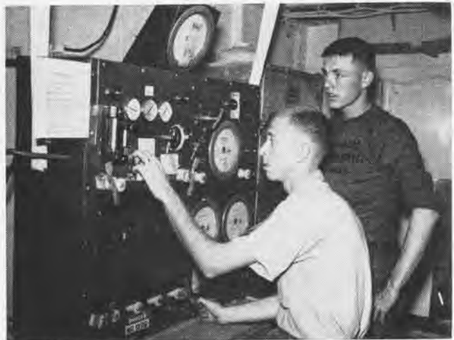
THE OXYGEN REGULATOR test stand in the carrier's paraloft is demonstrated by Sellers for the benefit of apprentice G. A. Varnadore.
