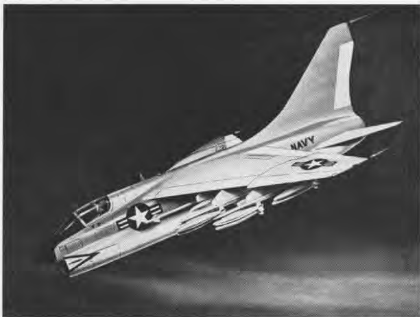
THE NEW VAL , substantially a version of the Crusader with a new engine, was designed by Ling-Temco-Vought (NANews, March 1963, p. 3). The light attack aircraft, to be designated A-7A, will be used by the Navy and Marine Corps. Its greater payload and range capabilities will enable it to have a longer time on station in close support of troops. Slightly larger than the A-4E, VAL will be easy to maintain with ready accessibility to all equipment for servicing.
