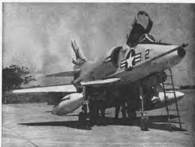
THE FINISHING TOUCHES are put on the new missile target as the Skyhawk is readied for the takeoff and launch of the target missile.
