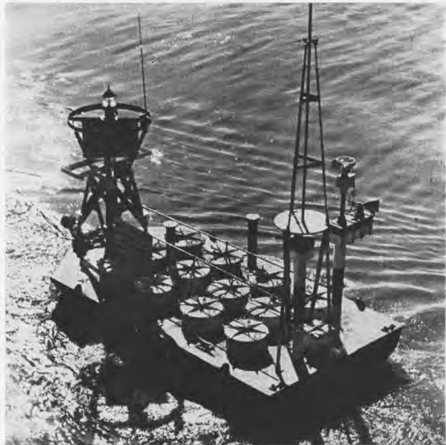
THE NAVY'S NOMAD weather boat is now on duty in the middle of the Gulf of Mexico, radioing temperature, barometric pressure, wind speed and direction, and sea temperature with instruments powered by a small atomic generator. The NOMAD is forerunner of a world-wide system of remote, unattended weather stations. The 60-watt nuclear generator is SNAP-7D. Earlier stations were powered by batteries that must be recharged every six months. SNAP-7D is designed to produce electric power continuously for ten years without having to be recharged.
