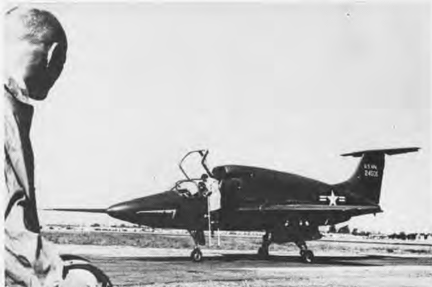
FIRST PHOTO of Army's XV-5A lift-fan jet vertical takeoff and landing (V/STOL) aircraft shows it rolling out of the Ryan Aeronautical plant at San Diego, preparatory to shipment to Edwards AFB for flight test. It was built for the Army Transportation Research Command. General Electric developed the lift-fan propulsion system. The two-seat subsonic jet is said to be capable of flying from fields no larger than a tennis court and can "live" with the ground forces.
